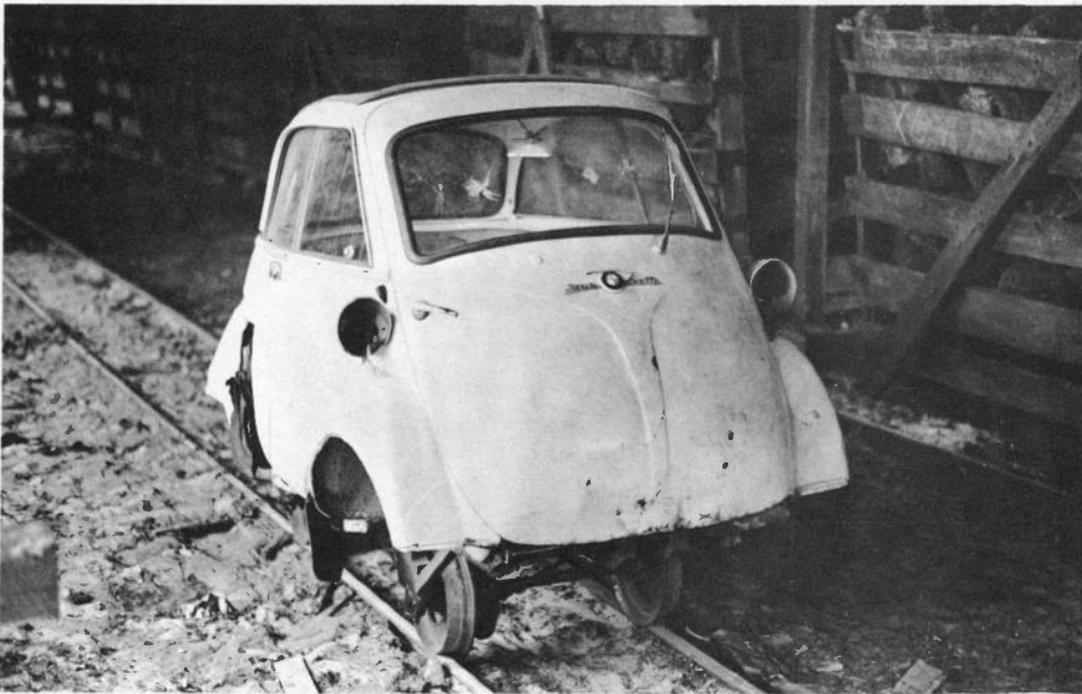
The modern scene. Brian Rumary and the Editor found this Isetta bubble car modified to run on 600mm. gauge tracks when they visited Lohne-Ost peat works, West Germany, on 6th. September, 1975.
