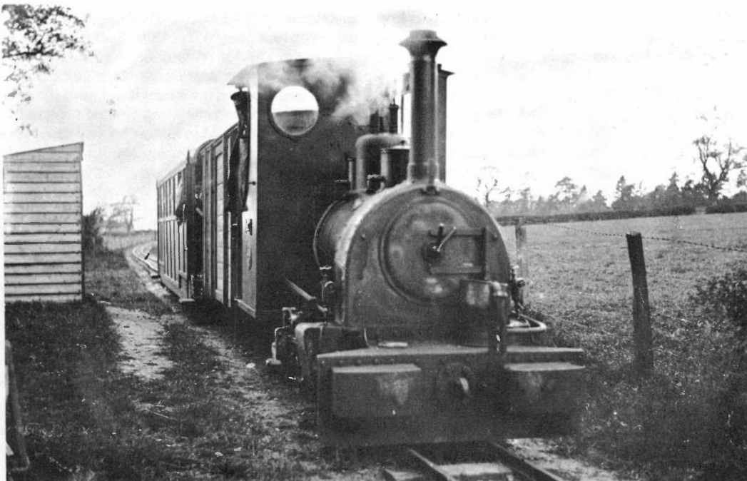
ESME on a passenger train from Warthill at Bossall station. A copper chimney cap has been fitted to the original stovepipe chimney. (Real Photographs Co. Ltd)
