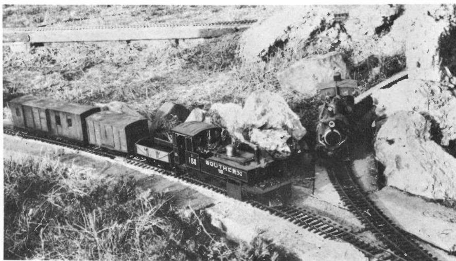
LEW with Tralee & Dingle and Isle of Man stock, passing the D.H.R. loco. The latter is a styrene body on a Lima 4F chassis with the centre wheels removed (D. Rowlands)
