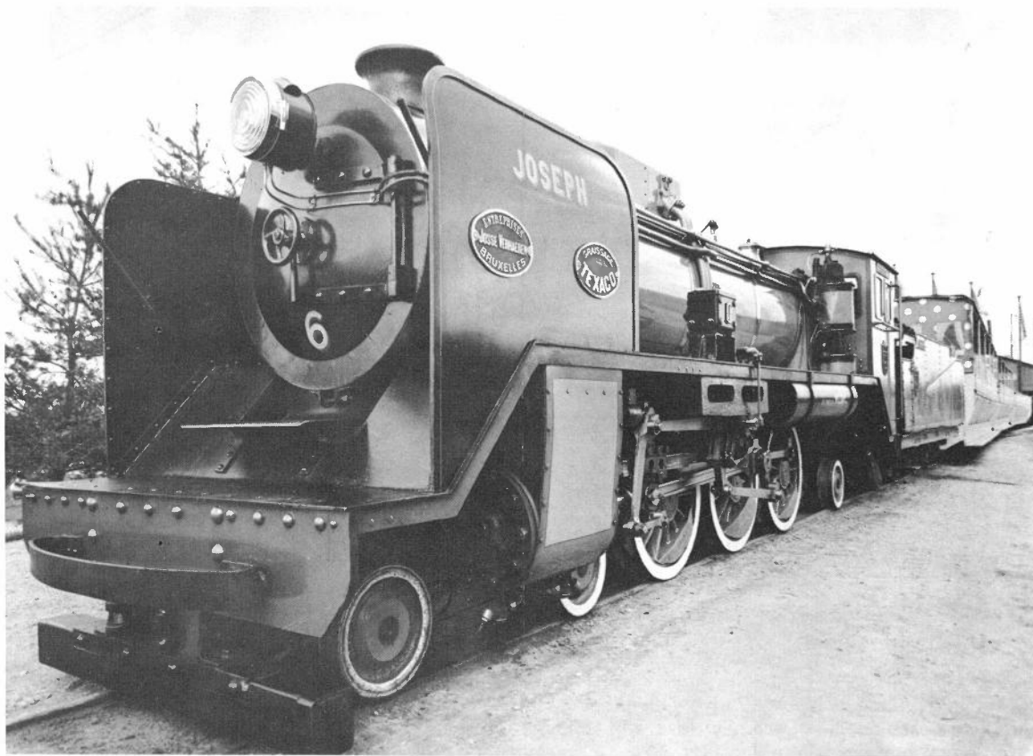
An impressive view of JOSEPH and train at Brussels. A large Westinghouse air pump is fitted in front of the cab. The train consists of two covered and two open coaches. (collection R.C. Riley)
