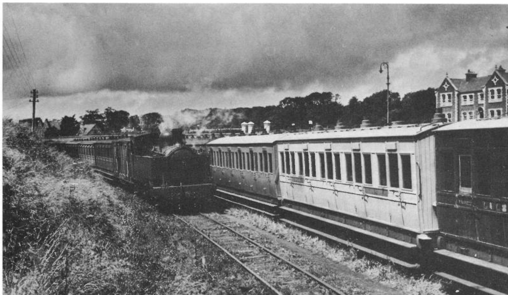
The timelessness of the Lough Swilly Railway is well portrayed in these scenes of the approach to Pennyburn yard. On the 7th July 1937 Hawthorn Leslie 4-6-2T 14 arrives in early afternoon with the 8.30 a.m. passenger train from Burtonport, 74 miles away on the west coast. The light grey carriage on the right (18) is a six-wheeler dating from 1885. Note the vents and pipes to the acetylene lights. (E.W. Hannan)
