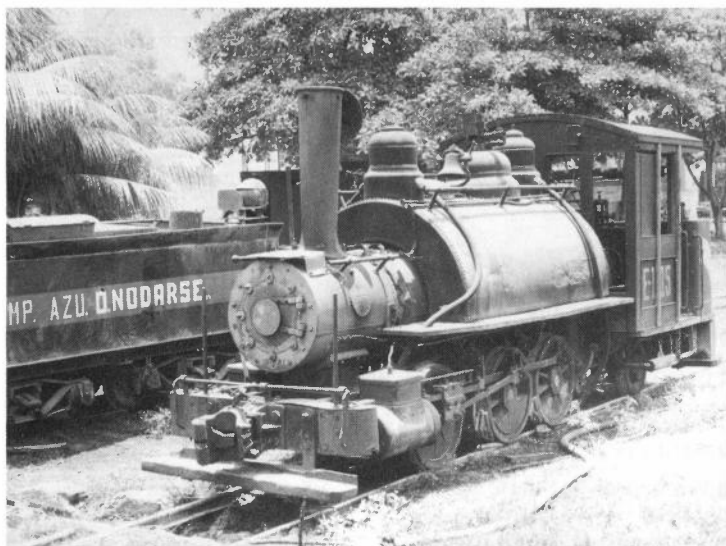
E-1115, a typical sugar mill 0-6-2T by Baldwin (56639/1923) basks in the sun.
