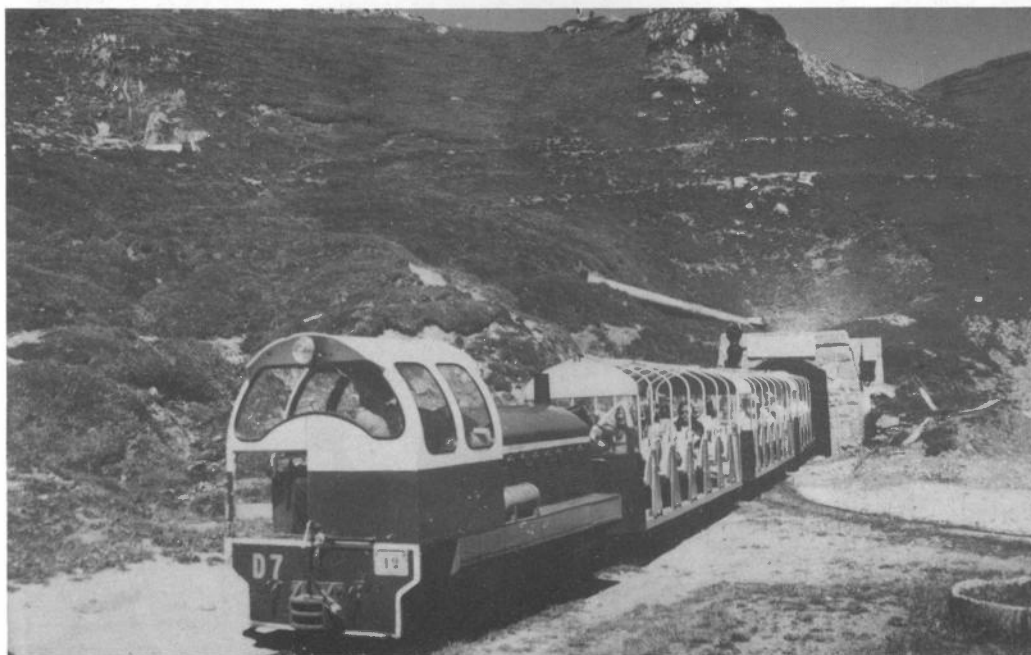
Billard D7 leaving the tunnel. Note the restricted loading gauge and colour-light signal on the left. (P. Delazzari)
