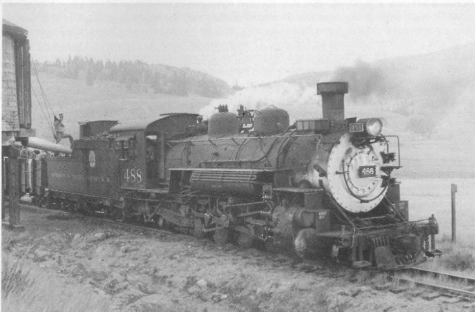
Ex. D. & R.G.W. R.R. 2-8-2 Class K.36 No. 488, having exchanged trains at Osier with 484 above, stops for water at Los Pinos tank. A third K.36, in steam at Chama would be the spare loco for the day, 27.9.80. These locos were Baldwin built in 1925. (Joseph P. Hereford Jr.)
