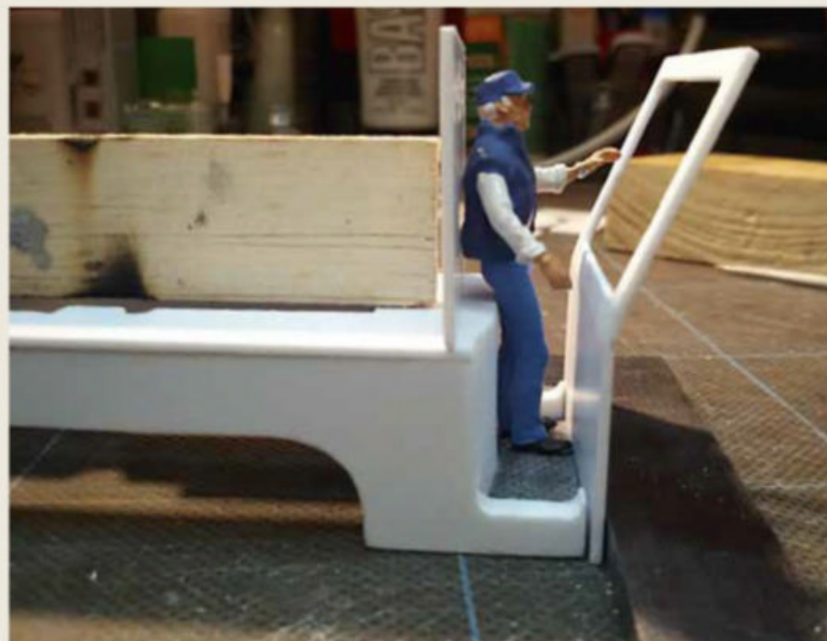
5 At the front, a pared down cab. Its outline was determined by the position of the driver: simple and pragmatic!
