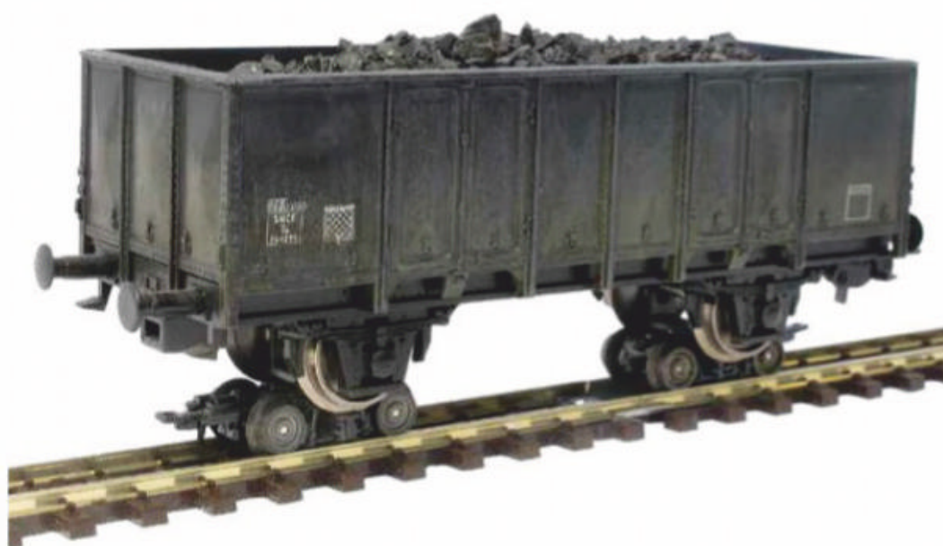
An open wagon carried on two Bemo Rollbocks.
