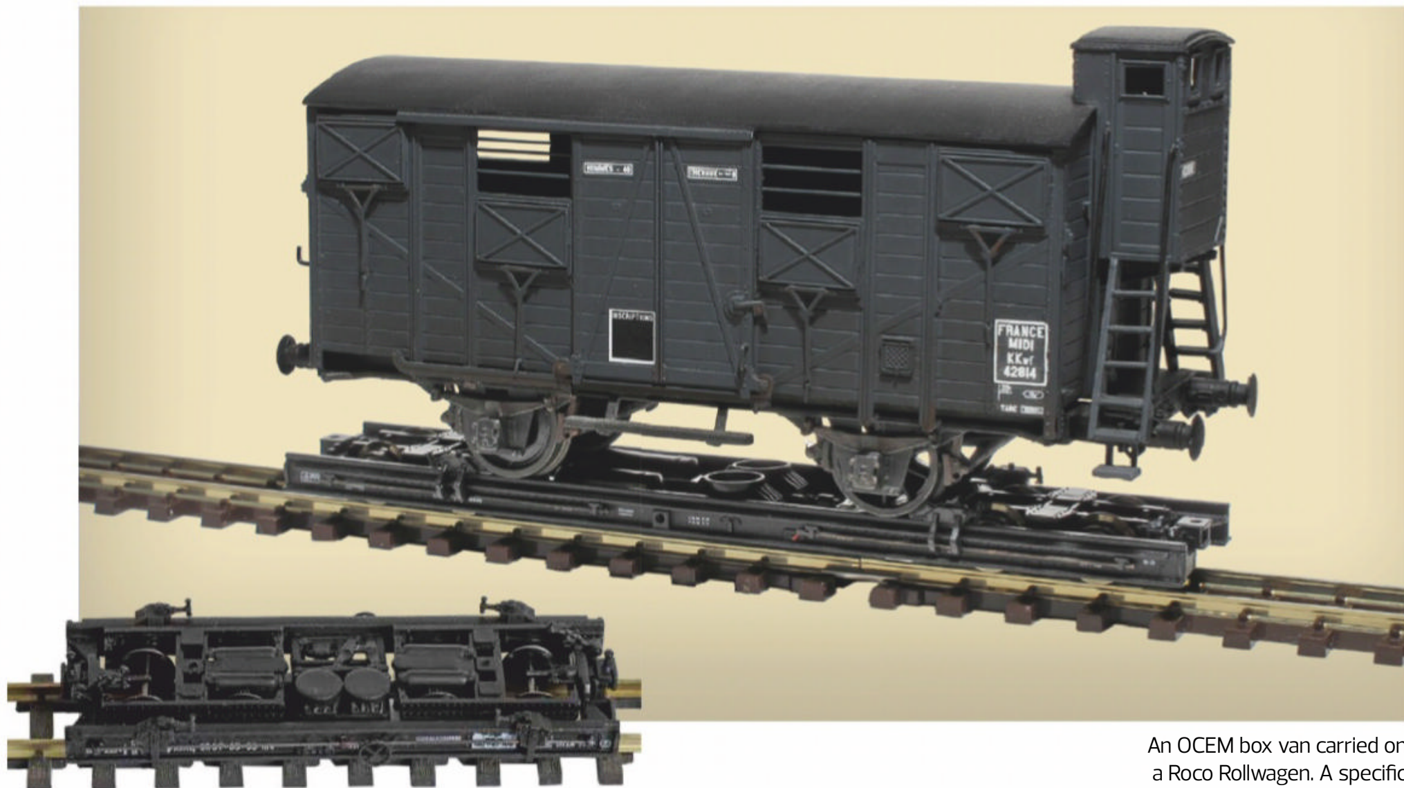
The MVT Rollwagen. The complete braking system is reproduced between the bogies.
