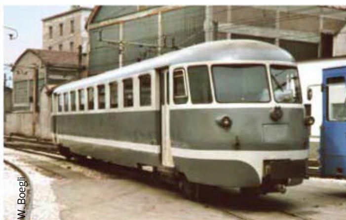
Diesel railcar (ex-Ferrovia-Mantova-Peschiera), converted into a pilot-car in 1977, at Trento-North in May 1975 .
