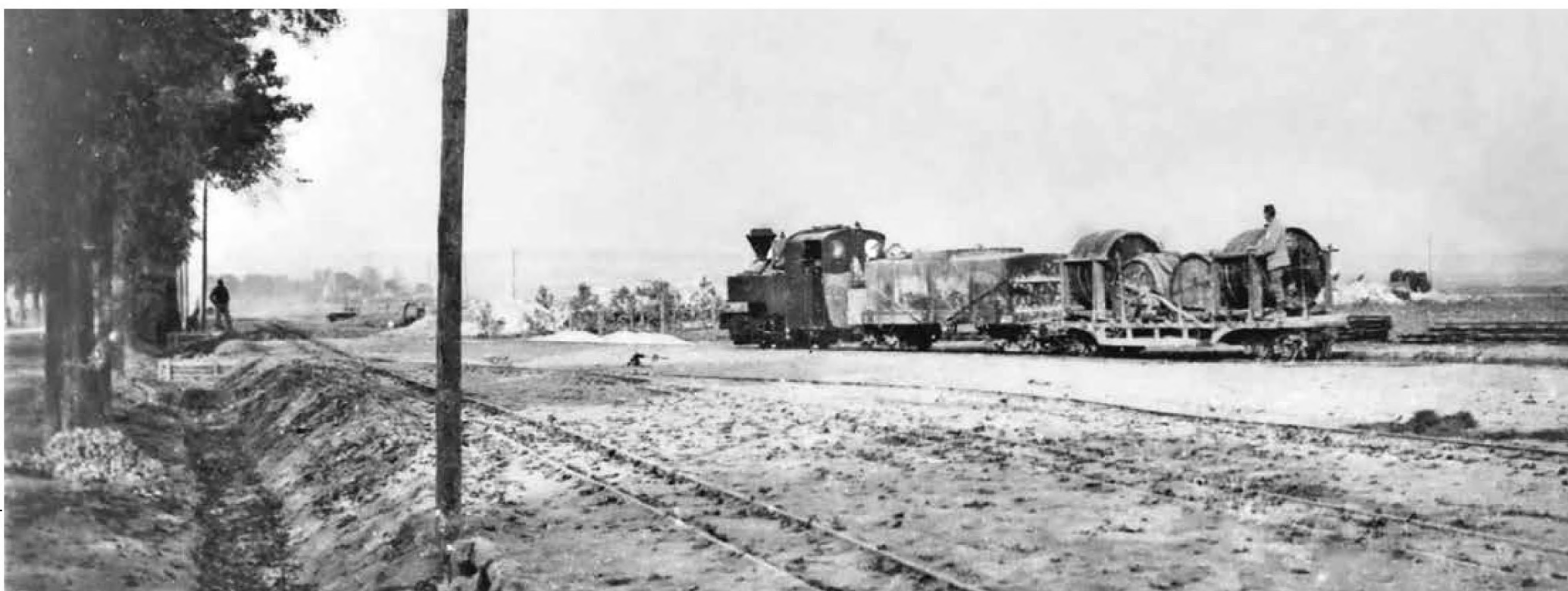
Another critical function of 60cm gauge was carrying drinking water. This Kerr-Stuart 0-6-0 tank engine is hauling a 1915 Decauville tank wagon and a Péchat platform loaded with barrels.
