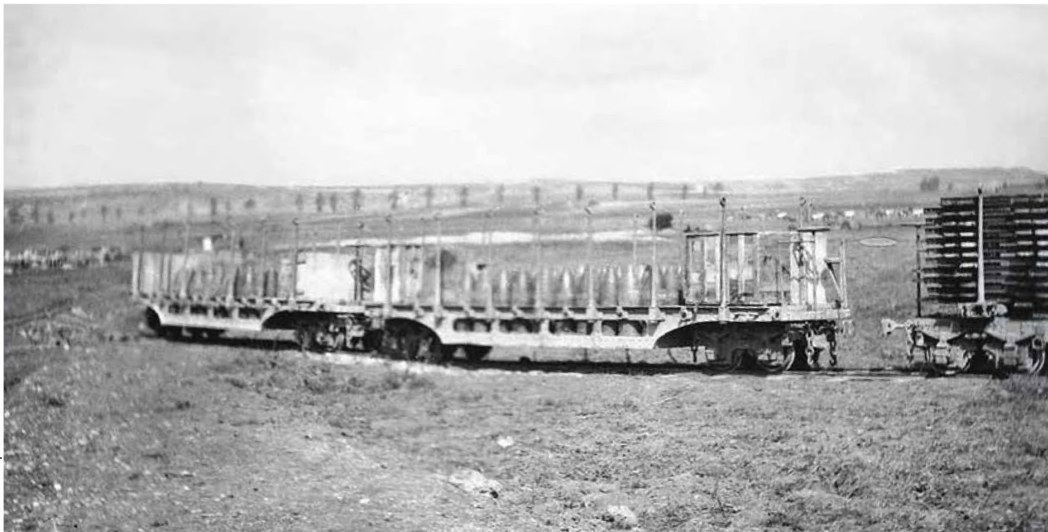
The first role of 60cm gauge track was to carry artillery ammunition. These two Péchat platforms are loaded with 220 calibre shells. The crates contain the proximity fuses.
