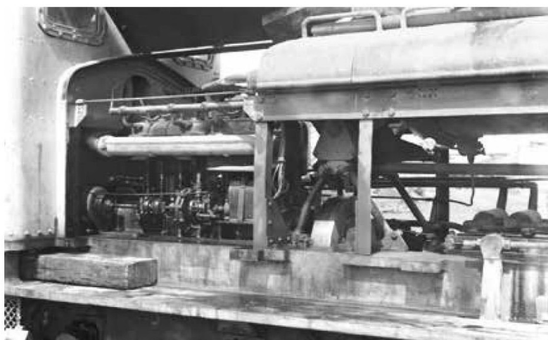
With the bonnets open, from left to right, the motor, flywheel and sandbox and the top of the gearbox, become visible.
