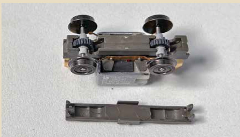
Once the keeper plate has been removed, the wheelbase can be modified. For re-gauging, the wheels must be pushed inwards on their axles. By pushing really hard, you can reach 9mm gauge.
