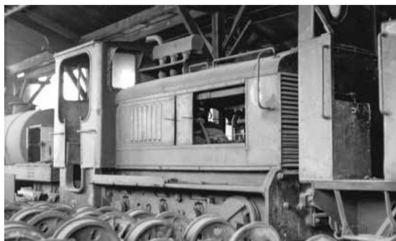
Villeron sugar mill used a Schneider tractor. Even re-motorized and with its body partly rebuilt, it remains quite recognizable.
