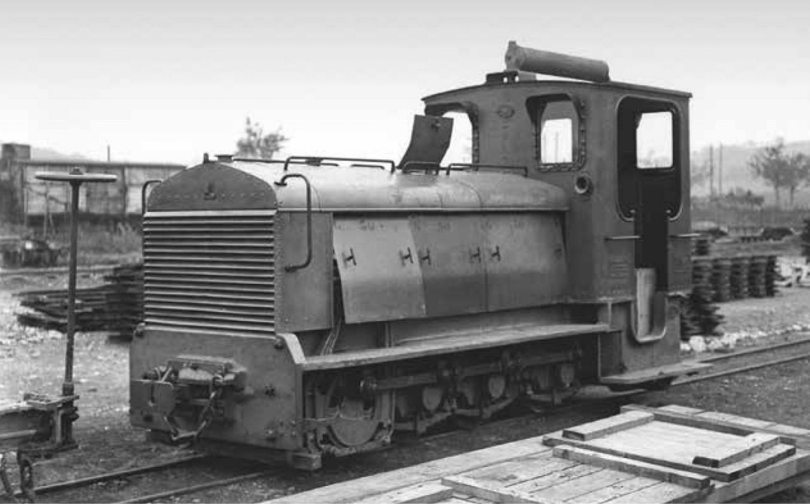
LG tractor N° 30 somewhere on the front. The markings on the bonnets are there to ease their dismantling and reassembly during maintenance.
