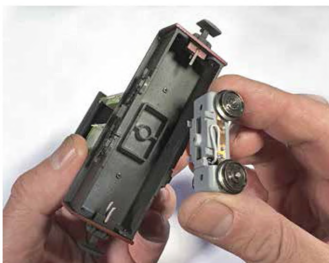
13 The motor unit fits in from below. It clip-fits onto the chassis.
