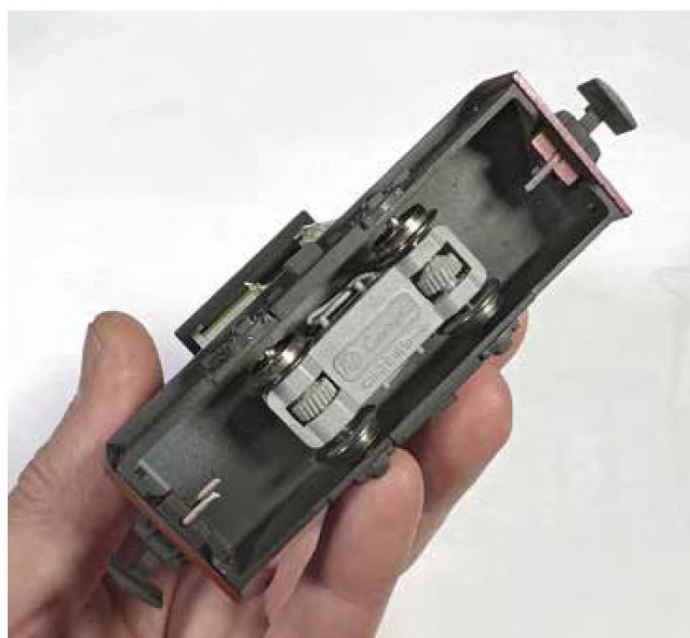
14 There is plenty of space to fit a simple decoder between the chassis frames.
