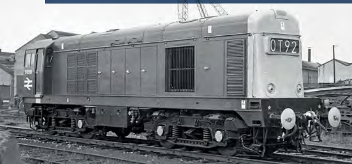
BELOW: Brand new Class 20 D8319 outside the Vulcan Foundry in September 1967. It entered service on January 27 the following year and is one of the examples delivered with air brakes fitted for use on Scottish MGR workings. (Rail Photoprints)
