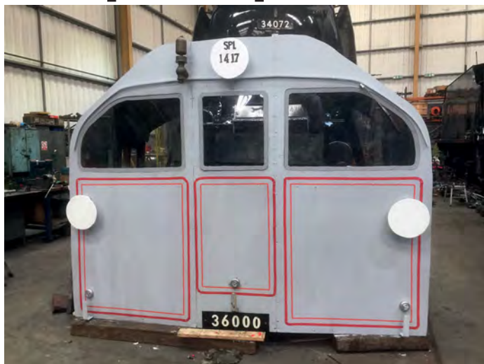
The Leader mock up at Herston Works was built using a wooden frame and cardboard. (Chris Worby)
