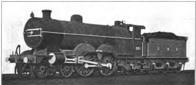
Fig. 5050. Ten-Wheel, Four-Coupled Locomotive. Great Northern Railway. Cylinders 19 in. x 24 in.; Working Steam Pressure 175 lbs. per sq. in.; Total Heating Surface 2,500 sq. ft.; Diameter of Drivers 80 in.; Weight on Drivers 84,640 lbs.; Total Weight 146,720 lbs.
