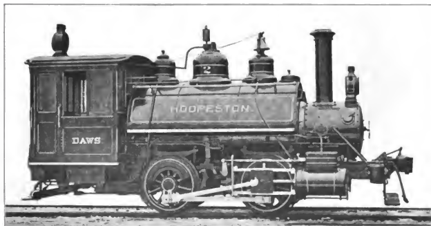
Fig. 6. Four-Wheel (0—4—0) Tank Switching Locomotive. Built by the Baldwin Locomotive Works for the Hoopes & Townsend Co. Cylinders 13 in. x 20 in., Working Steam Pressure 160 lbs. per sq. in., Heating Surface 414.71 sq. ft., Diameter of Drivers 42 in., Weight on Drivers 30,000 lbs., Total Weight 50,000 lbs.
