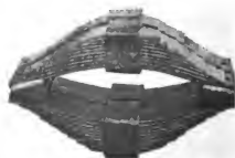
Fig. 1781. Elliptic Engine Truck Spring
