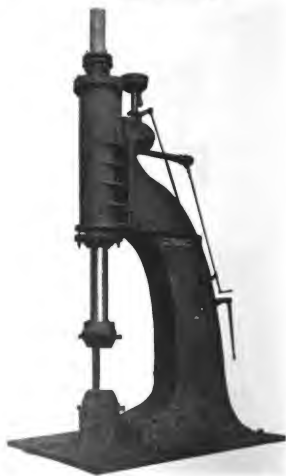
Fig. 4944. 2,000-lb. Single Frame Steam Hammer. William Sellers & Co., Inc.
