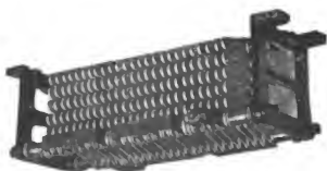
Fig. 4663. Grid Resistance. Westinghouse A. C. Electric Locomotive.
