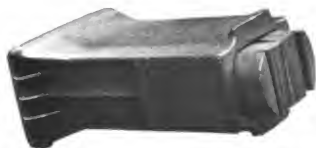
Fig. 3961. Gould Friction Draft Gear, Assembled.
