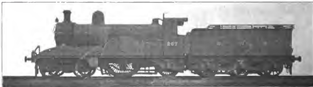
Fig. 5041. Eight-Wheel, Single Driver Locomotive. Great Northern Railway. Cylinders 19 in. x 26 in.; Working Steam Pressure 175 lbs. per sq. in.; Total Heating Surface 1,296.6 sq. ft.; Diameter of Drivers 92 in.; Weight on Drivers 49,760 lbs.; Total Weight 108,890 lbs.
