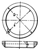
Figs. 239-240. Ground Washer for Dry Pipe Ball Joint.
