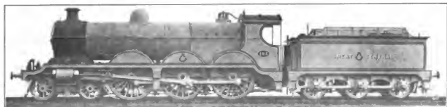
Fig. 5062. Ten-Wheel, Six-Coupled Locomotive. Great Central Railway. Cylinders 19½ in. x 26 in.; Working Steam Pressure 180 lbs. per sq. in.; Total Heating Surface 1,917 sq. ft.
