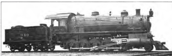
Fig. 47. Decapod (2-10-0) Tandem Compound Locomotive. Built by the Baldwin Locomotive Works for the Atchison, Topeka & Santa Fe. Cylinders 19 in. and 32 in. x 32 in., Working Steam Pressure 225 lbs. per sq. in., Total Heating Surface 5,300 sq. ft., Diameter of Drivers 57 in., Weight on Drivers 237,800 lbs., Total Weight 267,800 lbs.
