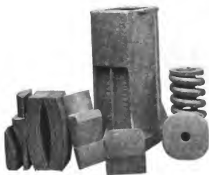
Fig. 3960. Gould Friction Draft Gear, Dismantled.
