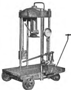
Fig. 4904. Portable Hydraulic Bushing Press. Watson-Stillman Co.
