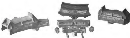
Figs. 4519-4521. Susemihl Roller Side Bearing American Steel Foundries.
