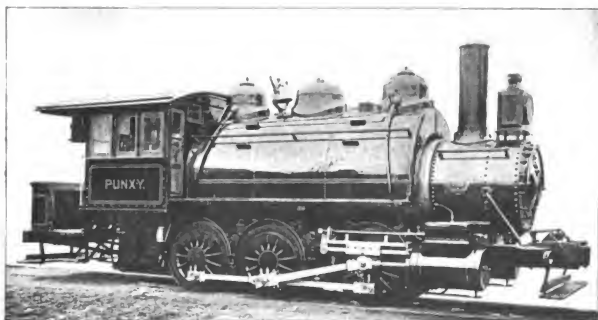
Fig. 14. Six-Wheel (0-6-0) Tank Switching Locomotive. Built by the American Locomotive Co. Cylinders 17 in. x 24 in., Working Steam Pressure 180 lbs. per sq. in., Diameter of Drivers 46 in., Weight on Drivers 96,000 lbs., Total Weight 96,000 lbs.
