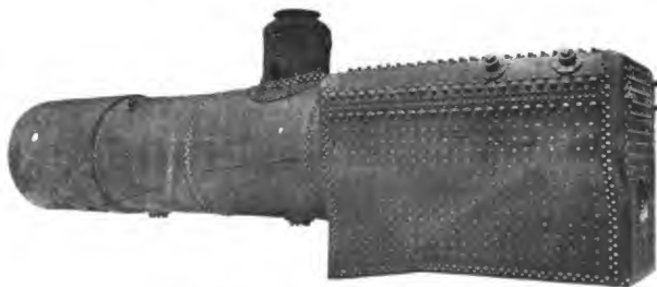
Fig. 148. Straight Top Boiler with Belpaire Firebox.
