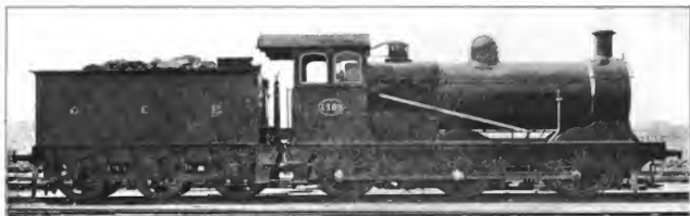
Fig. 5030. Six-Coupled Goods Locomotive. Great Eastern Railway. Cylinders-19 in. x 26 in.; Total Heating Surface 1,706.58 sq. ft.; Diameter of Drivers 39 in.; Weight on Drivers 102,680 lbs.; Total Weight 102,680 lbs.
