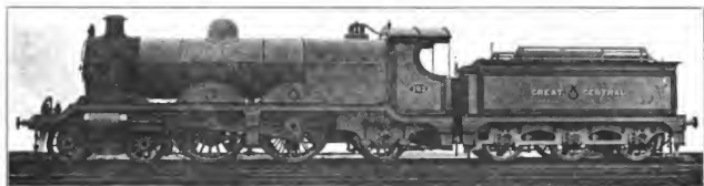
Fig. 5055. Ten-Wheel, Four-Coupled Locomotive. Great Central Railway. Cylinders 19 \frac{1}{2} in. x 26 in.; Working Steam Pressure 180 lbs. per. sq. in.; Total Heating Surface 1,931 sq. ft.
