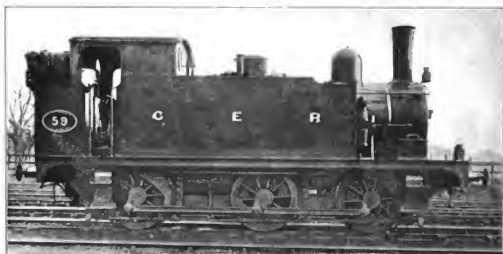
Fig. 5028. Six-Coupled Tank Shunting Locomotive. Great Eastern Railway. Cylinders 16\frac{1}{2} in. x 22 in.; Total Heating Surface 988.17 sq. ft.; Diameter of Drivers 48 in.; Weight on Drivers 95,100 lbs.; Total Weight 95,100 lbs.
