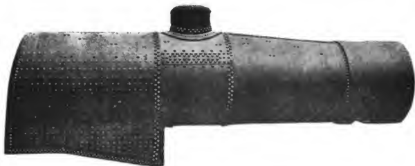
Fig. 145. Extended Wagon Top Boiler with Narrow Firebox.
