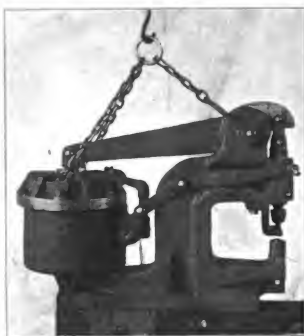
Fig. 4999. Portable Pneumatic Punch. Quincy, Manchester, Sargent Co.
