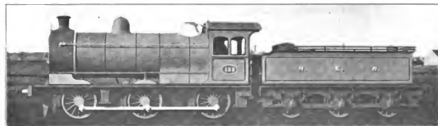
Fig. 5026. Six-Coupled Goods Locomotive. North Eastern Railway. Cylinders 18½ in. x 26 in.; Total Heating Surface 1,658 sq. ft.; Diameter of Drivers 55½ in.; Weight on Drivers 106,740 lbs.; Total Weight 106,740 lbs.
