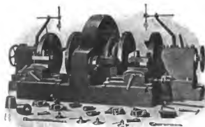
Steel-tired Car-wheel Lathe.
