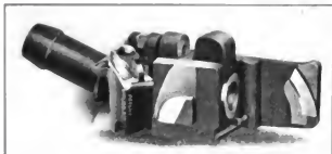
Fig. 3176. Sewall Steam Coupler, No. 20 AF.
