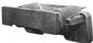
Fig. 3962. Gould Spring Buffer Plate.
