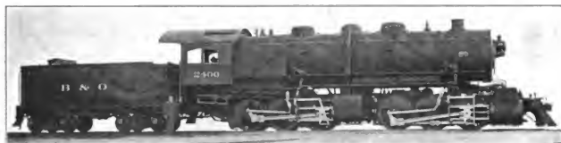
Fig. 22. Twelve-Wheel (0-6-0-0) Mallet Articulated Compound Locomotive. Built by the American Locomotive Co. for the Baltimore & Ohio. Cylinders 29 in. and 32 in. x 32 in., Working Steam Pressure 235 lbs. per sq. in., Total Heating Surface 5,585.7 sq. ft., Diameter of Drivers 56 in., Weight on Drivers 334,500 lbs., Total Weight 334,500 lbs.
