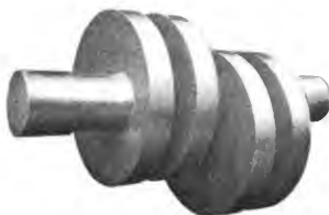
Fig. 2206. Built-up Disk Crank Axle.
