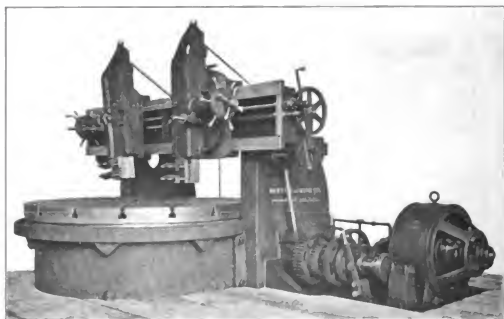
Fig. 4902. 84-Inch Tire Turning Mill. Betts Machine Co.
