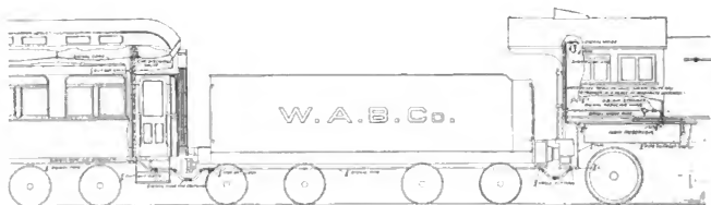
Fig. 2422. Diagram of Westinghouse Train Air Signal Equipment.
