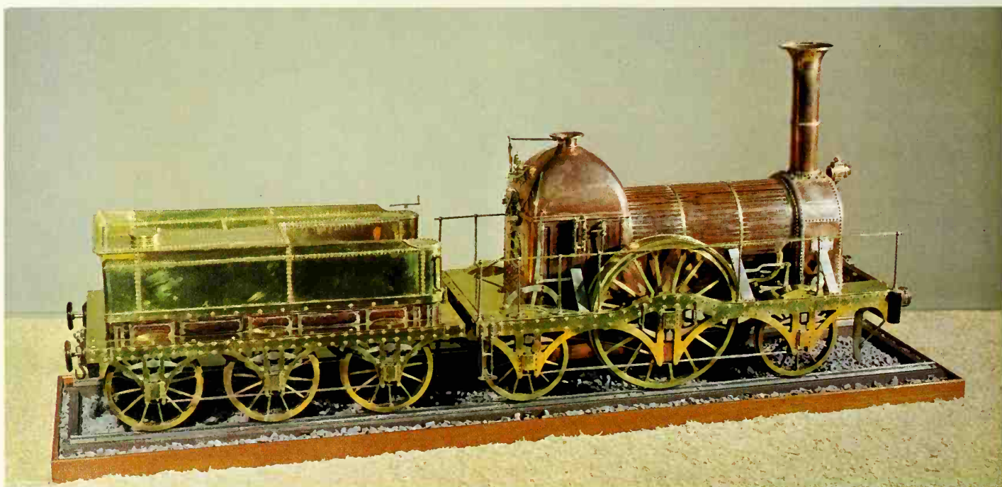
6 Contemporary model of the broad gauge locomotive 'Ixion', which was designed by Daniel Gooch and built for the GWR in October 1841. It was largely based on the design of North Star built by Robert Stephenson and Co. in 1837.
