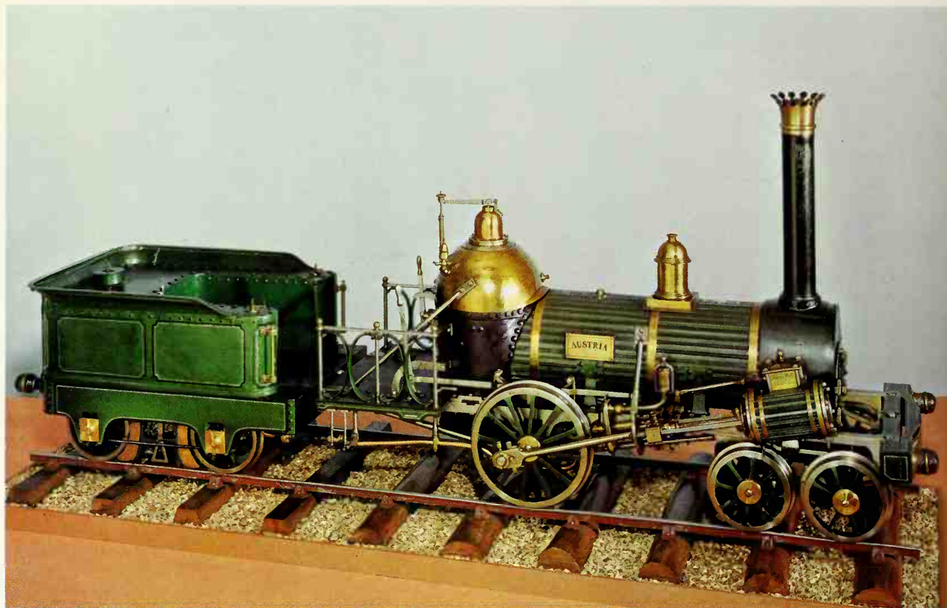
5 A model of a locomotive designed in 1843 by the American engineer William Norris, a Philadelphian, which has a special four-wheeled swivelling bogie for use on lines having steep inclines and sharp curves. Austrian railways acquired one of Norris's locomotives and named it 'Austria'.
