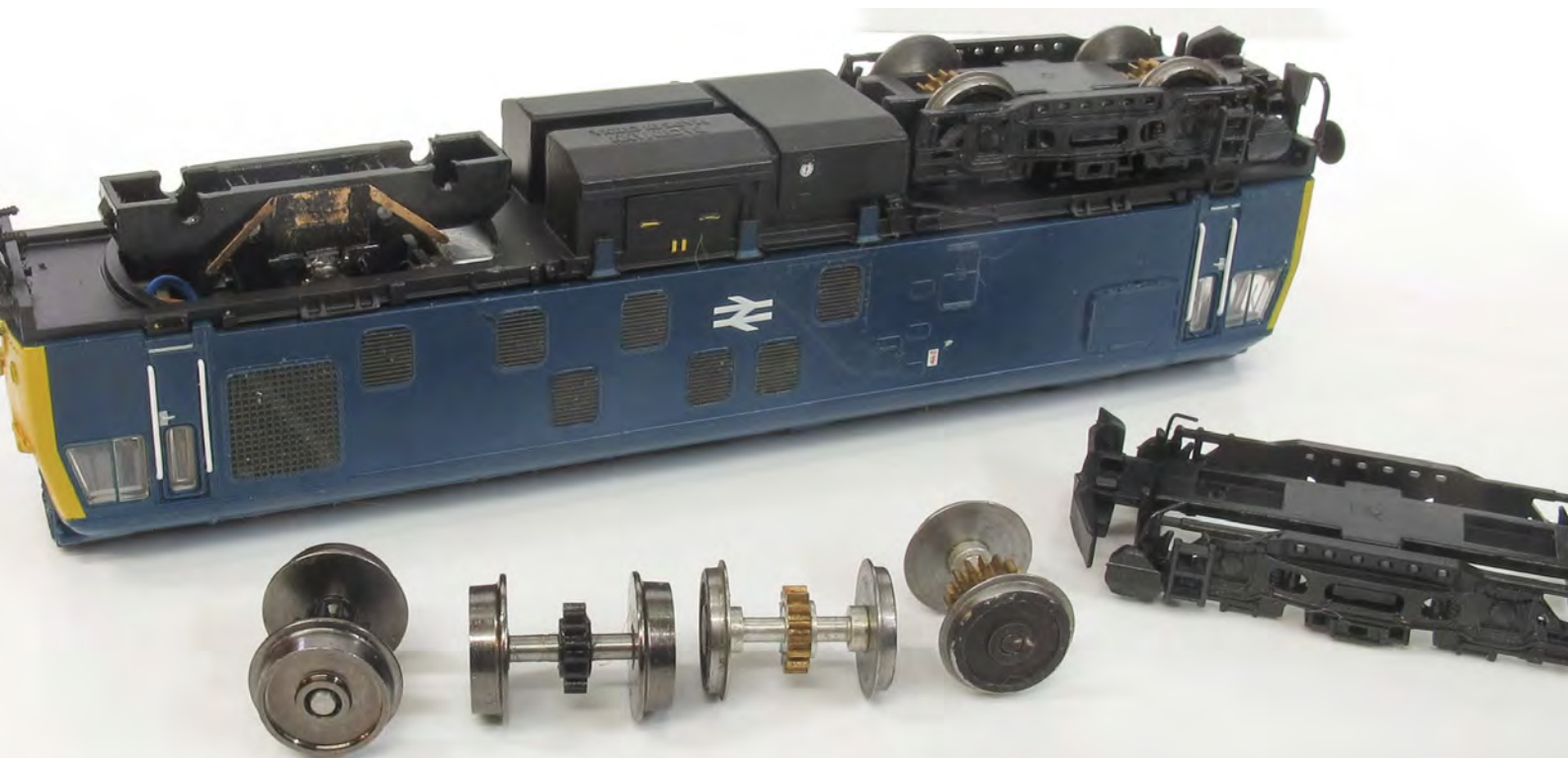
Farish Class 25 with 2mm Scale Association drop-in replacement wheels. The difference between a 2FS wheel and its N gauge counterpart is clear to see.
