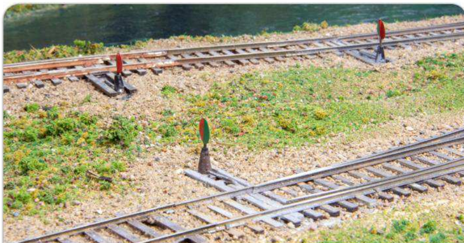
The switch stands along Skip's main line are made from double-pole double-throw (DPDT) slide switches that also control the frog polarity.
