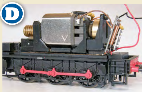
D This image of a partly dismantled 8-pin decoder socket assembly shows how much space this takes up within the model. The decoder can only be fitted vertically, and in this forward space. This restricts the choice of sound decoder to the miniaturised versions, the smallest commonly available one being the Zimo MX648.
