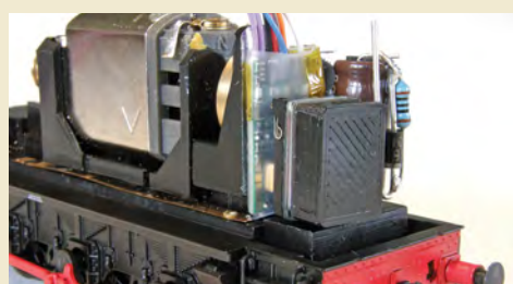
G I used Kapton tape to seal the cut insulation on the decoder which I then fixed in place with sticky mastic. The cube speaker and capacitor were also fitted in a dry run to ensure the body would refit without problem.
