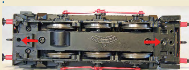
B After removing the tension lock couplings two body retaining screws are revealed. Take note of their orientation when you remove them as they are of different sizes.
