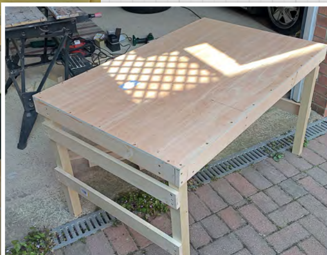
Above: All of the baseboards were built separately to pre-determined sizes using 9mm plywood for the surface and 69mm x 18mm planed timber for the frames. Legs are made from 44mm x 44mm timber.
