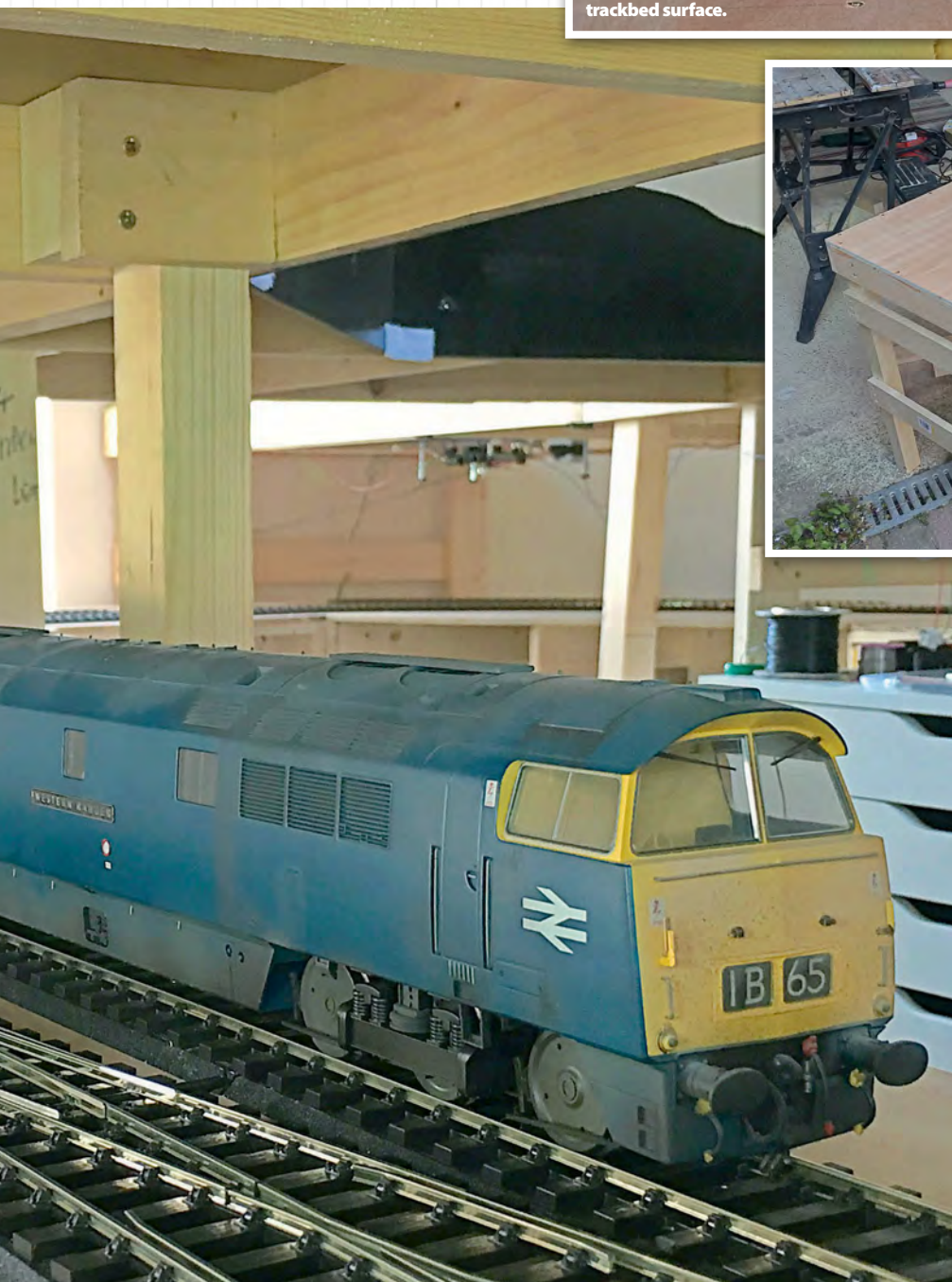
With the first two boards in place under the goods yard of Topley Dale tracks were placed to get a feel for how the height would look. 9mm plywood provides the trackbed surface.
