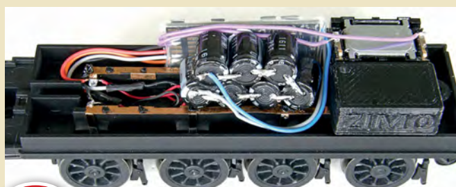
31 This home-made pack of seven 2.7v 1F supercapacitors has been wired in series to add their voltages together for safe operation at 16V.
