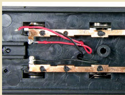
29 The wires from the locomotive pick-ups have been marked with white paint for easy identification. I soldered these plus the red and black wires from the decoder to the tender pick-up strips. I joined the orange decoder wire to the red motor wire from the 4-pin connector and the grey decoder wire to the black motor wire.
