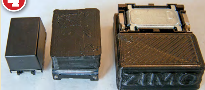
Zimo speakers from the left: 8mm x 12mm x 8mm, 11mm x 15mm x 9mm and 26mm x 20mm x 8mm. The largest of these will only fit in the eight-wheel tender model.
