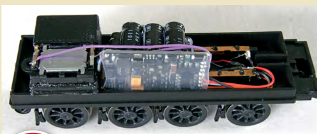
32 This alternative view shows the deployment of the components and the renewed wiring between the decoder and motor/track connections.
