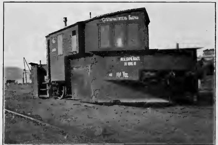
Snow Plough Commonly Used on Russian Railroads
