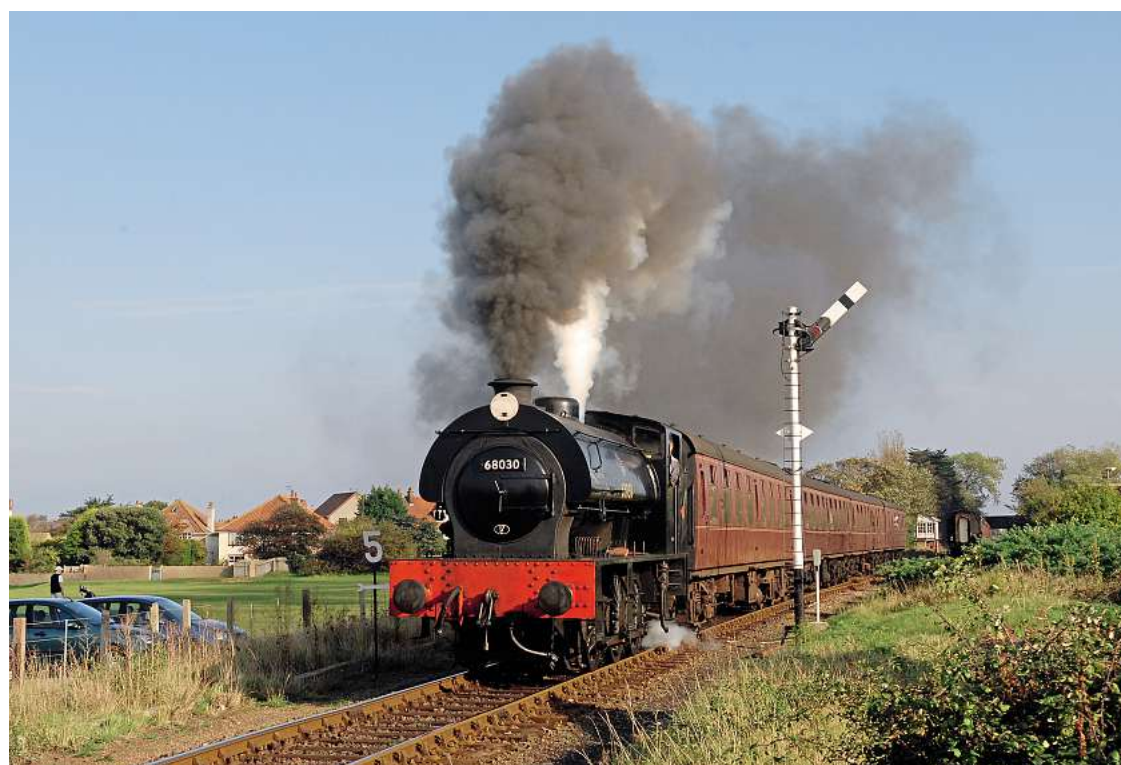
BELOW: No. 68030 departs from Sheringham on the North Norfolk Railway. The engine is in fact Hunslet-built Austerity 0-6-0ST No. 3777 which was never in BR stock.
