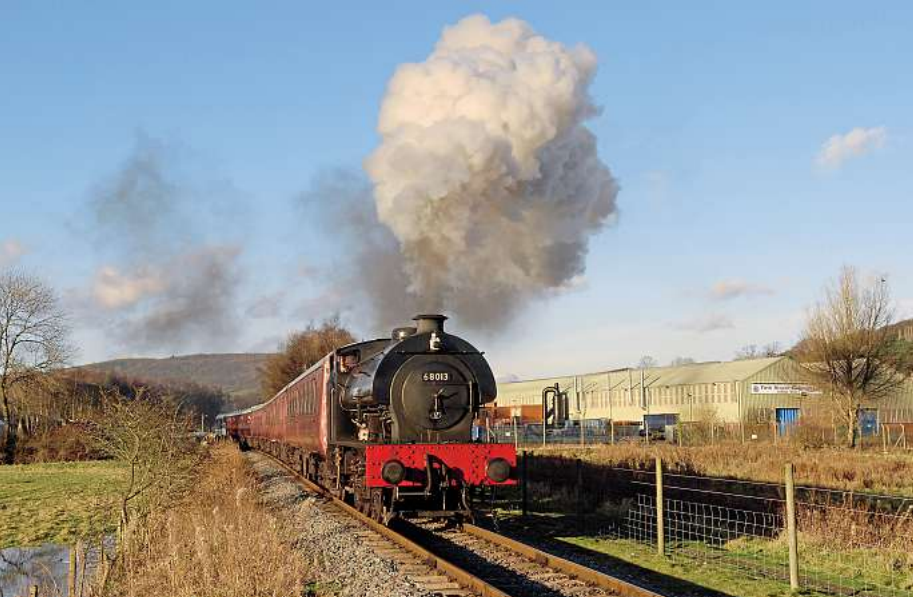
ABOVE: No. 68013, seen leaving Rowsley North on Peak Rail is in reality WD No. 150, Robert Stephenson & Hawthorns No. 7136 of 1944 which was rebuilt by Hunslets with a gas-producer firebox and underfeed stoker as late as 1969 and given a new works number 3892. It was sold straight into preservation at the Dinting Railway Centre.
