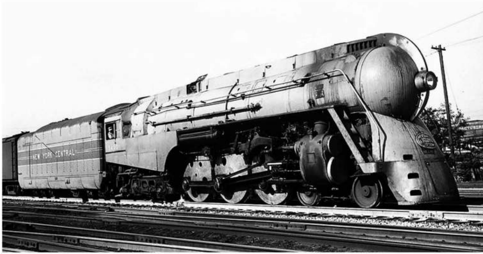
The New York Central's signature locomotive was the Henry Dreyfuss-designed Hudson, with a 4-6-4 wheel arrangement. Streamlined locomotive No. 5450 celebrates Independence Day on July 4, 1941.
