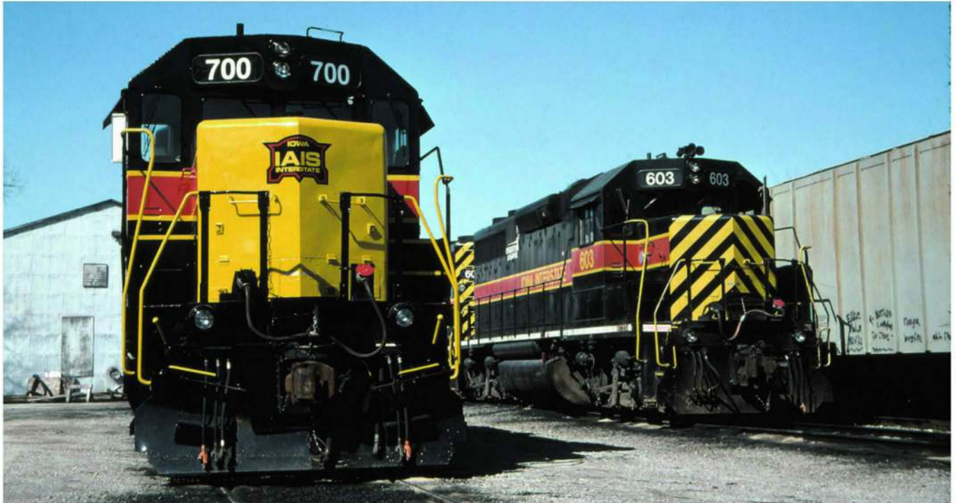
Both of these Iowa Interstate locomotives are variations of EMD's GP38. No. 603 is a GP38, while No. 700 is a GP38-2.
