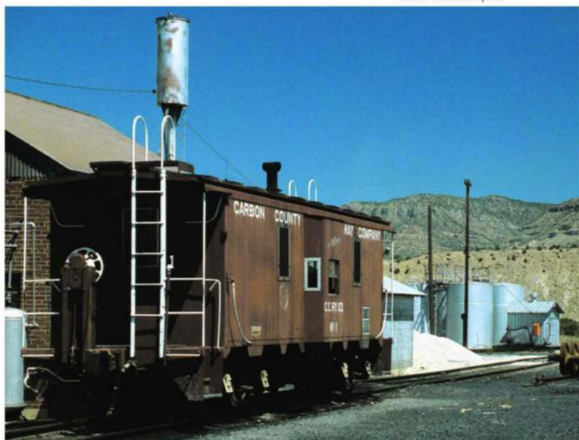
Above: When increasing freight car heights made the roof-mounted cupola useless as an observation post, some railroads built bay-window cabooses such as this one at the Carbon County Railway in Utah.
