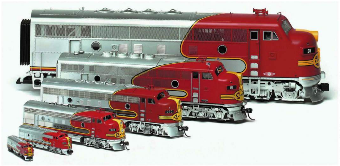
The relative sizes of different modeling scales are shown, represented by the same standard gauge prototype locomotive. From left to right are Z, N, HO, S, and O scale locomotives, followed by the largest, a G gauge diesel locomotive.
