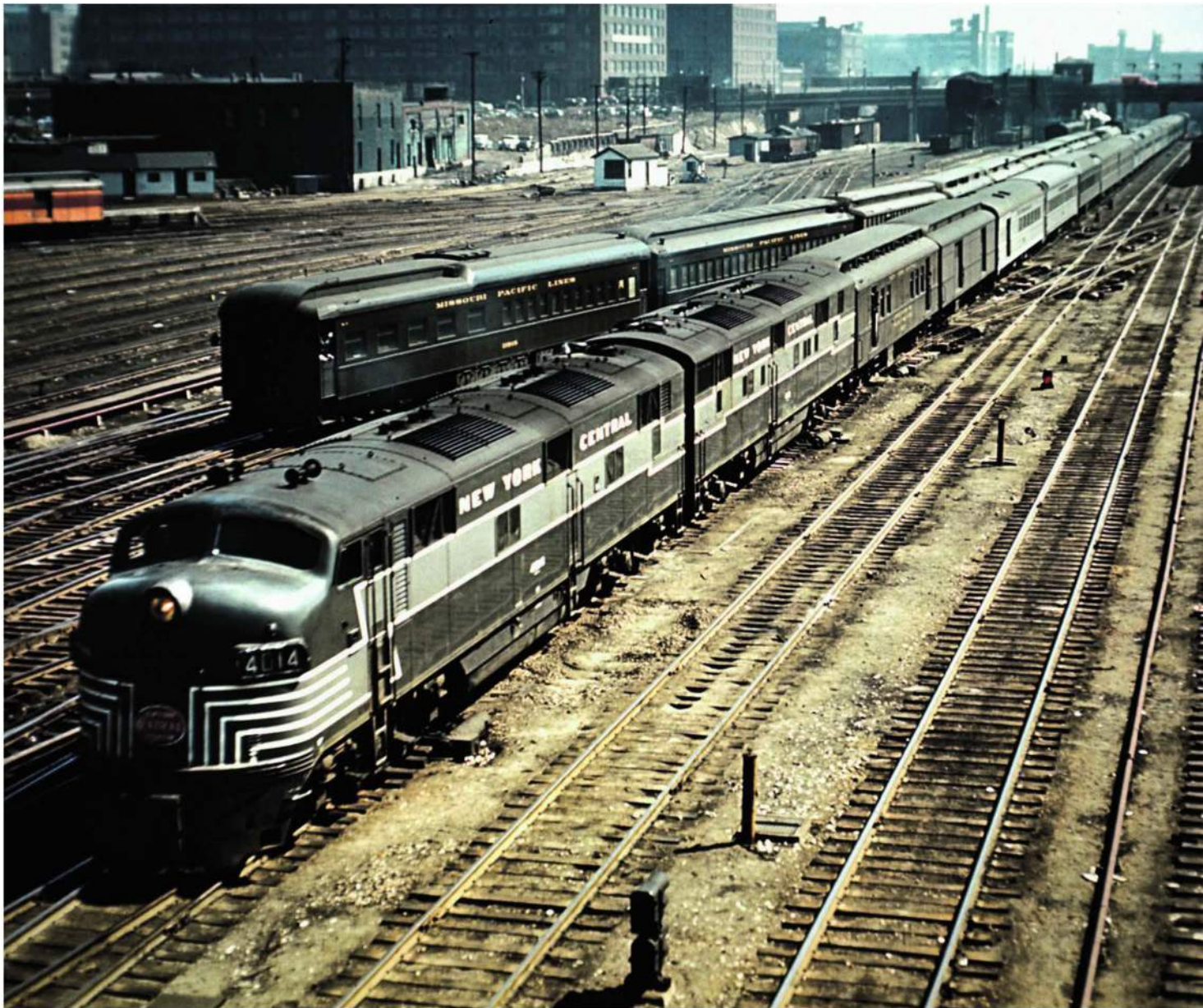
New York Central E7 locomotives leave St. Louis with a streamlined train (save the two older baggage cars directly behind the locomotive). Passing in the opposite direction is a steam-hauled Missouri Pacific passenger train.
