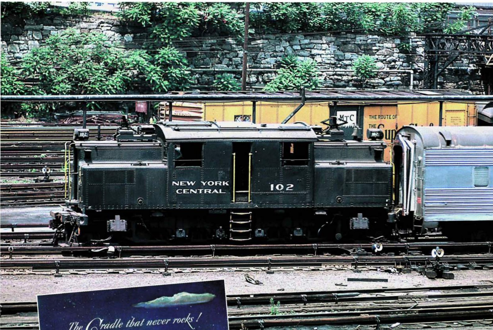
Above: Smoke abatement laws were the impetus for converting to electric-powered locomotion in many large cities. Electric locomotives replaced steam locomotives before a train entered the city. Here is an example of that process, with a New York Central ES1 locomotive hauling a passenger train through The Bronx in July 1962.
