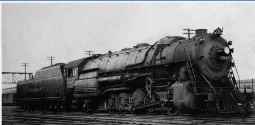
READING COMPANY NO. 3017 2-10-2 REBUILT FROM 1800 SERIES MALLETS
