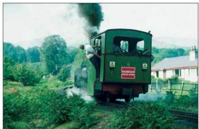
Bottom right: No 8 being taken up the line on test on 23 August 1984. The spikes with warning triangles were carried on the locos to be dropped off if the loco crew noticed a track defect.
