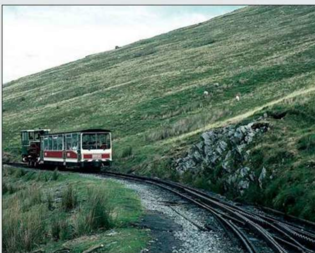
Left: A modern train about to enter the loop at Halfway, No 10 and carriage No 10 on 10 August 1989. The carriage had just entered service. At 2¼ miles from Llanberis, the gradient here is 1 in 11.
