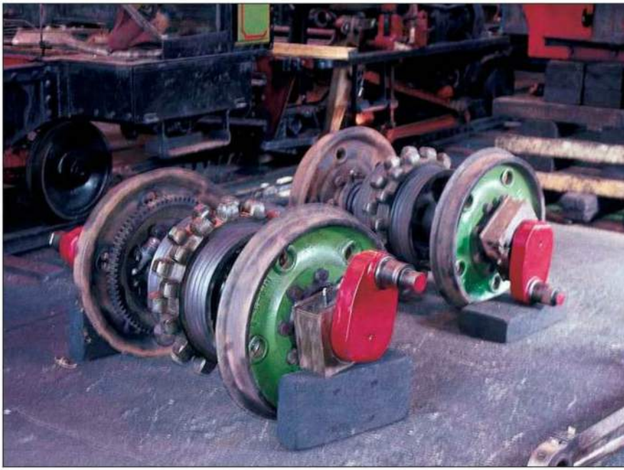
Left: A pair of loco wheelsets. The pinions last 18 months in service. 1 September 1992.
