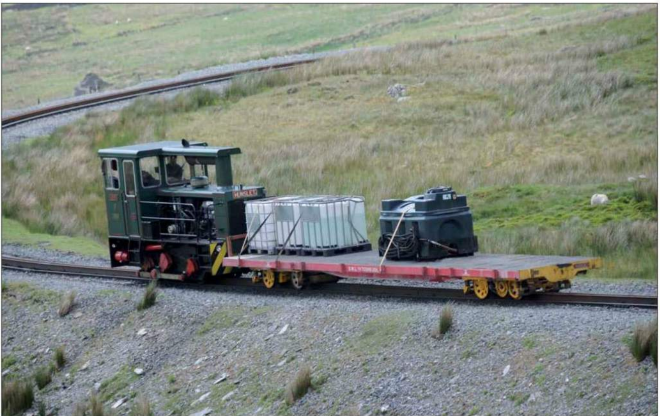
Below: With the completion of the summit building works the Hunslet wagon is used to carry water and fuel to the summit. On 13 June 2009, it was seen near Halfway with 3000l of water and 1,000l of fuel. The loco was No 9. Andrew Hurrell
