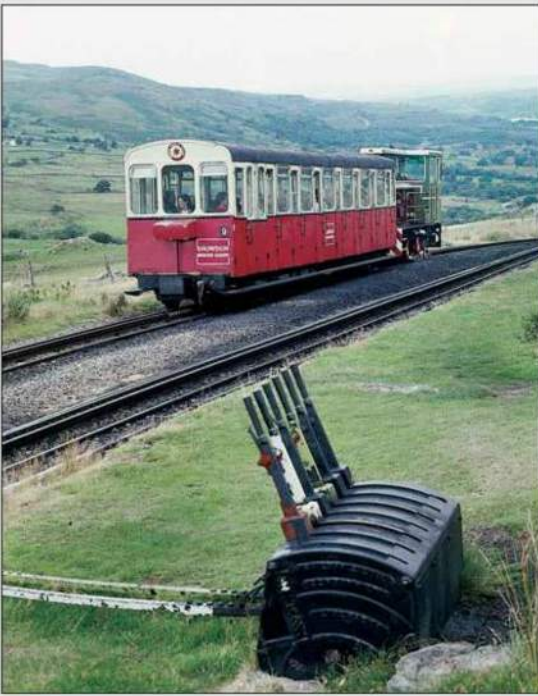
Left: The groundframe dominates this view of No 9 and carriage No 7 at Hebron, on 19 August 1989. Just over 1 mile from Llanberis, the gradient changes from 1 in 6 to 1 in 10.
