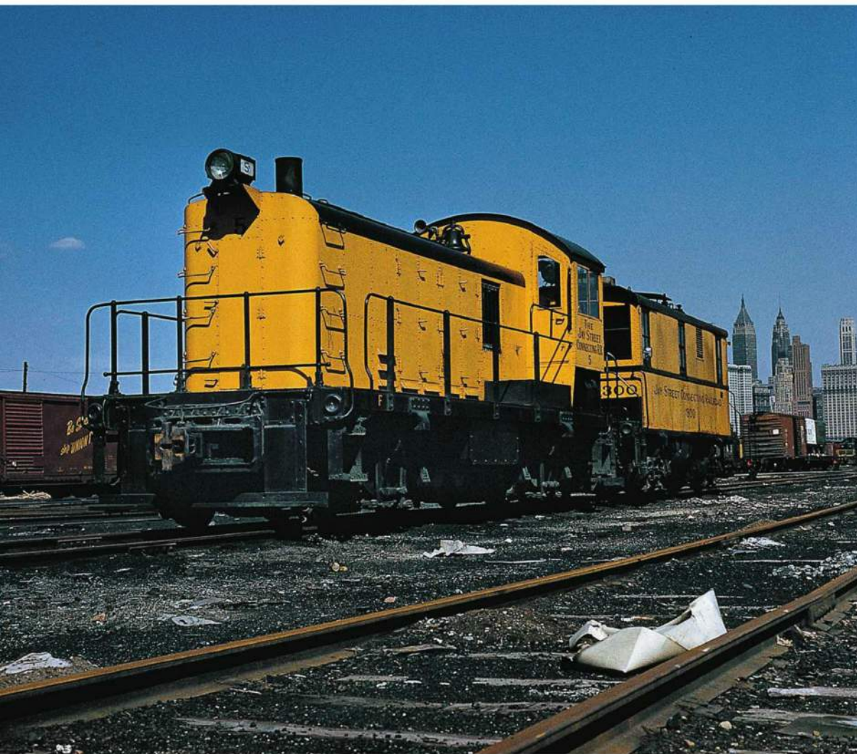
New York's Jay Street Connecting Railroad operated a variety of historically significant diesels. No. 5 is one of the early Alco hood-style switchers powered by the 531 diesel, while No. 300 is Alco's very first production diesel and the only boxcab switcher built after Alco left the GE-IR consortium. Richard Jay Solomon
