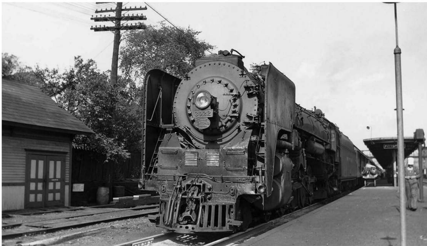
New York Central L3a No. 3022 pauses at Pittsfield, Massachusetts, with westbound passenger train No. 49 on September 12, 1948. This L3 class was built by Alco in 1940 and, like most Mohawks, had 69-inch drivers. The front coupler is lowered into the pilot, a standard safety precaution on many of the Central's modern steam designs.
