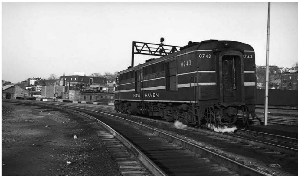
This rare photograph shows the back of New Haven DL109 No. 743 backing onto its train at Providence, Rhode Island, in the early 1950s. The New Haven assigned DL109s singly and in pairs to its Shoreline passenger services. Observers who witnessed the locomotives working full-throttle at speed noted they had a distinctive turbocharged whistle that sounded quite different from other 539-powered engines. Both Leo King, courtesy Center for Railroad Photography and Art
