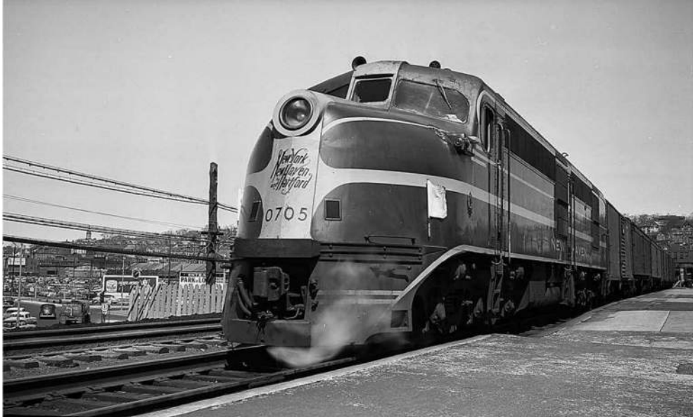
New Haven DL109 No. 705 leads an extra train at Providence, Rhode Island, in the early 1950s. The New Haven's 60 DL109s represented the bulk of Alco's production. These worked passenger services on the 157-mile run from Boston's South Station to New Haven, where electrics took over for the rest of the journey to New York City. Because they were intended for dual service, they used 19:64 gearing and GE-726 traction motors for 80 miles-per-hour maximum speed.
