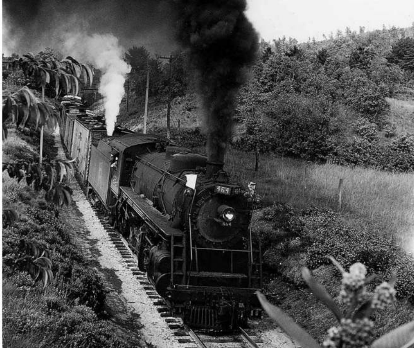
Central Vermont 2-8-0 No. 464 climbs with an extra freight at Smiths Bridge in Monson, Massachusetts. Working Stateline Hill's 1.27 percent grade makes for a good show. Notice the exhaust steam from the tender, which indicates the booster engine is working to give the locomotive extra tractive effort.
