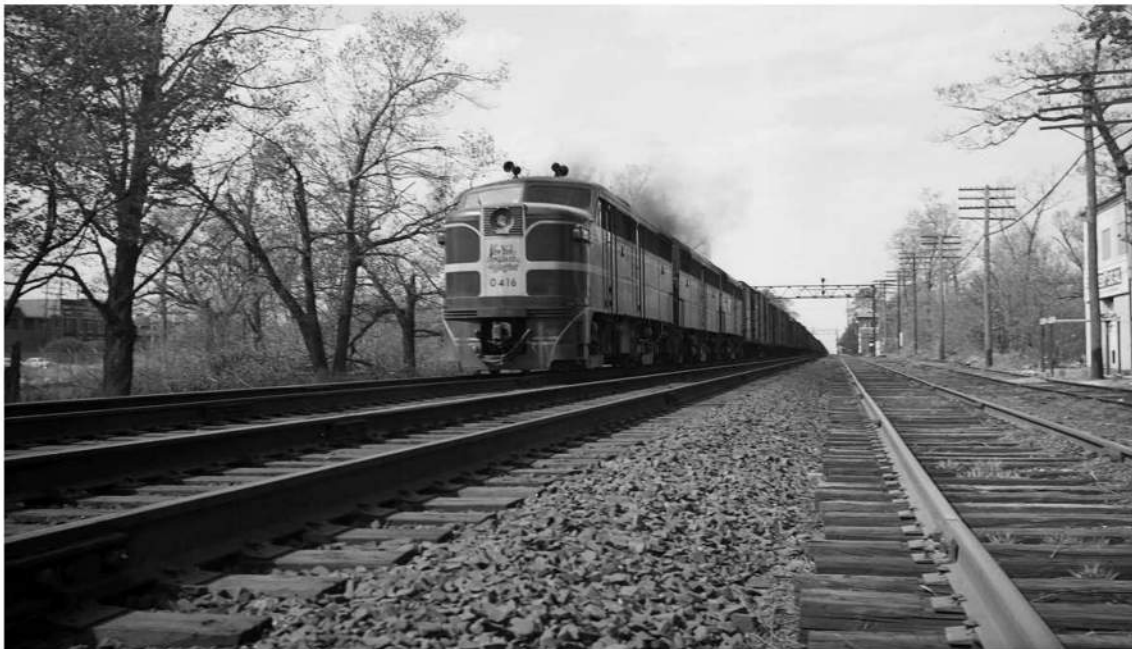
New Haven No. 0416 leads an A-B-A set of Alco FA-1s on the Shoreline with a long road freight at Warwick, Rhode Island, in the mid-1950s. New Haven bought a substantial fleet of Alco diesels, operating them in all types of service. Its final Alcos were C-425s built in 1964. Leo King, courtesy Center for Railroad Photography and Art
