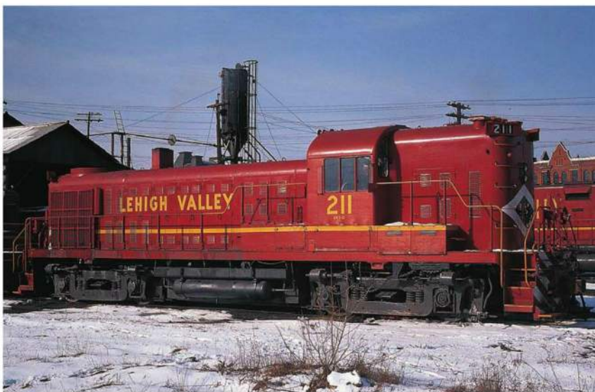
Originally Pennsylvania Railroad No. 8445, this was the railroad's sole RS-3 equipped with both dynamic brakes and a steam generator. The Penn Central later traded it to the Lehigh Valley, which renumbered it No. 211 (filling the spot in the LV's roster previously occupied by an RS-2). The unusual locomotive survived into the Conrail era and was rebuilt with a 12-567 engine as an RS-3m by Altoona shops. In the mid-1980s, it was bought by a private party and later donated to the Rochester Chapter National Railway Historical Society. In March 1975, it was photographed at Sayre, Pennsylvania. In 1990, it was repainted in Lehigh Valley paint and is maintained in operable condition at the museum at Industry, New York. Doug Eisele
