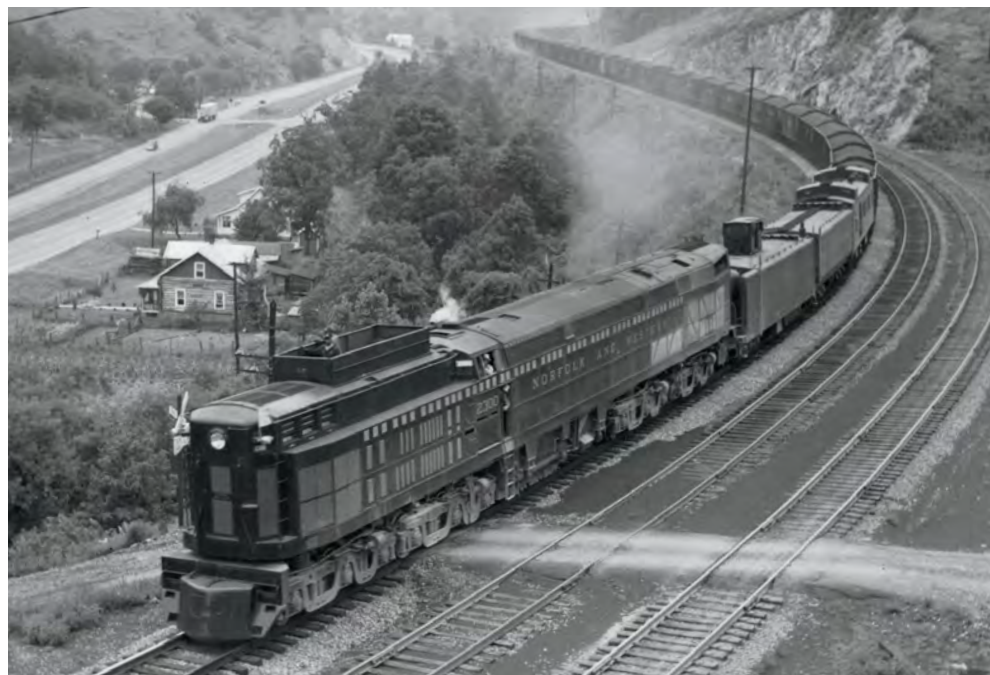
Steam-turbine-electric No. 2300 Jawn Henry —N&W's bid for a coal-fired future—drops down Christianburg Hill with its own doghouse-equipped water tender, an extra canteen, the road's dynamometer car, and tidewater-bound coal loads. LeRoy A. Scott
