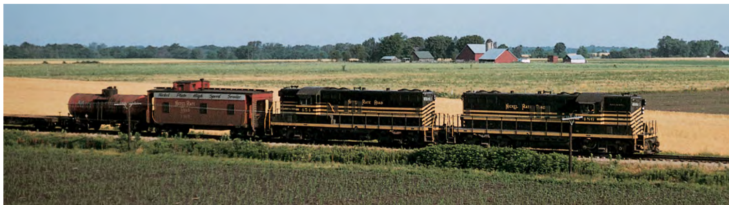
EMD was late to the road-switcher party, but it soon swamped the other builders. Its 1,500-h.p. GP7 of 1949 sold to the tune of 2,729 units before being succeeded in 1953 by the 1,750-h.p. GP9, of which 4,257 were built. Diesels like these two Nickel Plate GP9's, handling a local freight approaching Madison, Ill., in 1958, finished off the famous NKP Berkshires. M. L. Powell, J. David Ingles collection
