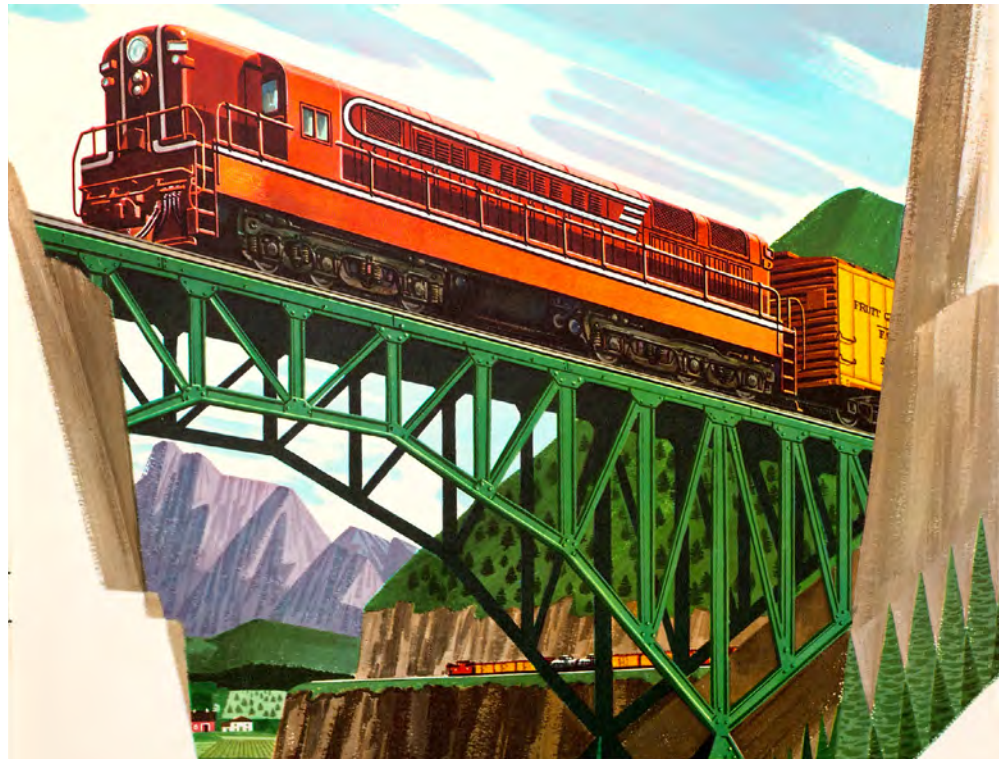
At 2,400 h.p., Fairbanks-Morse's six-motor H24-66 "Train Master" was by far the most potent road-switcher of its day. Production spanned 1953-57 and totaled 127 units; in all, 186 FM-design C-C road-switchers were built (plus 30 A1A-A1A's), the first in 1951. FM
