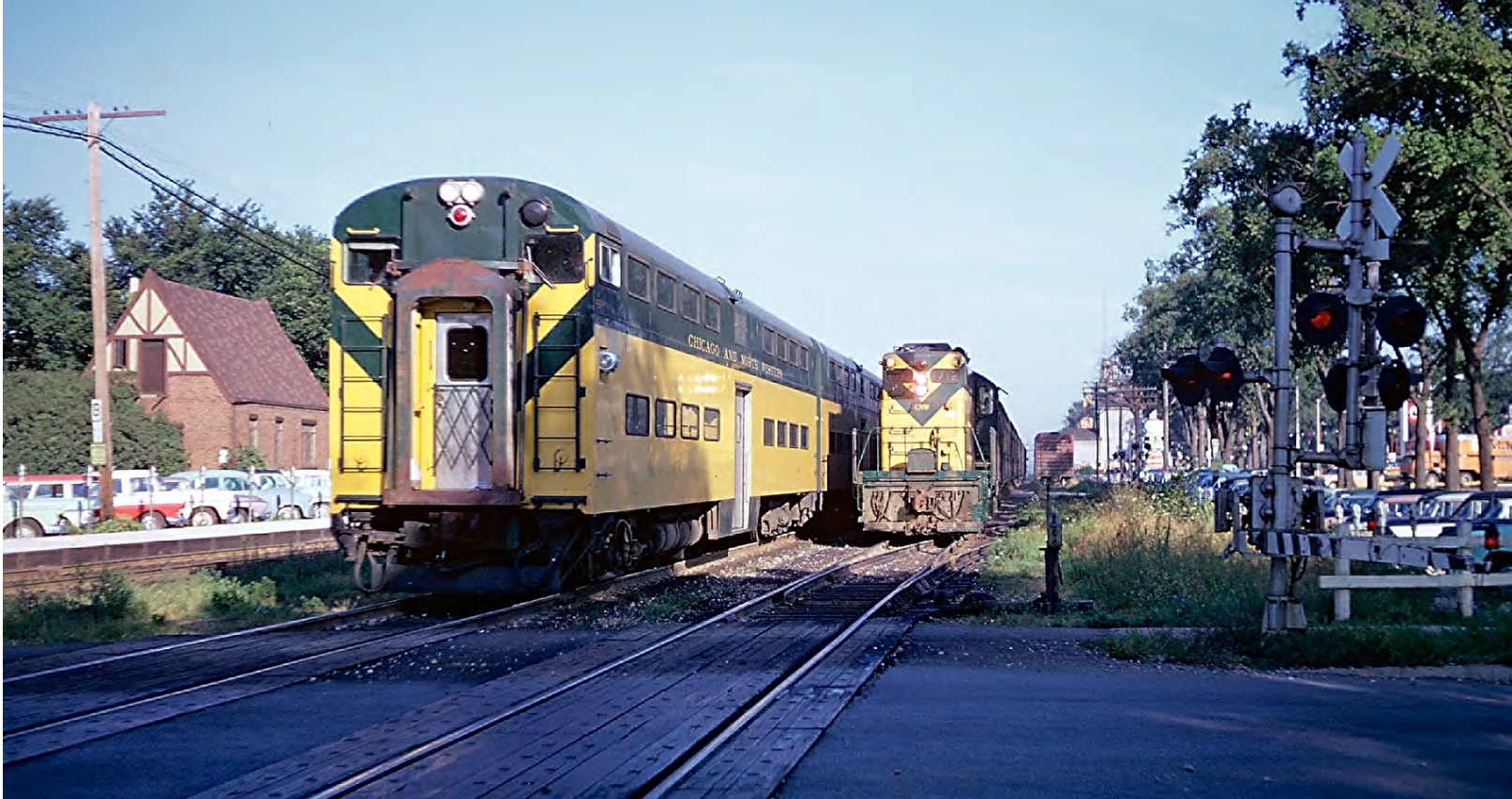
Burlington introduced the bilevel “gallery” car in 1950 for its Chicago suburban service, followed in 1955 by C&NW (above, at Arlington Heights in August ’61) and SP. The idea proved more durable than other ’50s cost-cutting concepts like ultra-lightweights. Bob Johnston
