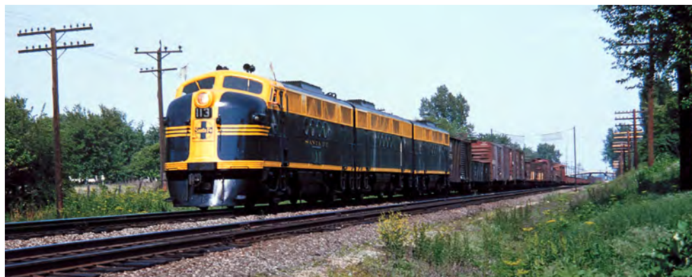
GALESBURG, ILL., JUNE 3, 3:37 P.M.: Near the CB&Q's bridge over the Santa Fe, and six minutes before the Burlington FT's passed, an A-B-B set of Santa Fe FT's rolls 127 cars west. Santa Fe's 320 FT's constituted the first big fleet of road freight diesels.
