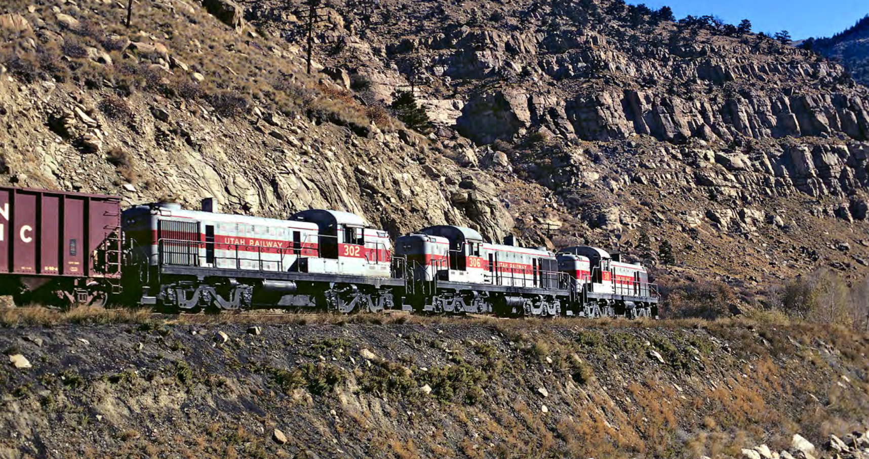
Alco's first C-C (six axles, all powered) road-switchers were the modified RS1's for the Army in 1942–45 (plus 6 for Mexico in '46). Although it built A1A-A1A (six axles, four powered) units for weight distribution beginning in 1946, Alco's first domestic C-C's came in '51. Three such 1,600-h.p. units (two RSD4's bracketing an RSD5) descend Solider Summit with a Utah Railway train in 1970. J. David Ingles
