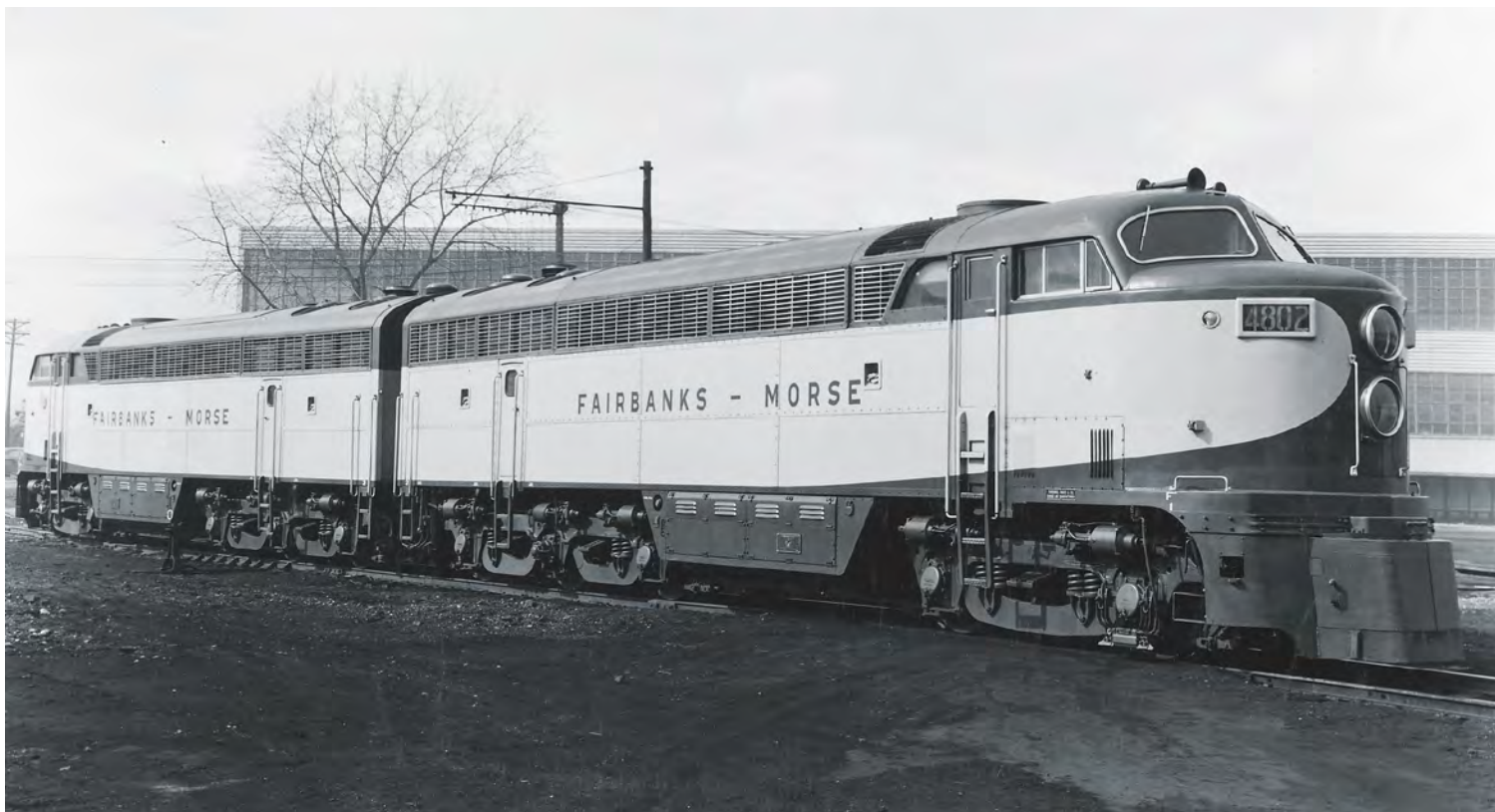
Fairbanks-Morse's two-unit set of 2,400-h.p. B-A1A C-Line cabs, painted in two-tone green and numbered for their aggregate horsepower, poses at its Beloit, Wis., birthplace before hitting the demonstration trail. Fairbanks-Morse
