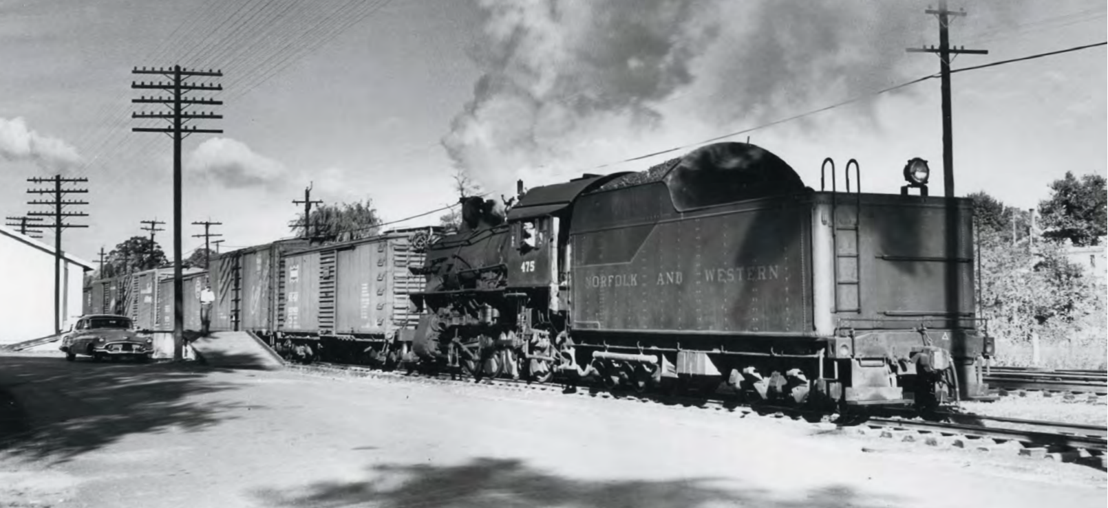
Rare elsewhere, the 4-8-0 was N&W's top freight engine until 1910, when the first articulateds arrived. Out of an original fleet of 286 Twelve-Wheelers, by 1954 three dozen remained, including 1906-built 475, switching at Potts Valley Junction on the Radford Division.
