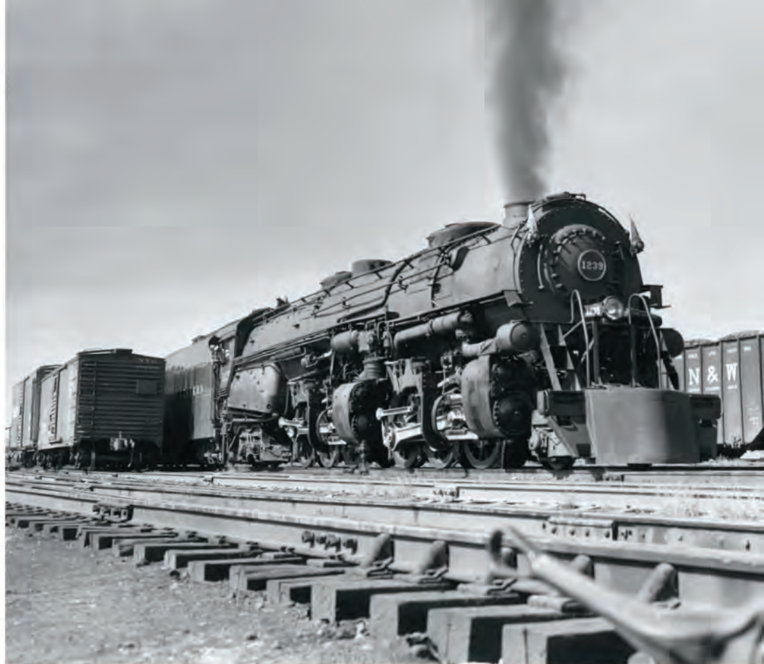
N&W's top fast-freight engines were 43 class A simple-articulated 2-6-6-4s. No. 1239, built in 1949 as part of the final A order, couples to time freight 84 at Roanoke.
