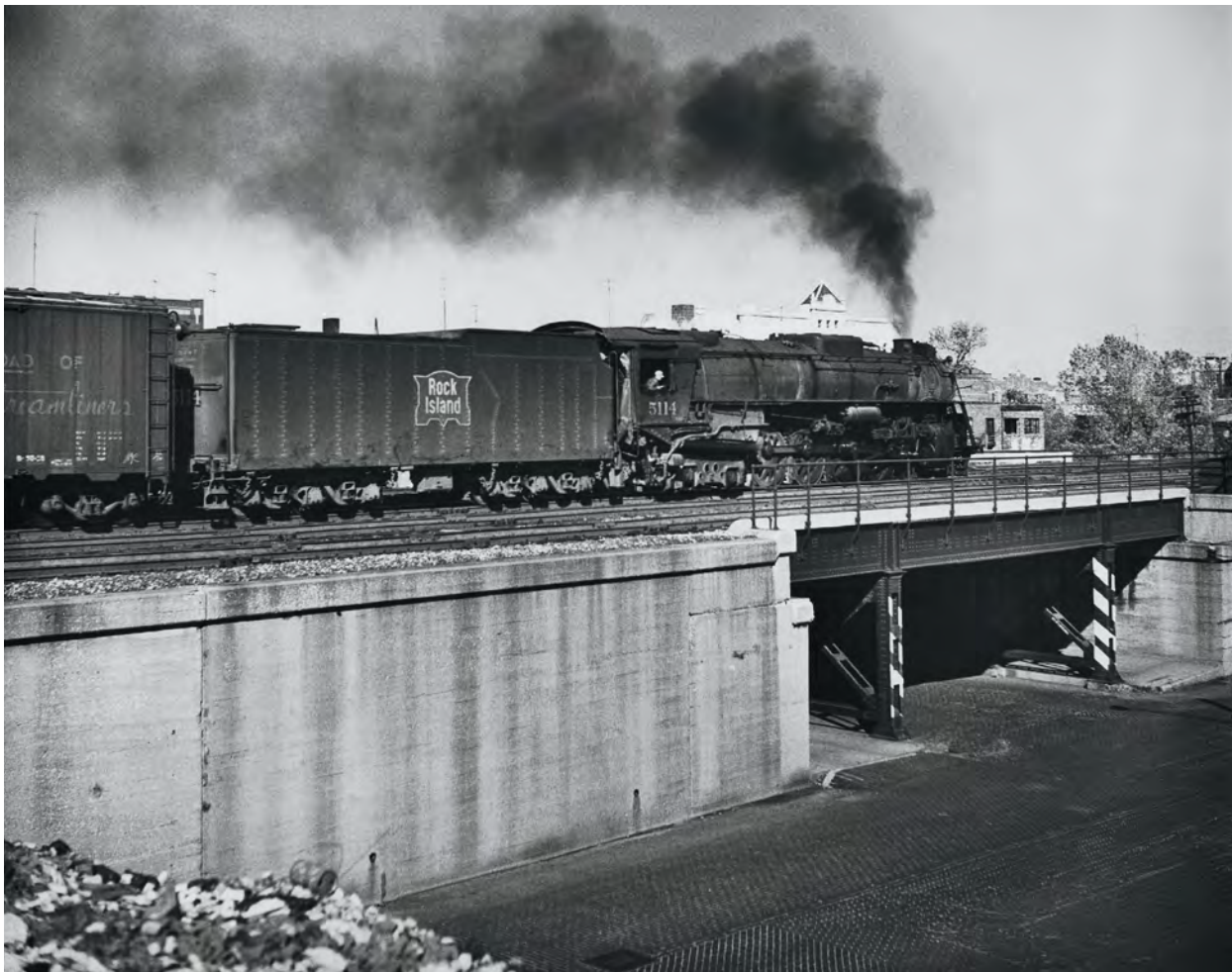
Another afternoon photo looks northeast from the GM&O right of way as Rock Island R-67-class 4-8-4 No. 5114 steams through with an eastbound freight. RI bought 85 4-8-4s, largest fleet in the U.S. All came from Alco, in 1929 (25), 1930, (40), 1944 (10), and 1946 (10). Originally intended just for freight work, they became good dual-service machines as RI standardized them with 74-inch drivers. Some led short lives, as RI dieselized in 1953.
