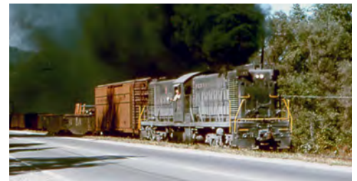
Lima's only C-C's were 22 twin-engined 2,500-h.p. units for PRR; they were transfer units, not general-duty road-switchers. Fred D. Cheney Jr.; William D. Volkmer collection
