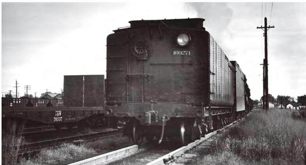
By adding 16,000 gallons of water capacity, canteens like this one with class A No. 1239 boosted tonnage ratings, cut running times, and enabled the closure of water stations.
