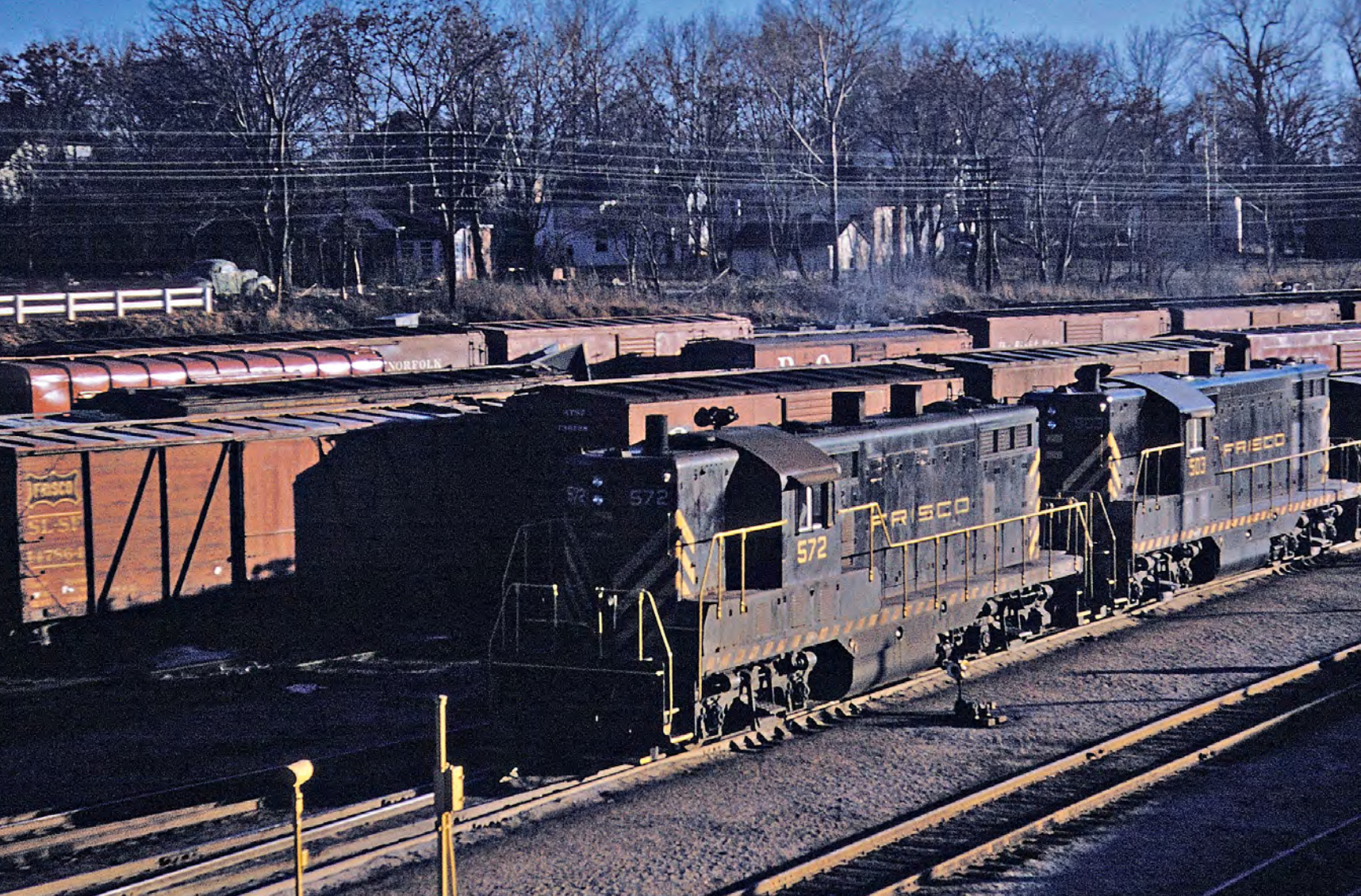
Road freight: In 1958, Frisco GP7's 572 and 503 arrive at Lindenwood Yard west of St. Louis. The stacks on their short hoods indicate they have steam generators for passenger work. Frisco, early to dieselize, had 128 GP7's but no GP9's. R. R. Wallin; J. David Ingles collection
