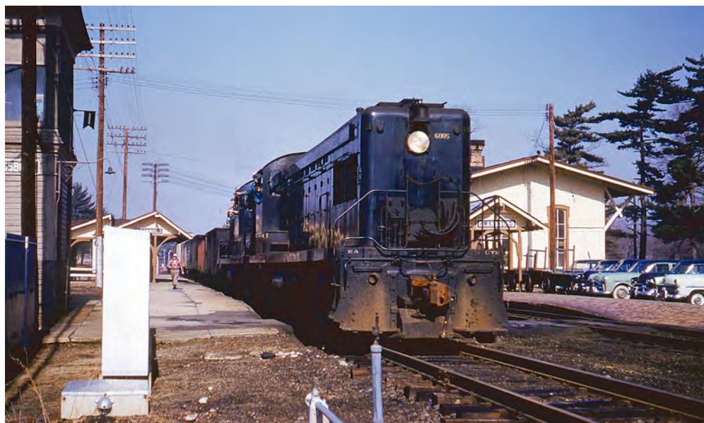
Baldwin built its first road-switchers in 1947, eventually producing 277 B-B (four axles, all powered) versions before quitting the market in 1956. Two dual-service Pennsylvania-Reading Seashore Lines AS16's work a freight at Glassboro, N.J., in 1955. Frank Kozempel
