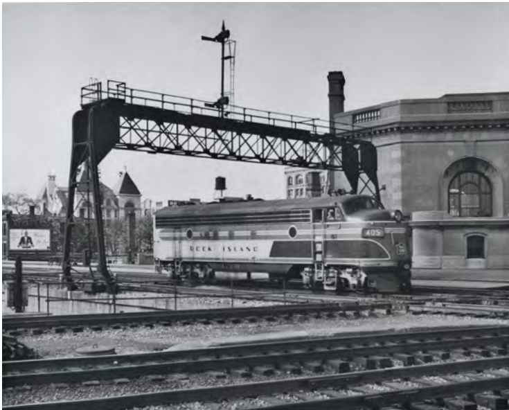
In a view looking northwest, FP7 405, one of RI's 10, has cleared the diamonds as it backs in from the coach yard to the east to couple onto its suburban train. Alco RS3's have just supplanted some FP7's here, but RI also employs the FP's on intercity trains.
