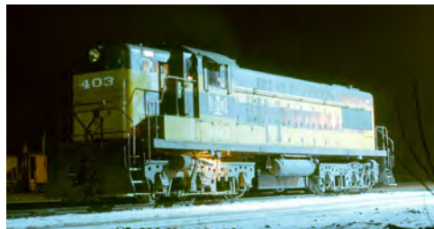
The first of Baldwin's 308 C-C's (including 70 transfer units, but not 50 A1A-A1A road-switchers) was the DRS-6-6-1500 of 1948; Bessemer 403 rests in 1970. Eric Hirsimaki
