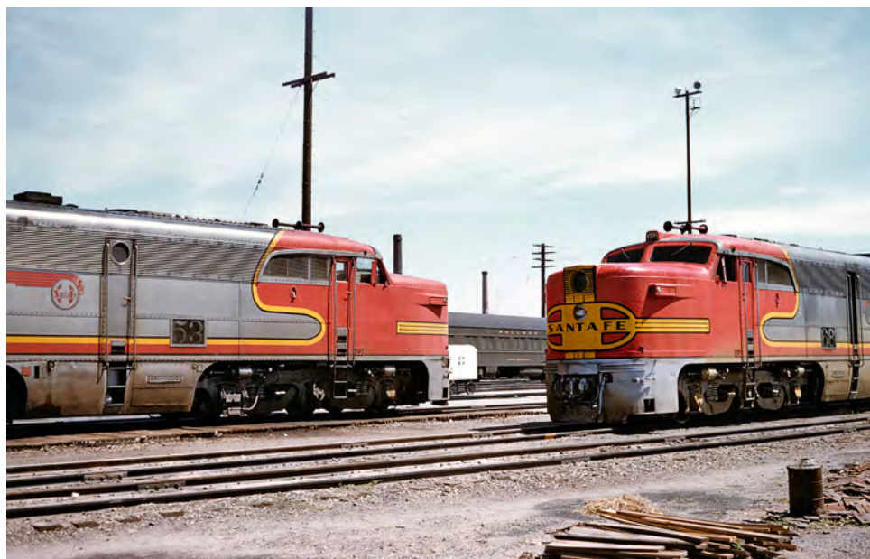
Favorites face to face: Two of Santa Fe's 44 Alco PA passenger units (including 16 B's) meet in La Junta, Colo., on August 8, 1954. Four of the classics survive, after a second career on Delaware & Hudson: two in Mexico and one each in Oregon and a museum in Frisco, Texas. Al Chione coll.
