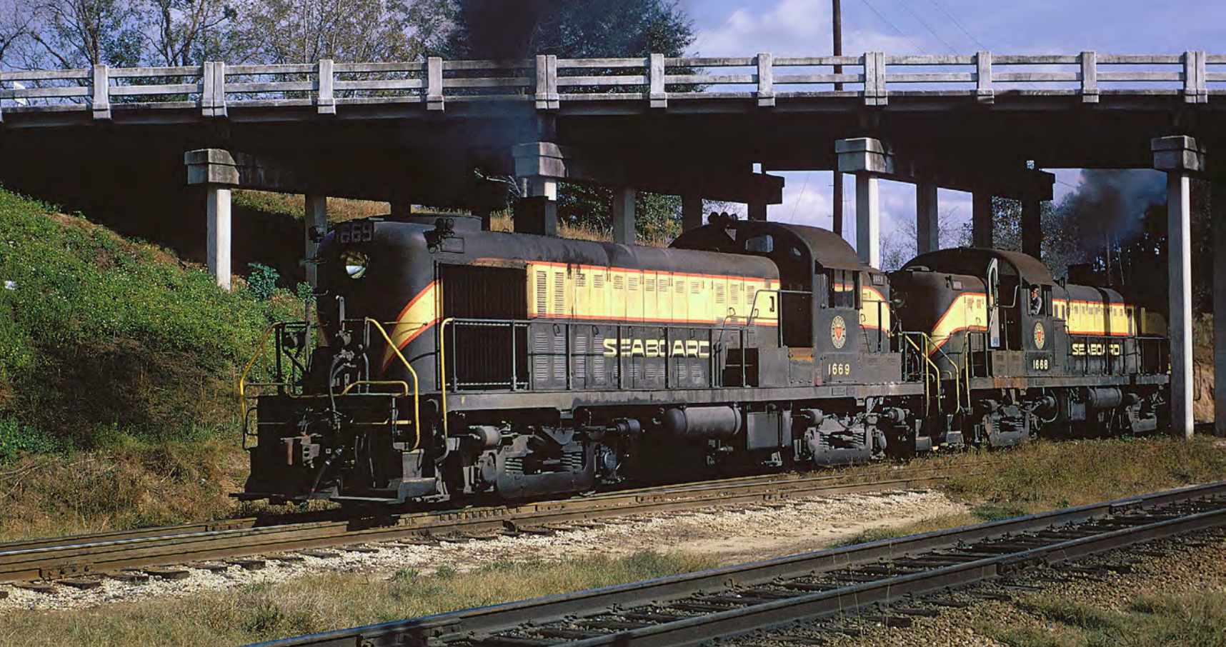
Alco built on its RS1 success with the 1,500-h.p. RS2 of 1946, then the 1,600-h.p. RS3 in '50. Sales figures reflect the rise of road-switcher popularity: 383 RS2's, 1,370 RS3's. Seaboard RS3's 1669 and 1668 work at Madison, Fla., in 1965. Harry L. Juday, J. David Ingles collection
