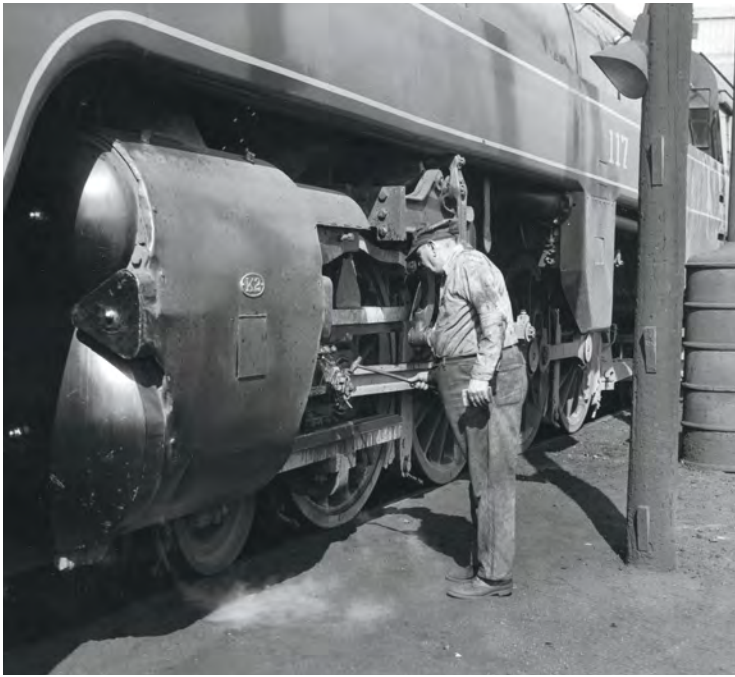
2:11 Next, two inspectors go over the engine, looking for any trouble that might have developed on the road.
