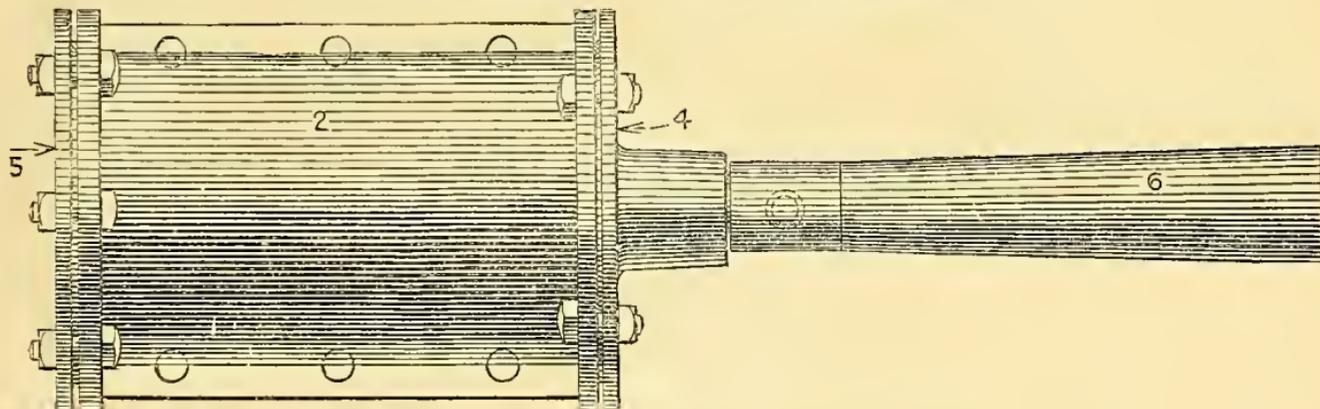
Fig. 727. BRAKE-CYLINDER, for Westinghouse Automatic Tender-brake.
