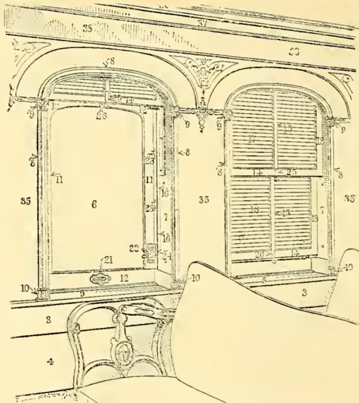
*Fig. 301. PERSPECTIVE VIEW OF PASSENGER-CAR WINDOWS.*
