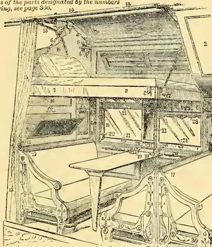
Fig. 298. PERSPECTIVE VIEW OF SECTION OF SLEEPING-CAR.
