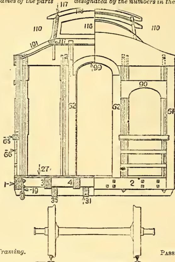
Fig. 224. End View, showing Framing.
