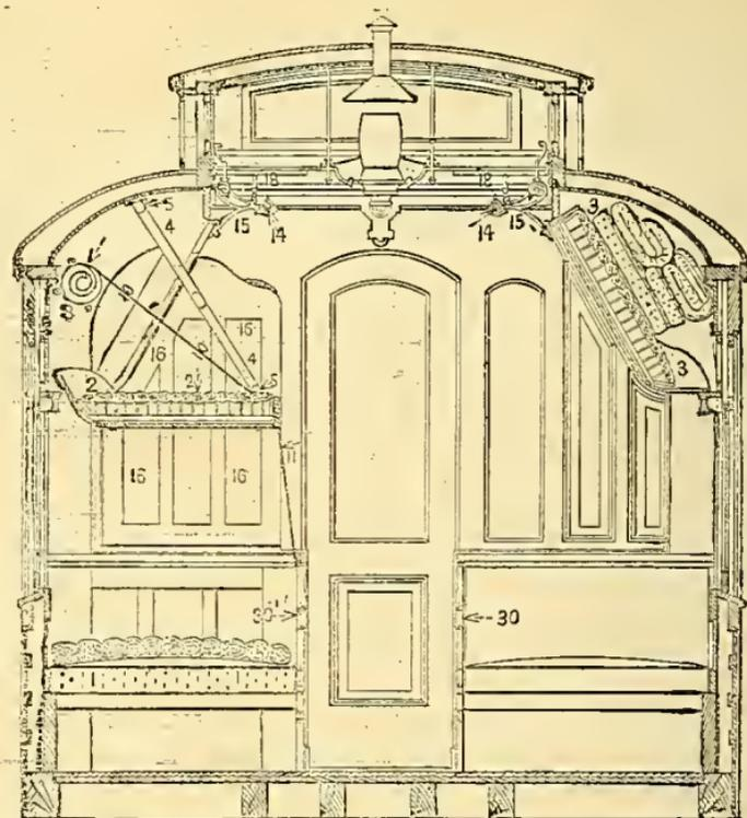
Berths Lowered. Fig. 297. Berths Raised.
