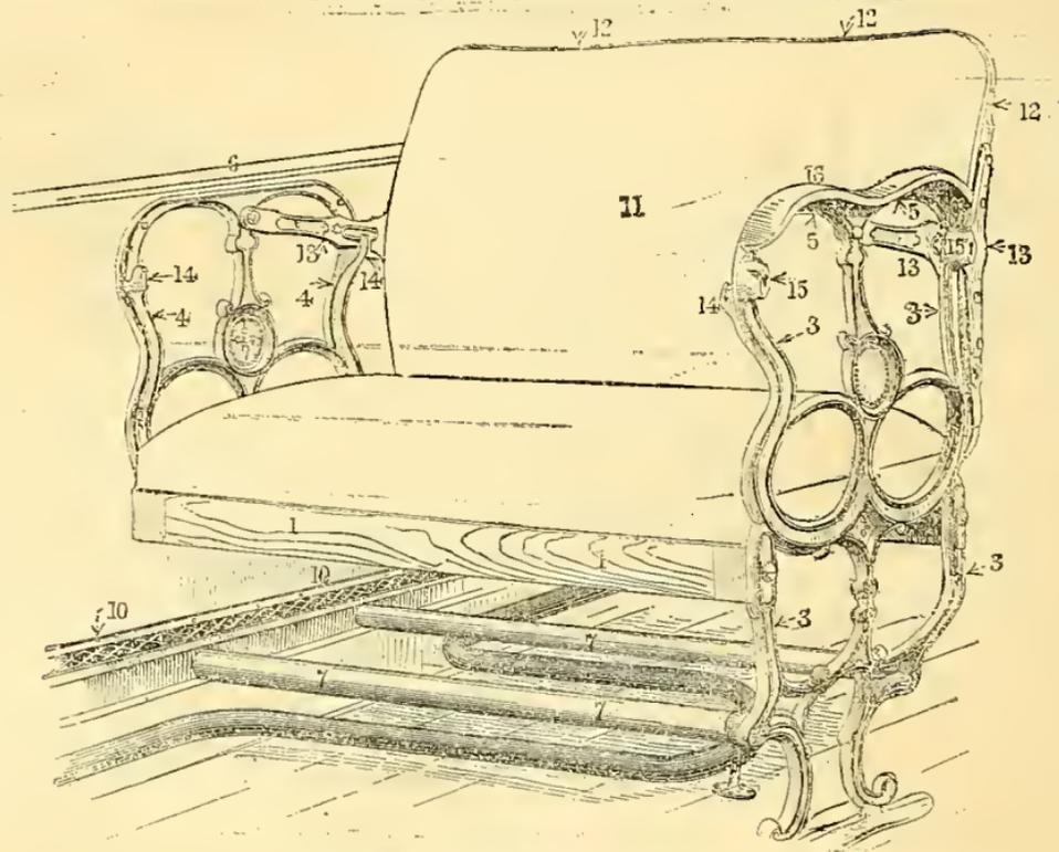
Fig. 401. CAR-SEAT, WITH IRON ENDS. Perspective View.
