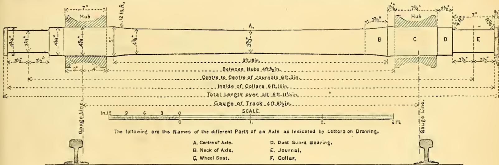
The engraving represents the dimensions of the axle when finished. Weight, finished, 347 lbs.
