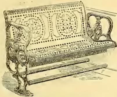
Fig. 402. PERFORATED-VENEER CAR-SEAT.
