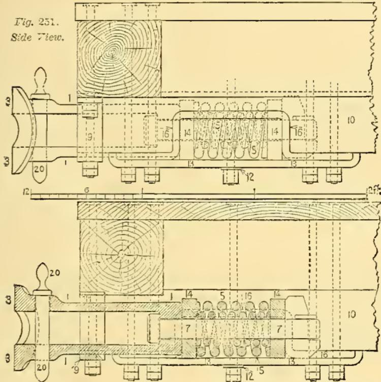
Fig. 252. Longitudinal Section. DRAW-GEAR FOR FREIGHT-CARS, PENNSYLVANIA RAILROAD.
