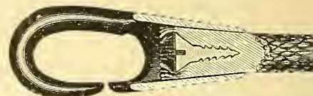
Fig. 710. BELL-CORD COUPLING.
