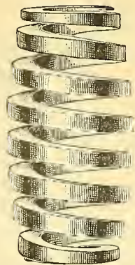
Fig. 2050. KEG-SHAPED SPIRAL-SPRING.
