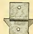
Fig. 1864. DECK-SASH PIVOT- PLATE.
