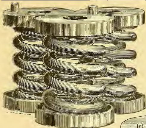
Fig. 2073. ROUND-BAR BOLSTER-SPRING (for 15-ton car.)
