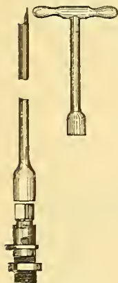
Fig. 1597. WATER-COOLER VALVE, with SOCKET and WRENCH. (1-5 full size.)
