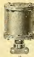
10 Fig. 308. (10.) STANDARD DRIVING-WHEEL BRAKE-CYLINDER. (See Fig. 314.)
