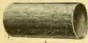
3 Fig. 302. (3.) AUXILIARY RESERVOIR (10 by 24 in.).
