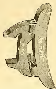
Fig. 1977. COMBINED BRAKE-SHOE AND HEAD. (Showing dovetail-joint and "Standard" split-key.)
