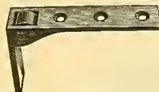
Fig. 1855. SLIDING-DOOR FRICTION- ROLLER.
