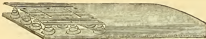
Fig. 1212. SPRING-EDGE SEAT-CUSHION, with SLATTED FLEXIBLE TOP and STEEL CROSS-PIECES.
