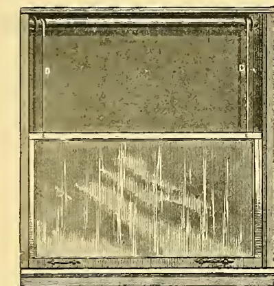
Fig. 1703. ORMSBY SASH-BALANCE (overhead style). (This drawing represents the principle of the device only and not its actual application.)
