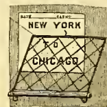
Fig. 1048. "PENFOLD" CARD-RACK for freight cars. (Attached to car-bodies as shown at 80, Fig. 93.)
