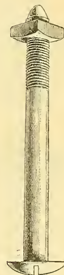
Fig. 1189. SEAT-JOINT BOLT. (For fastening seat-rail (1, Fig. 1122) to iron seat-ends. Also used at wall end.)
