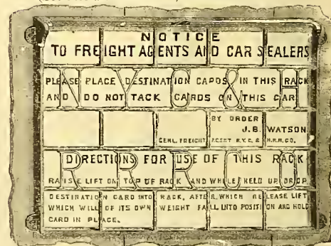
Fig. 1049. FREIGHT-CAR CARD-RACK. (Malleable iron), for carrying DESTINATION CARDS. (Usual sizes, inside measure, 5 1/2 x 6 1/2, 7 x 9, 9 x 12 inches. Attached to car-bodies as shown at 80, Fig. 93.)
