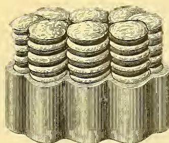
Fig. 2046. EIGHT-GROUP WOOL-PACKED SPIRAL-SPRING.
