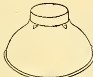
24 Fig. 1401. FIRE-CHAMBER (Top section).
