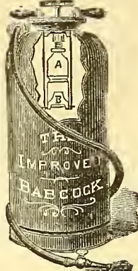
Fig. 1041. BABCOCK FIRE-EXTINGUISHER. A. Acid bottle. B. Acid-bottle Carrier. Bottle-breaking Head shown above A.
