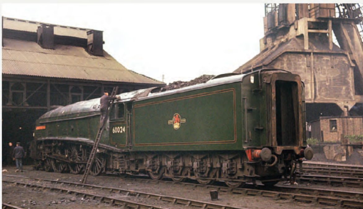
Kingfisher is a rare visitor to the Southern Region's Nine Elms shed in London. The corridor tender – complete with central gangway to allow changeover of crews mid-trip and which was essential to long-distance non-stop running – can clearly be seen. COLOUR-RAIL
