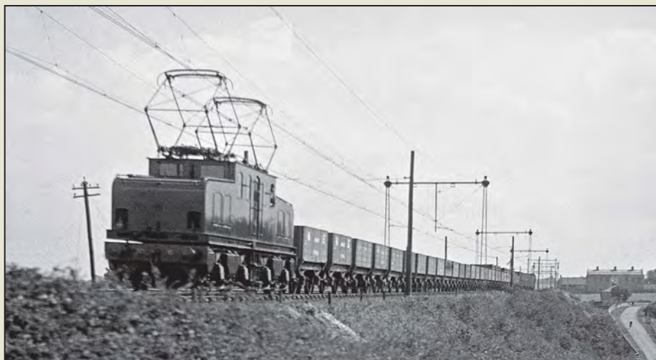
Left: North Eastern Railway electric freight loco No. 4, is seen leading a westbound empty mineral train near Aycliffe on 24 August 1923. 1,500V dc electric operation only lasted on this route from January 1916 until July 1935. NER No. 4, later became LNER No. 6491 and BR No. 26503.
