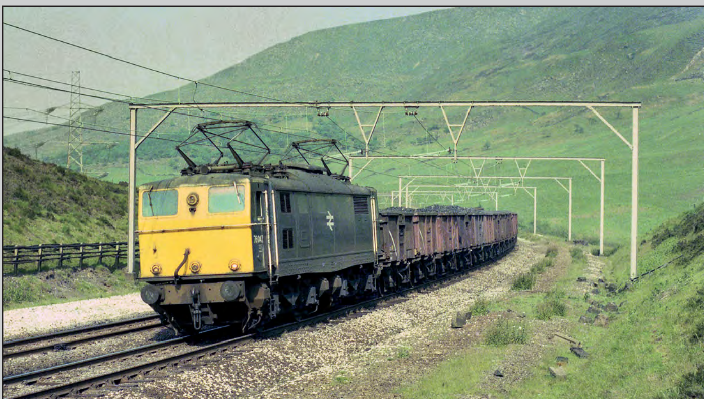
Below: Vacuum brake only No. 76047 approaches Torside on 23 June 1977 powering train 8M29, the 11.05 Mansfield to Garston loaded coal, formed of four-wheel wagons. This was another of the former passenger locos, once named Diomedes. www.rail-online.co.uk
