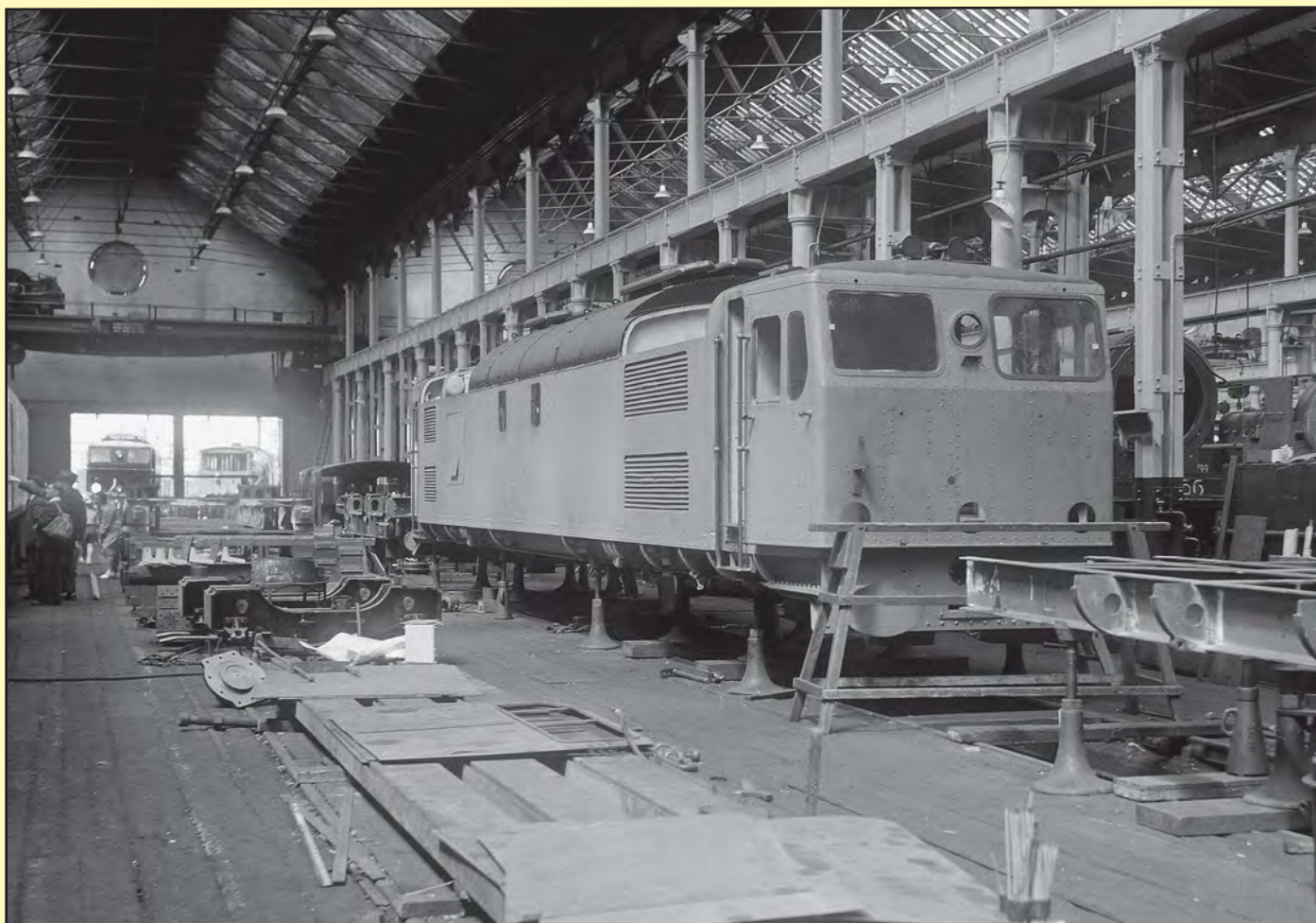
Above: The EM2 fleet were constructed at Gorton Works between mid 1953 and the end of 1954. Here No. 27001 is seen under advanced assembly, seen sharing works space with steam loco overhauls.
