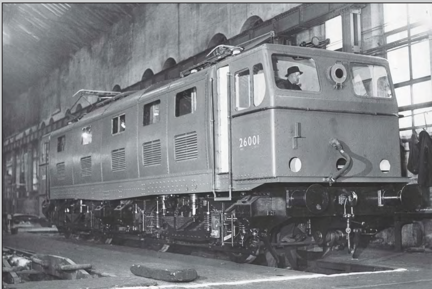
Below: The pioneer member of the production fleet, No. 26001 was taken to Dukinfield Works in mid-April 1950 for electrical work to be carried out, returning to Gorton some eight weeks later, when this image was recorded of the loco in the final assembly bay, but prior to painting. The locos first major outing was in October when it was hauled over the Woodhead route before being hauled south to Ilford where it could perform dynamic tests over the Shenfield line as well as brake performance trials on Brentwood bank. CJM-Collection
