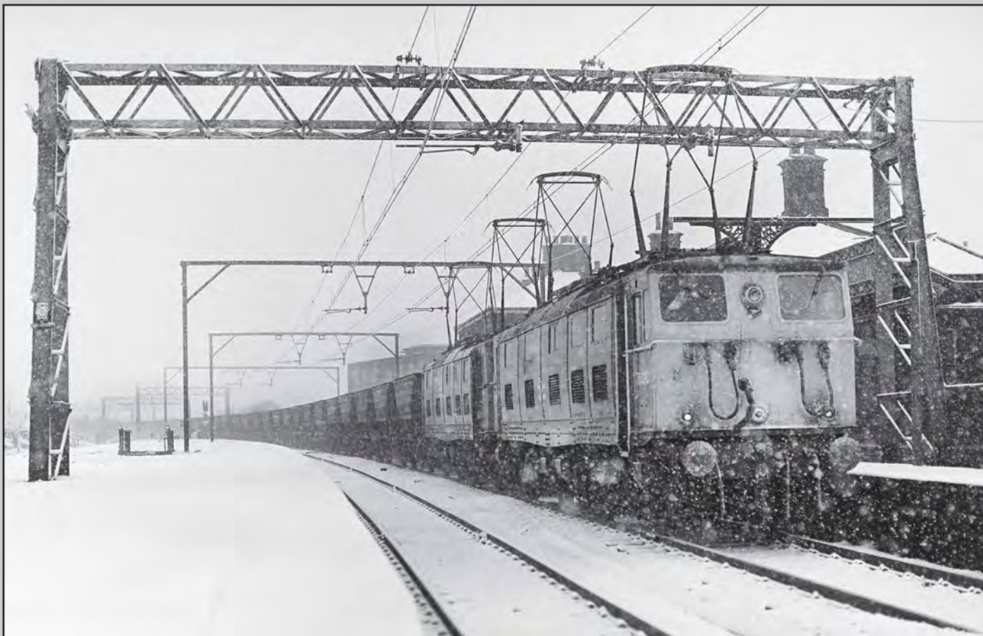
Above: The Manchester-Sheffield-Wath line, passing over the Pennines was almost guaranteed to have snow every winter, giving difficult operating conditions. However the 1,500V locos performed well with few failures caused by the ingress of snow. At just before 11.00 on the morning of 31 January 1980, multiple fitted Class 76s Nos. 76026 and 76010 pass through Penistone station at the head of a 36 vehicle MGR air braked coal train. CJM
