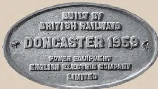
Above: Cast builders plate as fitted to the BR Southern Region HA class electric locos. These followed the standard design with the extra casting showing the power equipment supplier English Electric below. The plate shown is from loco No. 71011, the original E5011. CJM
