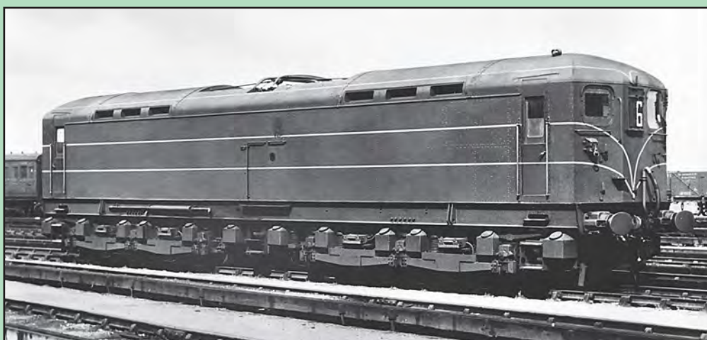
Above: The second of the Southern booster electric locomotives emerged from Ashford workshops in 1945, painted in Southern green livery and numbered CC2. Again the loco emerged with little publicity due to the ongoing war restrictions and issues. The loco was slightly different from the original example in not having a stencil headcode box on the front end, but sporting an additional marker light towards the upper bodywork. The loco is seen when very new with its pantograph in a raised position, viewed from its equipment or grilled body side. CJM-Collection
