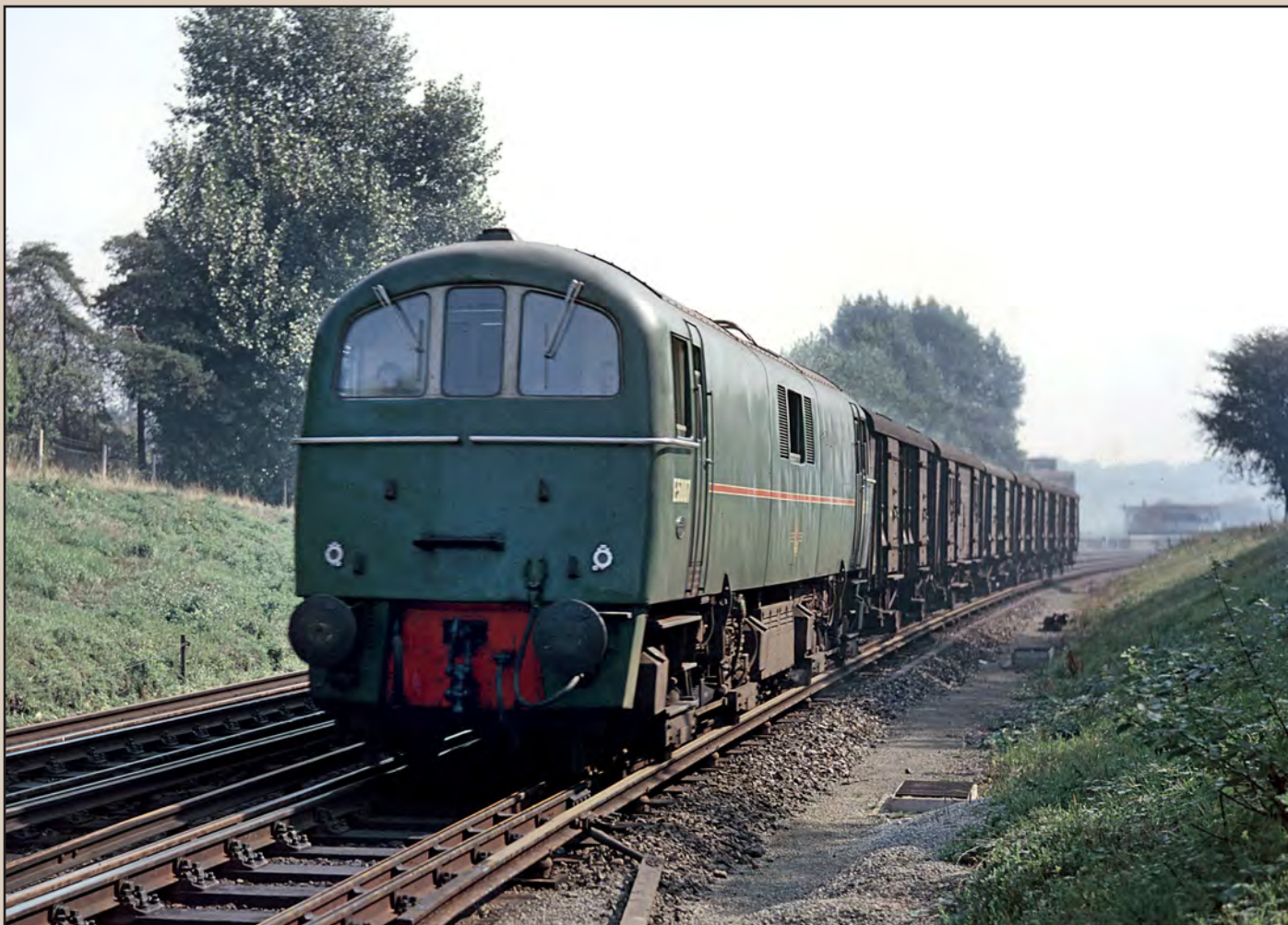
Above: With the equipment room drop-light window open to reduce heat, No. E5007 passes Shortlands Junction in spring 1960 with a short 4-wheel van train from Dover to Bricklayers Arms. Although often only associated with passenger services, the HA class booster electrics were frequently seen on Southern Eastern section freight and van services. CJM-Collection
