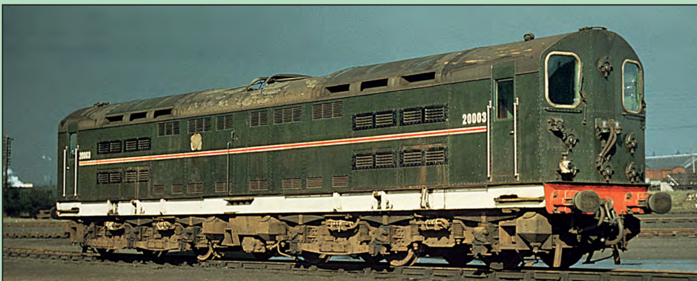
Below: Looking in rather poor external condition and devoid of any BR motif on the bodyside, No. 20003 stands at Eastleigh in May 1959. By the looks of the loco, the white sole bar had recently been applied. This loco was obviously awaiting attention at the nearby workshops as part of the power pickup equipment is missing from the near bogie and some of the high tension cables have been tied up. www.colour-rail.com
