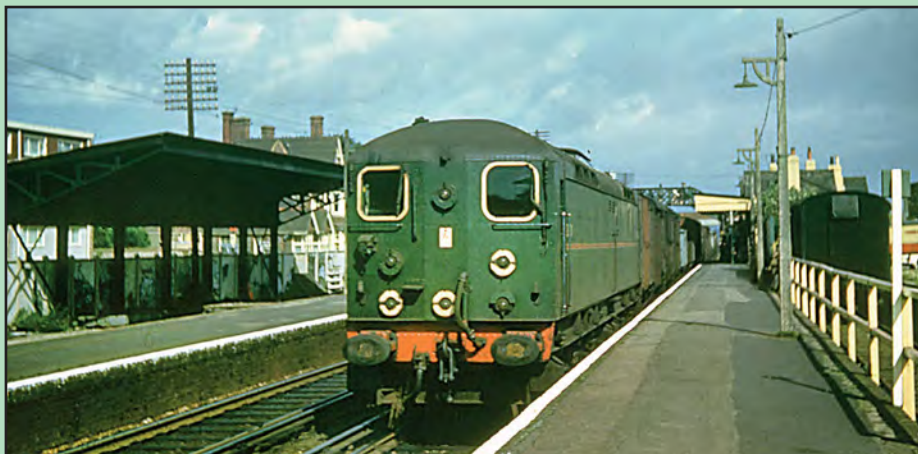
Right: In immaculate condition at Eastleigh Works in May 1959 following a classified overhaul, No. 20002 shows BR Southern green, with a red buffer beam and buffer shanks and a white sole bar. It is worth noting the varnished hardwood show beams, which did not stay in this condition for long once the loco was in daily service. Buffer beam connections on these locos was only basic with a coupling hook and shackle, a vacuum pipe mounted upward from the buffer beam and a steam heat pipe mounted downwards from the buffer beam. www.colour-rail.com / T Owen
