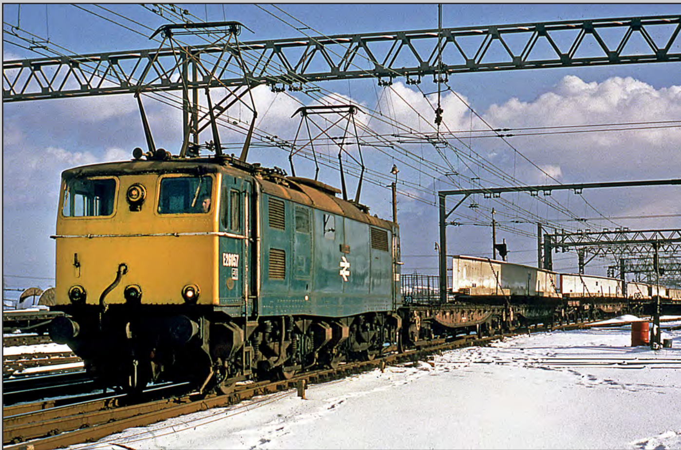
Above: One of the original passenger-equipped EM1s No. E26057 Ulysses, carrying standard rail blue livery but with its original number with an 'E' prefix and still sporting its cast nameplate as late as 1970, is seen passing Penistone at the head of a special freight transporting large steel girders, who's length span more than one wagon. After the passenger services ceased on the Manchester-Sheffield route, the passenger locos were used for normal freight operations. www.colour-rail.com / P. Hughes
