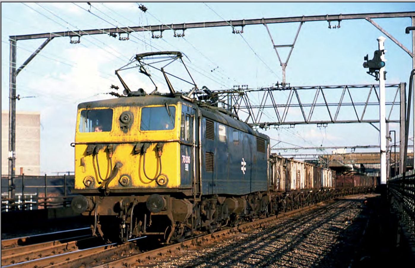
Below: Carrying its five-digit TOPS number, 76006 and full rail blue corporate livery, this dual brake fitted example, equipped with multiple control equipment passes through Sheffield Victoria in 1978 at the head of a long freight service. This loco was completed at the end of December 1950 and remained in traffic until July 1981, eventually being broken up by C F Booth of Rotherham in May 1983. www.colour-rail.com / P. Hughes
