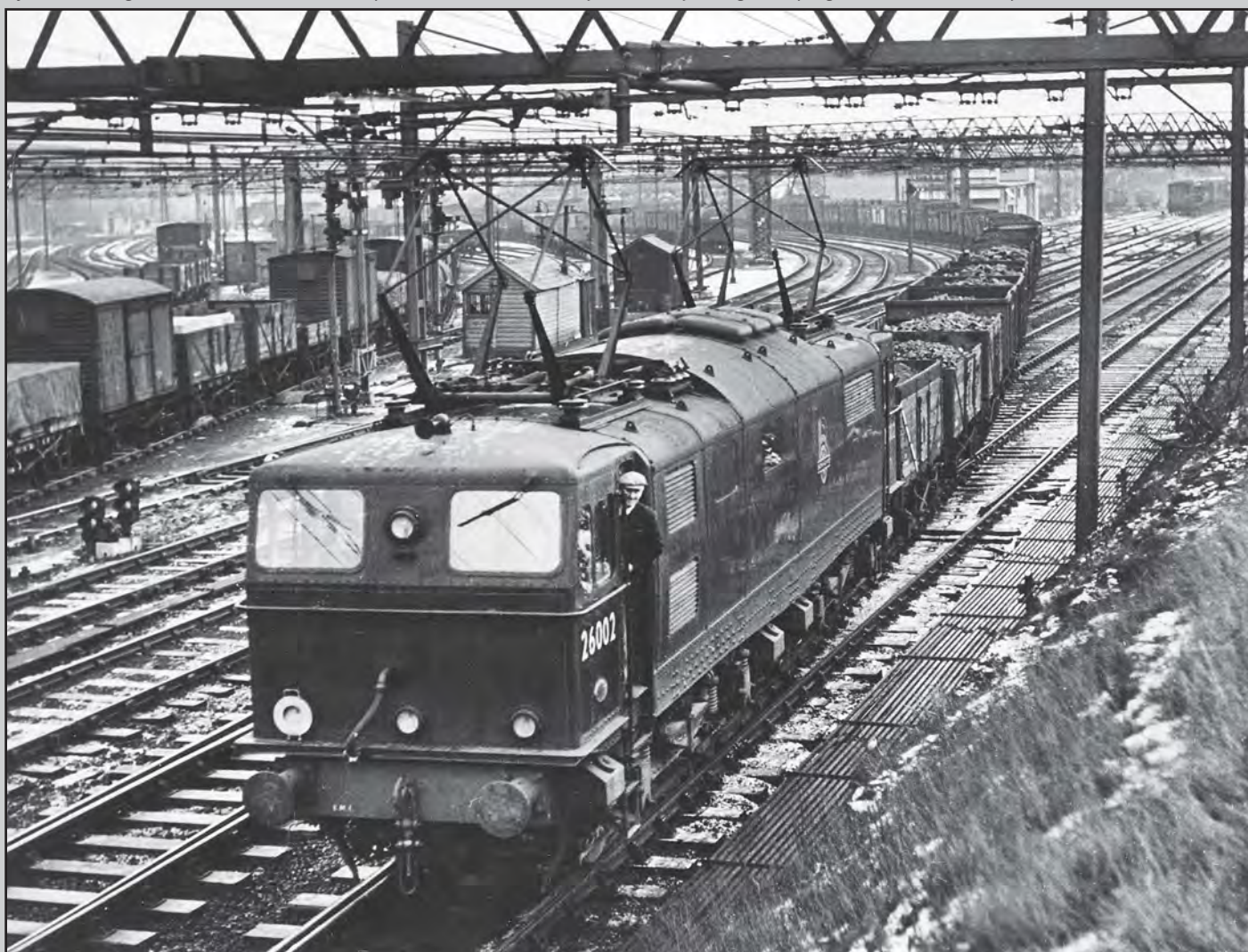
Below: In January 1952, soon after commencement of electric services, the second loco of the production design No. 26002 crosses Barnsley Junction, Penistone powering a long coal train, formed of wooden bodied four-wheel wagons. This locomotive was delivered to Wath in late 1951 after a period of dynamic testing in the London area based at Ilford, which saw the loco operate both passenger and freight consists in the Shenfield area. CJM-C
