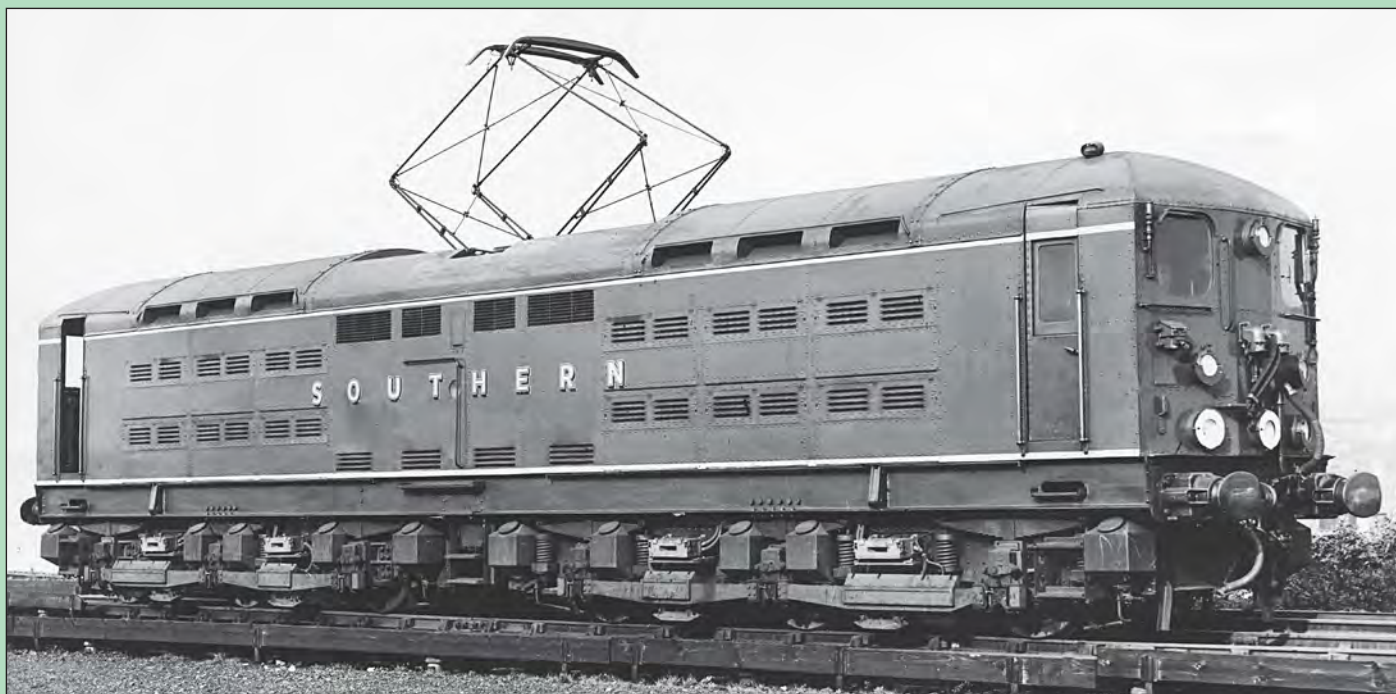
Above: The second of the Southern booster electric locomotives emerged from Ashford workshops in 1945, painted in Southern green livery and numbered CC2. Again the loco emerged with little publicity due to the ongoing war restrictions and issues. The loco was slightly different from the original example in not having a stencil headcode box on the front end, but sporting an additional marker light towards the upper bodywork. The loco is seen when very new with its pantograph in a raised position, viewed from its equipment or grilled body side. CJM-Collection
