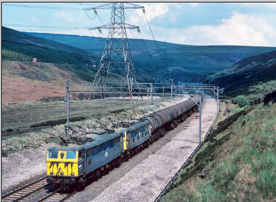
Left Top: As heavier air braked trains were introduced over the Woodhead route, so the use of double headed Class 76s increased, using the locos multiple control facilities. On 9 June 1977, Nos. 76028 and 76027 approach Woodhead with a westbound oil train formed of bogie vehicles. Tom Heavyside
