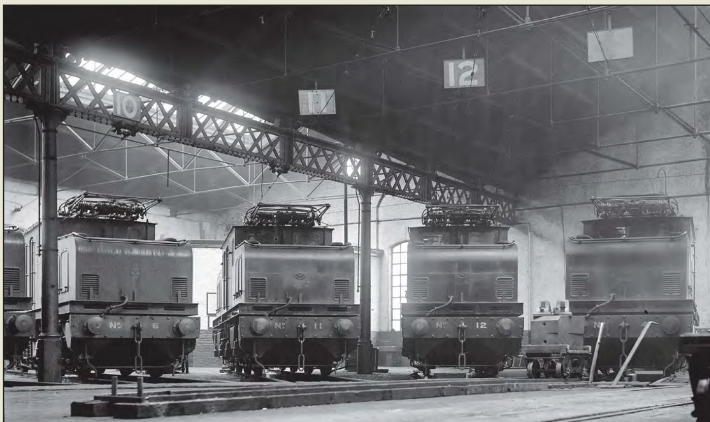
Below: The number three roundhouse at Shildon was adapted to house and maintain the 10 North Eastern Electric locos. In this picture recorded on 21 May 1932, when the electrified system was still in full use, shows Nos. 6, 11, 12 and 4 stabled between duties in the stalls, with a fifth loco on the far left side.
