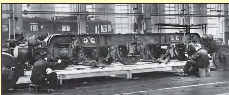
Below: Class EM2 bogie under overhaul at Gorton Works. CJM-Collection
