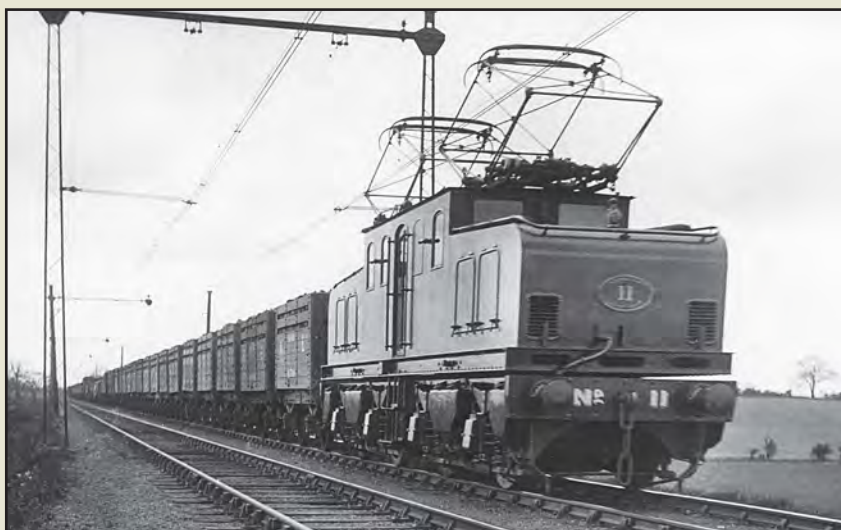
Above: The first of the Newport-Shildon 1,500V dc electric locomotives No. NER3 is seen posed in the yard at Darlington Works on 11 May 1914, painted in workshop grey, but lined and branded. The two pantographs have been raised for the photograph, but of course no overhead power equipment was to be found at the works. CJM-C
