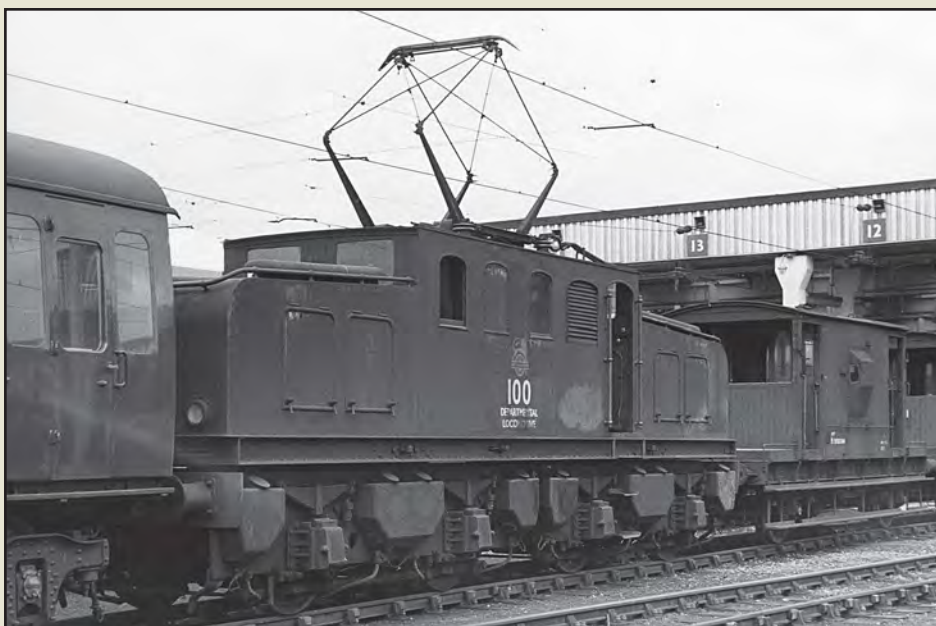
Above, Left and Below Left: The rebuilding work for NER No. 11 was authorised in 1936 and soon after it was transferred from Darlington to Doncaster for a major strip and rebuild. Revised traction equipment was installed as was a totally revised driving cab with new controls. From the outside the most noticeable difference was the moving of the cab door from the central position to the right end on both sides, as well as the obvious changes to the power collection, now using a single pantograph. Output horsepower was increased to 1,256hp with a corresponding increase in tractive effort to 37,000lb. The official release date in its new guise was 13 October 1944. Due to World War 2 and the stopping of the Woodhead electrification, 6498 was stored and eventually moved to South Gosforth. The loco, renumbered as 26510 was then transferred south to Ilford on 24 August 1949, where it became the depot pilot, becoming Departmental 100 in 1959. In the above view No. LNER26510 is seen at Shenfield while undertaking testing. In the middle view the loco is seen marshalled with a Shenfield electric at Ilford depot, while in the lower image, it carried the identity of Departmental 100 outside the servicing shed at Ilford. All: CJM-Collection
