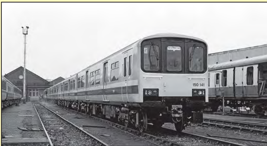
Above: Following the November 1984 order for the follow-on Class 150/1 stock delivery was rapid. In this view taken on 27 September 1985, set No. 150106 is seen in York Works Yard as a complete structure but prior to fitting out. No handrails are fitted, the cab doors are not fitted and the battery box is open. This set was delivered to Derby shed a month later. Colin Burnham
