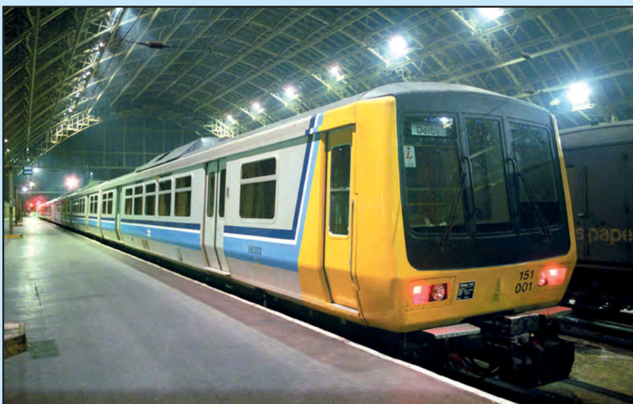
Left Below: After both the Class 150 and 151 Prototype sets were given the green light for main line normal speed operation, a number of special nighttime paths were organised between Derby and London St Pancras for mileage accumulation and high speed dynamic testing to be undertaken. Some of these test runs were undertaken alone, others in pairs and some with a Class 150 and a 151 working together. This view in early 1986 shows Class 151 No. 151001 and Class 150001 under the great Barlow roof at London St Pancras. This picture is in the position of where the Eurostar platforms are today.
