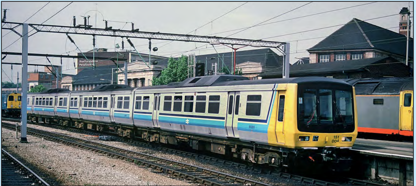
Above: Externally the Class 151 was left in raw aluminium, with painted yellow ends and a two-tone blue and white body side band. The raw aluminium extended to the roof and roof pod. The underframe was finished in black. These were some of the first units to have a contrasting colour or livery difference on the passenger doors, which omitted the mid-height banding. On 28 June 1988, set No. 151004 (renumbered from 151002) arrives at Stoke-on-Trent with the 14.38 Crewe to Derby service.
