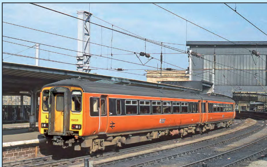
Above: The final 14 Class 156s were outshopped from Metro-Cammell painted in Strathclyde Passenger Transport Executive orange and black livery. These sets were funded by the PTE to operate on Glasgow non-electrified services in an attempt to replace the worst of the first generation DMMU sets. On 21 August 1992, set No. 156507 departs from Glasgow Central with an afternoon service bound for East Kilbride. CJM
