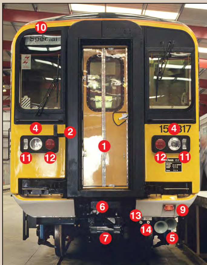
Above: Class 153 front end layout. The 'new' or small cab end is shown on the left. The cab on the right has received subsequent modification in terms of valance, marker lights and obstacle deflector plate. 1: Gangway door, 2: Lamp bracket, 3: Joint LED red tail and white marker light, 4: Headlight, 5: Warning horns, 6: BSI coupling, 7: Electrical connection box, 8: Obstacle deflector plate, 9: Emergency jumper cable, 10: Destination indicator, 11: Marker light, 12: Tail light, 13: Emergency air supply, 14: Emergency coupling air supply. Both: CJM
