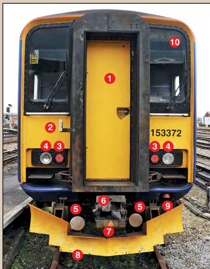
Above: Class 153 front end layout. The 'new' or small cab end is shown on the left. The cab on the right has received subsequent modification in terms of valance, marker lights and obstacle deflector plate. 1: Gangway door, 2: Lamp bracket, 3: Joint LED red tail and white marker light, 4: Headlight, 5: Warning horns, 6: BSI coupling, 7: Electrical connection box, 8: Obstacle deflector plate, 9: Emergency jumper cable, 10: Destination indicator, 11: Marker light, 12: Tail light, 13: Emergency air supply, 14: Emergency coupling air supply. Both: CJM
