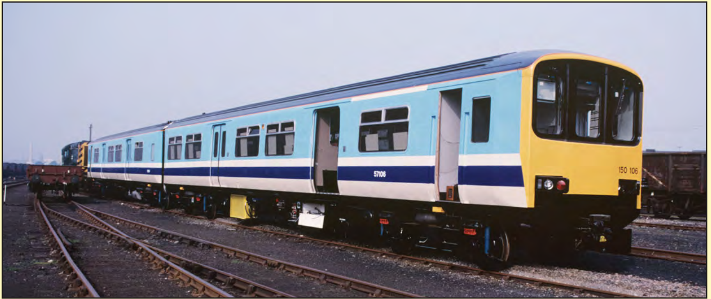
Above: Following the November 1984 order for the follow-on Class 150/1 stock delivery was rapid. In this view taken on 27 September 1985, set No. 150106 is seen in York Works Yard as a complete structure but prior to fitting out. No handrails are fitted, the cab doors are not fitted and the battery box is open. This set was delivered to Derby shed a month later. Colin Burnham
