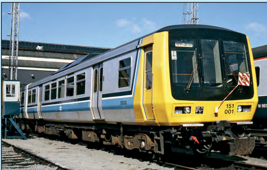
Above: Externally the Class 151 was left in raw aluminium, with painted yellow ends and a two-tone blue and white body side band. The raw aluminium extended to the roof and roof pod. The underframe was finished in black. These were some of the first units to have a contrasting colour or livery difference on the passenger doors, which omitted the mid-height banding. On 28 June 1988, set No. 151004 (renumbered from 151002) arrives at Stoke-on-Trent with the 14.38 Crewe to Derby service.
