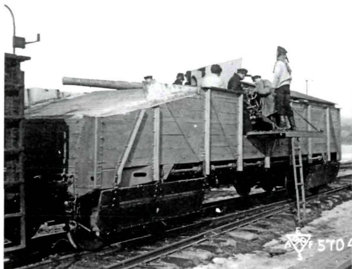
Armored trains formed by sailors were a common feature of both Red and White forces in the Russian Civil War. Their ships provided a handy source of deck guns that could easily be mounted on flatcars, as seen here on a White Russian armored train of the Army of Siberia in January 1920, built in the Vladivostok naval yard. (NARA)
