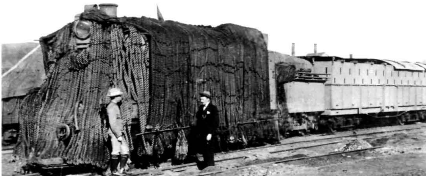
One of the more curious innovations during the Boer War was the use of protective carpets made of heavy rope to protect the locomotive from small-arms fire, resulting in the "Hairy Mary" seen here. (Australian War Memorial P01328.012)
