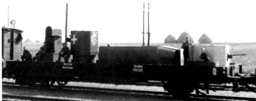
German armored trains in 1939 were primitive compared to their Polish counterparts. This is the artillery car of PZ 4, armed with a 37mm gun in the lower turret and a 75mm IG 18 infantry gun in the upper turret. (MHI)
