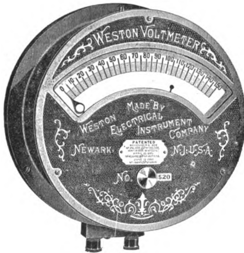
FIG. 336.—WESTON VOLTMETER. immediately without any swing. To find the difference
