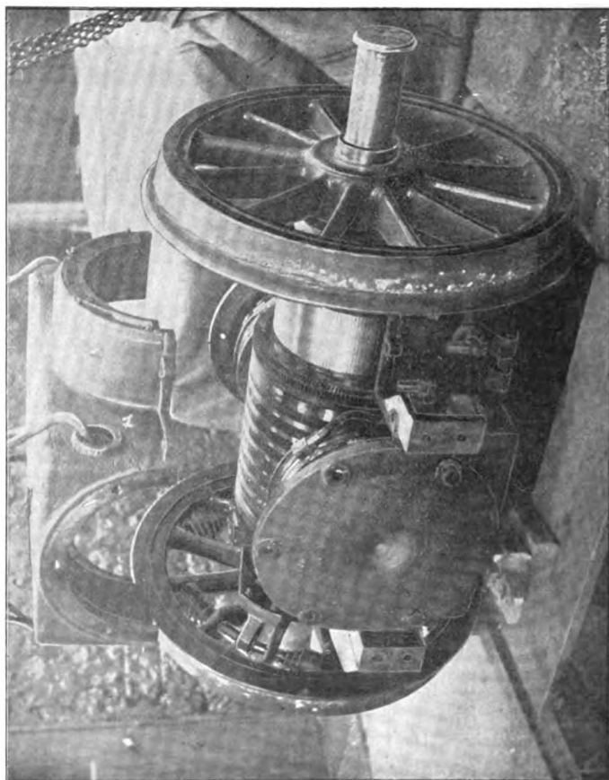
FIG. 368.—HEILMANN ELECTRIC LOCOMOTIVE. View showing the Upper Half of Field-yoke removed, exposing to view the Poles, Armature, and Commutator of Motor.
