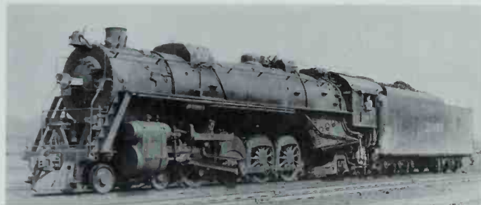
The 2600-class engines were IC's finest 4-8-2s. They were built by the road's shops at Paducah, Kentucky, in 1942 and 1943. The web-spoke drivers were uncommon; the absence of an air tank under the running board is accounted for by a reservoir cast integral with the frame.
