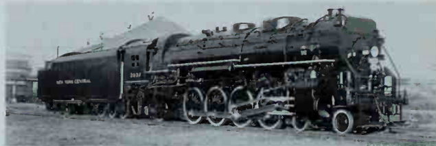
New York Central L-3-b 3037, built by Lima in 1940, was built as a freight locomotive, but NYC eventually discovered its modern 4-8-2s were equally good in passenger service. Lima photo; collection of P. E. Percy.
