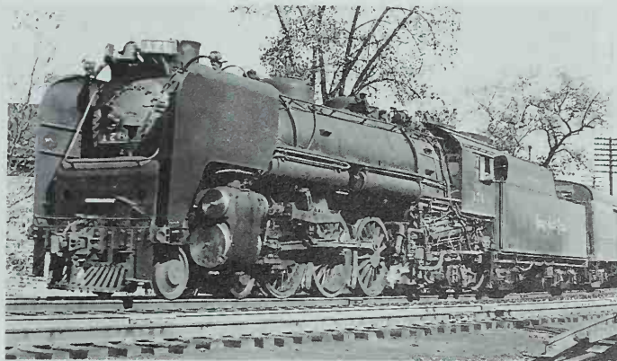
Nickel Plate's Hudsons looked bigger than they were after the smoke lifters were added. In actuality they were little more than a USRA light Pacific with a four-wheel trailing truck. Photo by Robert Hally.
