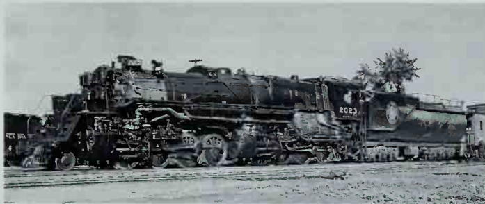
The need for a wide firebox over 63" drivers made the 2-8-8-0s Great Northern's tallest engines. Photo by Russell D. Porter.
