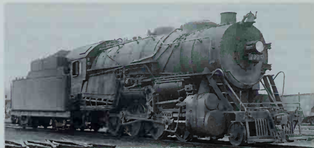
The heaviest nonexperimental Consolidations were Reading's I-10sa class, built by Baldwin between 1921 and 1923. They tipped the scales at 322,690 pounds. Reading 2008, photographed at Rutherford, Pennsylvania, in 1948, shows that the Wootten firebox was just about as wide as Reading's clearances allowed. Photo by A. D. Hooks.
