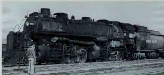
UP's standard road freight power for a decade was the 2-8-8-0. In the late 1930s and early 1940s UP converted them to single-expansion engines and renumbered them in the 3500 series. Photo by J. F. Orem.
