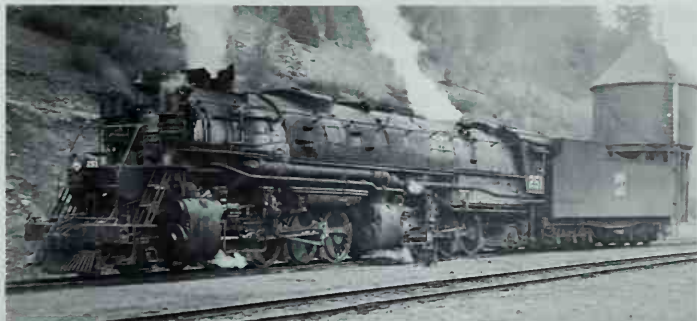
The 2-8-8-2s were large, modern articulateds. Number 251 was the first of the 1931 batch. The second group, built in 1938, had disc drivers and welded tenders. Photo by Ed W. Bewley.
