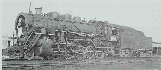
Gulf, Mobile & Ohio 261, photographed in 1941, shows off more than a decade of modifications to the original design, among them a Coffin feedwater heater mounted on the front of the smokebox, a second sand dome, and a large single-phase air pump replacing one of the original pair. Photo by Bernard Corbin.
