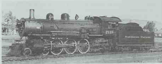
Compared with Q-class No. 2080, shown on page 35, Q-1 Pacific No. 2119 illustrates the early development of the type, with a larger boiler and outside-frame trailing truck. By 1945 more than half the class, built between 1904 and 1907, had been retired. Photo by R. V. Nixon.
