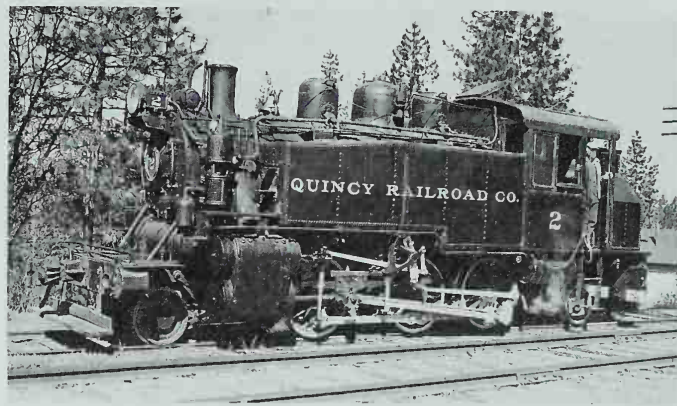
Quincy Railroad 2, an Alco product of 1924, carried enough water in the side tanks and fuel oil in the rear tank for the 6-mile run between Quincy, California, and the connection with the Western Pacific at Quincy Junction. Photo by Guy L. Dunscomb.
