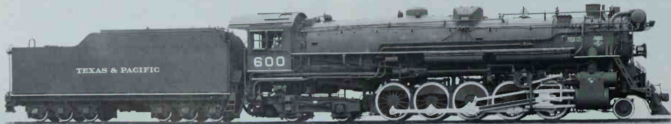
Texas & Pacific No. 600 was the first 2-10-4. It was a development of Lima's A-1, and had the same short frame and articulated trailing truck. The empty space above the trailing truck would be occupied by an ashpan on a coal-burning engine. Lima photo.
