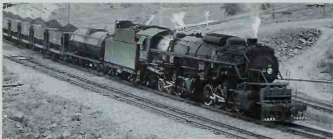
Mallet 211 was one of five rebuilt from compounds to simple engines. Forward and rear cylinders the same size is the clue. Photo by Frank A. King.
