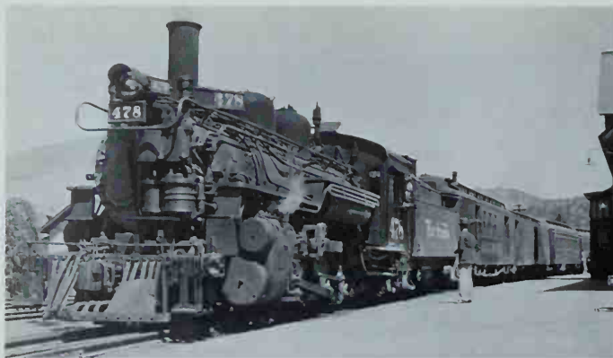
The K-28 "Sports Model" narrow gauge Mikados carried their air pumps on the smokebox fronts. They were best known for hauling the San Juan , the last named narrow gauge passenger train in the U. S., between Alamosa and Durango, Colorado. Photo by Kent Day Coes.
