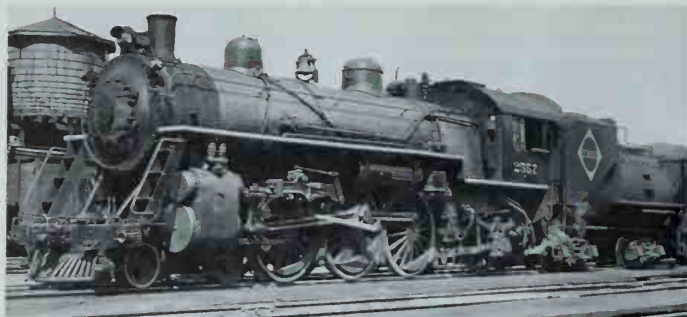
The K-1 Pacifics were built with inside valves and Stephenson valve gear; No. 2557 shows how they looked after rebuilding with outside valves and Baker gear. Photo by H. W. Pontin.
