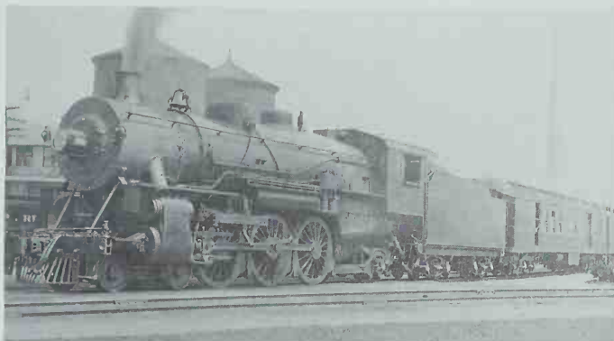
BR&P 616, shown at East Salamanca, New York, was the highest-numbered of the WW class of Pacifics. The piston-rod extensions and the undersized trailing truck frame are interesting features. Trains Collection.
