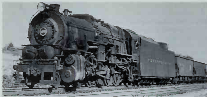
The H11 Decapods were the equivalent of two H8 Consolidations on coal and ore trains. Large as they were, they were outweighed by the 2-10-0s of Lehigh & New England. Photo by Richard J. Cook.
