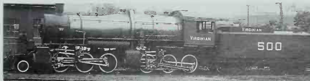
Virginian 500 was the first 2-6-6-0 built. It was one of four, which were followed by eight larger 2-6-6-0s, then Virginian turned to eight- and ten-coupled power and electric locomotives. Richmond Works photo.
