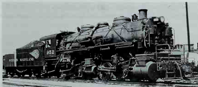
Western Maryland's nine 0-6-6-0s were built as 2-6-6-2s in 1909 and 1910. With the arrival of large 2-10-0s, the articulateds were stripped of their lead and trailing trucks and put to work as heavy switchers. Photo by Leslie R. Ross.
