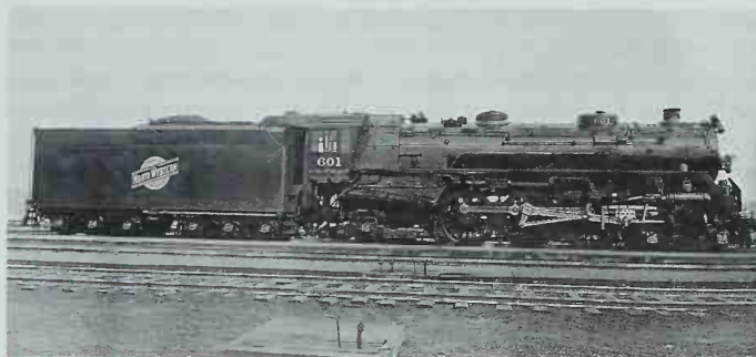
Omaha Road's E-3 Pacifics were built a year after the class H Northern and have some of the same details, such as outside-journal lead truck and slant-front cab. C&NW photo.
