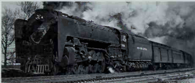
Niagara 6001, first of the production 4-8-4s, wheels the Iroquois west through Berea, Ohio, during its first winter of service. With their high headlights and smoke lifters the Niagaras brought a new look to the New York Central. Photo by Richard J. Cook.
