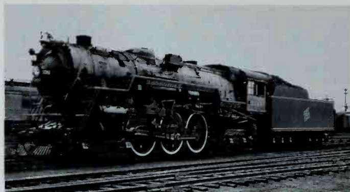
Milwaukee's racy F6 4-6-4s were a major step forward from the Pacifics. They had outside-journal lead trucks, cast trailing trucks, and large tenders — but between the Pacifics and the Hudsons the railroad had lavished its resources on electric locomotives. Milwaukee Road photo.
