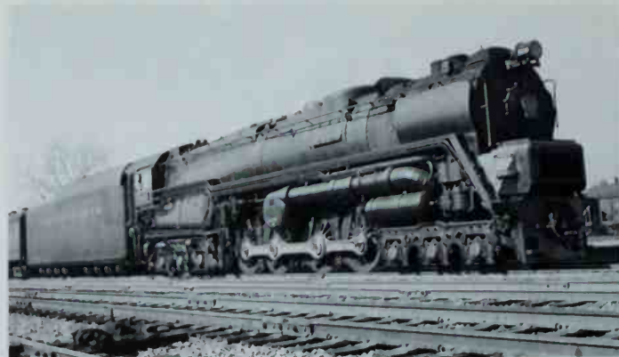
Chesapeake & Ohio orange-and-silver steam turbine-electric No. 500 was an enormous piece of equipment, 20 feet longer than today's auto-racks and piggyback flats, and its tender was about the size of today's covered hopper cars. Baldwin photo.
