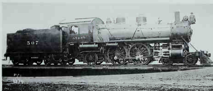
Santa Fe 507 is a balanced compound. The high-pressure cylinders are inside the frames; rods from those cylinders are connected to cranks on the first axle. All four cylinders drive on the first axle. The eccentrics for the Stephenson valve gear are on the second driving axle. Note the minimal counterweight on the first driver and its position. Collection of Frederick Westing.
