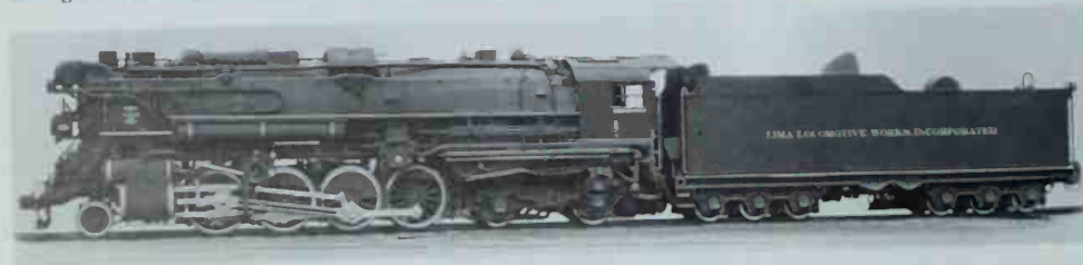
Lima Locomotive Works 1 — the A-1 — was the first Berkshire and the first locomotive with a firebox large enough to require a four-wheel trailing truck. The piping for the booster engine on the trailing truck, the piping for the Elesco feed-water heater, and the outside dry pipe leading from the steam dome to the front-end throttle all contributed to the appearance of power. Lima photo.
