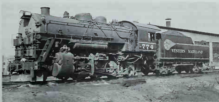
The H-8-class Consolidations had switcher-size drivers, 52", for use on steep branches out of Elkins, West Virginia. Photo by Russell L. Wilcox.
