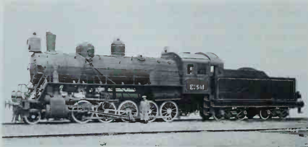
Number 541, built by Baldwin in 1917, was one of the group shipped to Russia. Characteristic Russian details include the elaborate railings along the running board, dual headlights on the pilot beam, buffers and screw couplings, and the hood over the front of the tender. BLW photo, collection of H. L. Broadbelt.
