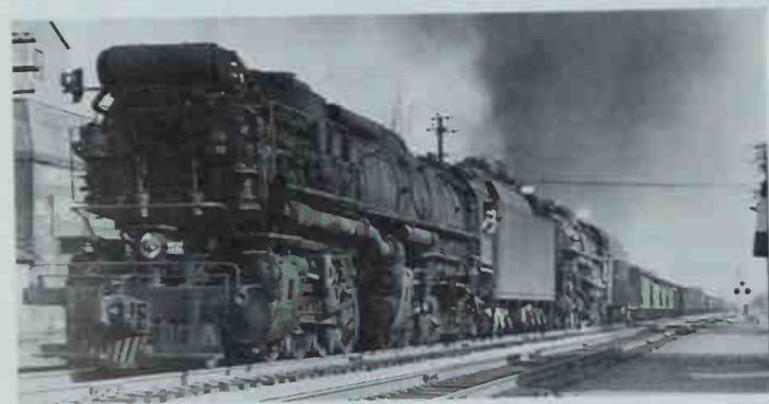
Chesapeake & Ohio's 2-8-8-2s were the first nonexperimental simple articulateds. Number 1541 and 2-10-4 3016 lead a long coal train north through Linworth, Ohio. The number of appliances and the amount of piping on 1541 borders on the incredible. Photo by Richard E. Dill.
