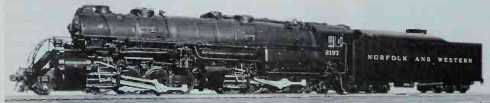
Norfolk & Western Y6b 2197, built in 1952 and scrapped in 1959, represents the ultimate development of the compound articulated with efficiency features like a feedwater heater and roller bearings all around. N&W photo.
