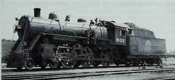
The E-7-class Ten-Wheelers were obviously passenger engines with their 73" drivers. Disk drivers such as No. 507 received during a visit to Oelwein shops were rare on small locomotives, particularly in full sets. Photo by Henry J. McCord.
