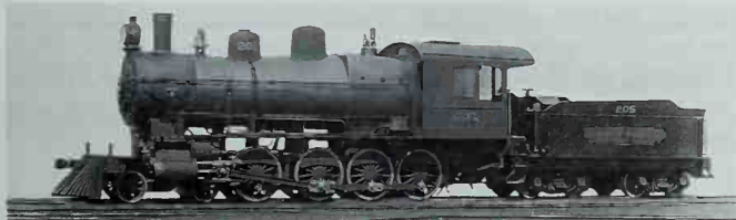
Twelve-Wheeler 205 was built by Brooks in 1899. Its inboard valves and narrow Belpaire firebox are typical of Brooks locomotives of the time. It was renumbered 225 in 1911 and rebuilt in 1926 with outboard piston valves, Walschaerts valve gear, a wide radial-stay firebox above the drivers, and an extended smokebox. 205, Alco Historic Photos; 225, collection of Harold K. Vollrath.
