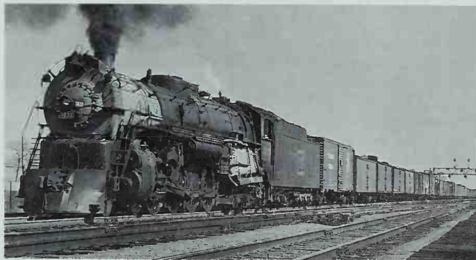
Burlington built O-5A 5633, a handsome 4-8-4, in its West Burlington, Iowa, shops in 1940. With its solid pilot and vestibule cab, it represents the ultimate development of steam freight power on the road. Here one is leading a westbound freight at Eola, Illinois, in 1949. Photo by Henry J. McCord.
