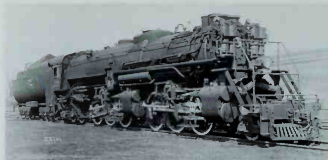
Drivers 69" in diameter make Seaboard 2501 a racy-looking engine. It has an Elesco coil-type feedwater heater and a semi-Vanderbilt tender. Baldwin photo, collection of H. L. Broadbelt.
