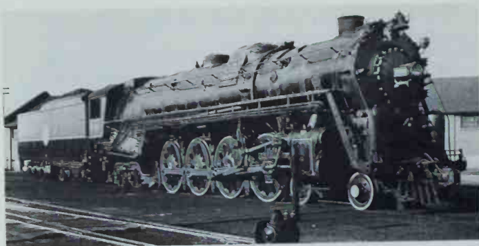
The ultimate development of dual-service power on the Atlantic Coast Line was the R-1-class 4-8-4, built by Baldwin in 1938. In appearance the R-1s were very much the modern Baldwin locomotive.
