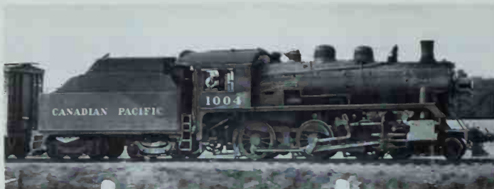
Between 1881 and 1949 Canadian Pacific acquired 3,257 steam locomotives, 502 of which were D-10 Ten-Wheelers like No. 1004, which is shown leading a freight at Wroxeter, Ontario, in July 1957. Photo by Don Wood.
