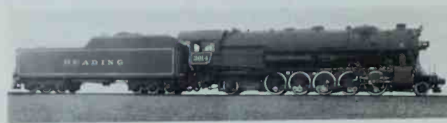
Reading 3014 and the other members of the K1sb class were the heaviest 2-10-2s built. The Hodges trailing truck appears dwarfed by the Wooten firebox, but was adequate to carry its 57,000 pound load. Broadbelt collection.
