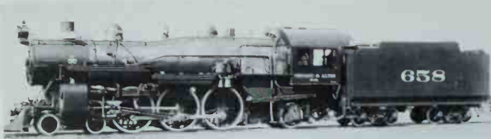
Harriman characteristics of Chicago & Alton 4-6-2 658 include the extended smokebox, deeply arched cab roof, and a tapered boiler course between the steam dome and the sand dome. Alco photo.
