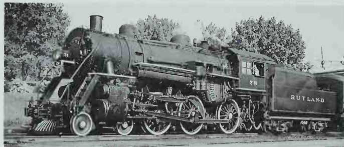
The 1912 Ten-Wheelers were relatively modern, with superheaters, piston valves, and Walschaerts gear, and remained in service until dieselization. Photo by L. B. Herrin.
