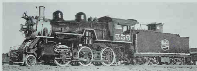
Missouri-Kansas-Texas found the 2-6-0 ideal for light freight service on light rail. Number 555, photographed at Altus, Oklahoma, in April 1946, is not only a modern-looking Mogul (especially for one built in 1904) but also a well-maintained one. Photo by Preston George.
