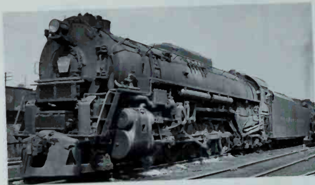
In 1942 the Pennsylvania Railroad was caught between an immediate need for heavy freight locomotives and a ten-drivered duplex that needed more drawing-board work. PRR copied Chesapeake & Ohio's 12-year-old T-1 for the 125 members of the J1 class, which many consider Pennsy's best modern engines. Photo by Don Wood.
