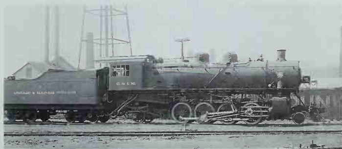
C&IM 23 (later 523), class E-2, was built by Alco's Brooks Works in 1918. Its 51" drivers suited it well for coal-mine switching and short hauls of heavy trains. Note the Southern valve gear. Alco photo.
