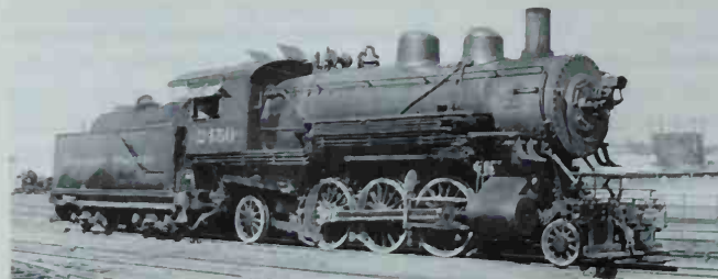
The Prairie developed first as a middleweight, medium-speed freight engine. Northern Pacific 2450, built by Alco in 1907, illustrates the characteristics: main rod connected to rear drivers, firebox behind rear drivers, and inboard piston valves (typical of the era in which most Prairies were built). Photo by R. V. Nixon.
