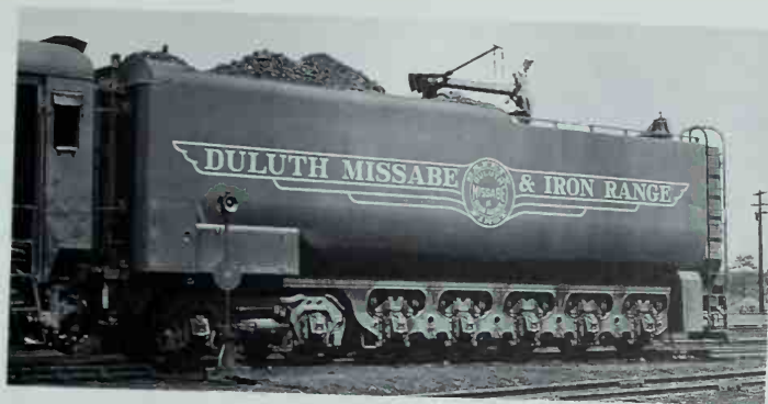
The pedestal tender, with a four-wheel lead truck and a ten-wheel rigid frame, was introduced in the late 1930s. The all-welded tender of DM&IR 225 carries a bell for backup moves. Photo by Bruce R. Meyer.
