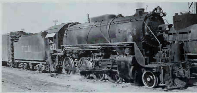
Consolidation 211, the first of 10 built by Baldwin in 1946, was obviously derived from the U. S. Army's 2-8-0 of World War II. Photo by C. W. Witbeck.
