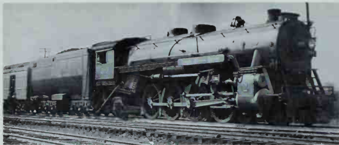
Mountain 263, at Richmond in 1938 on the northbound Orange Blossom Special , typifies the modernized M-2, with Elesco coil-type feedwater heater and 12-wheel tender. Photo by Bruce D. Fales.
