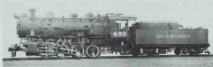
The C-2a class was the ultimate development of T&P's switcher fleet, with tender booster, front-end throttle (under the dome in front of the stack), and an outside pipe carrying superheated steam to the turret for the auxiliaries. Baldwin photo; collection of H. L. Broadbelt.
