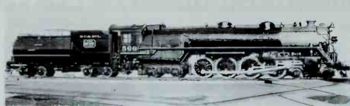
NC's J2-class 4-8-4s were among the lightest of the type, weighing 381,000 pounds as built. Only the J2s, the "Giders," had outside lead truck journals. Alco photo.
