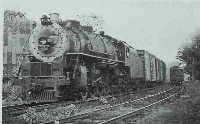
Rutland 93 was the last of the four Mountains. They were built by Alco in 1946, the last 4-8-2s built by a commercial builder in North America. Photo by S. K. Bolton Jr.
