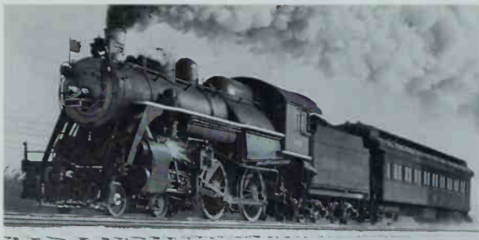
American 938 speeds west across the Jersey Meadows with a single coach in tow in November 1938 — white flags on the smokebox indicate the train is an extra, not a regularly scheduled run. The 4-4-0 is one of nine Camelbacks that were rebuilt with single cabs, concealed piping, and a shroud over the turret and pop valves. Photo by J. P. Ahrens.
