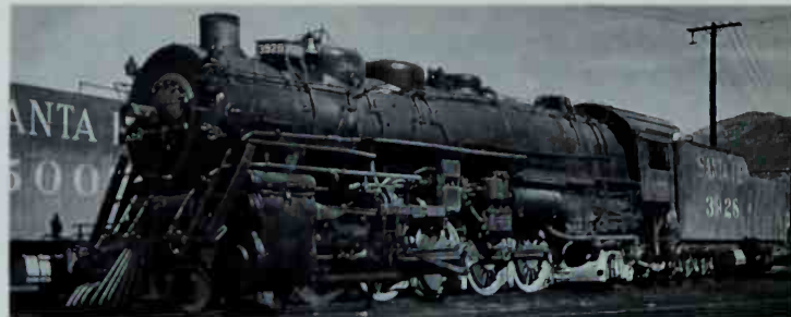
Number 900 was part of Santa Fe's second order for 2-10-2s. Note that the firebox extends over the rear pair of drivers. Number 3928 was among the last built. The drivers are larger, and the firebox lies entirely behind them. Both locomotives were photographed at Raton, New Mexico, in spring 1950. Photos by C. C. Tinkham.
