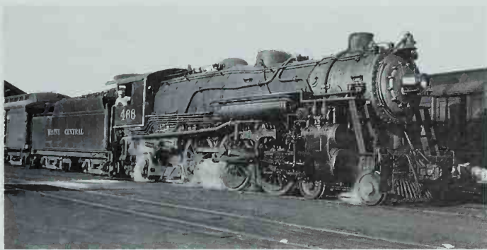
The C-3 Pacifics, built in 1917 and 1924, were up-to-date engines with cast trailing trucks and boosters. Photo by Peter Ascher.
