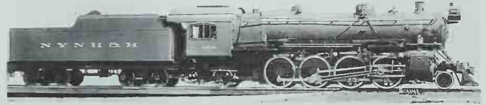
The J-1 Mikados had an extremely low profile, with cabs set much lower than customary. Alco photo.
