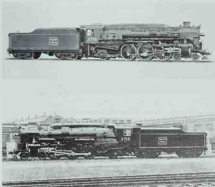
The official portrait of Boston & Maine P-4-a 3710 (Lima, 1934) shows the right side of the locomotive painted flat black. The running board and tires are trimmed in white and the rods have been painted white with the fluted areas filled in. Taken at the same time, the informal view of the left side shows glossy black paint and polished rods; the photographer's portable wood and canvas panels are visible behind the engine. Lima photos; lower photo, collection of Allen County (Ohio) Historical Society.
