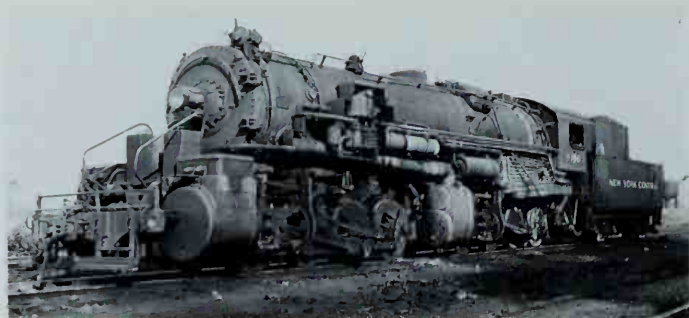
The most successful compound design was the Mallet. New York Central 7106 illustrates the difference in diameter between the high-pressure (rear) and low-pressure (front) cylinders. It was built by Alco in 1920; here in 1946 it was employed in hump switching at Selkirk Yard, near Albany, N. Y. Photo by LaMar M. Kelley.
