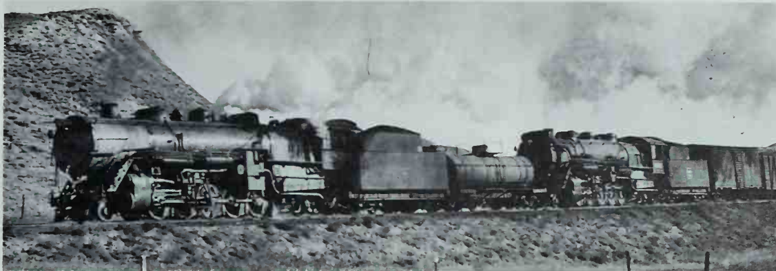
Fat-boilered 2-10-2s 6148 and 6161 lead a freight near Clearmont, Wyoming, in 1942. Both are lignite-burners and have extended smokeboxes. Number 6148 has Worthington BL feedwater heater; 6161 has an Elesco unit. The tank car behind 6148's tender is an auxiliary water car; the hoses and pipes are clearly visible along the side sill of the tender. Photo by W. R. McGee.
