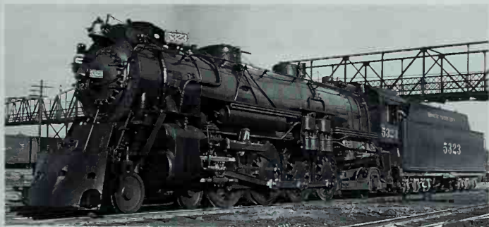
Mountain 5323, shown at St. Louis in November 1939, a month after emerging from Sedalia Shops, shows almost no trace of it USRA light 4-8-2 origins. The 75" drivers were the largest used on any 4-8-2 in North America. Collection of Louis A. Marre.
