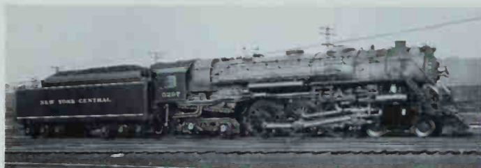
New York Central's Hudsons had tenders with large coal bunkers and small water tanks. NYC photo, collection of F. H. Howard.
