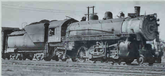
Mikado 2274, an MK-7 built by Baldwin in 1917, is typical of UP's Harriman Mikes. The trailing truck is an early version of Commonwealth Steel Company's Delta truck. Photo by Arthur Stensvad.
