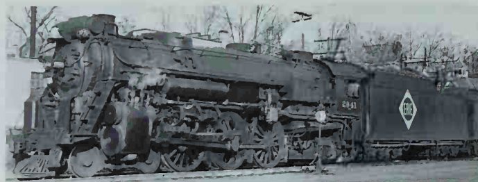
Only Erie had USRA heavy Pacifics, and the 1923 copies that Baldwin built were an improvement on a good design. The K-5-As were rebuilt in 1941 with cast frames and cylinders and pilot-mounted air pumps. Some received full sets of disk drivers; others, like No. 2941, had only their main drivers replaced. Photo by Vic Neal.
