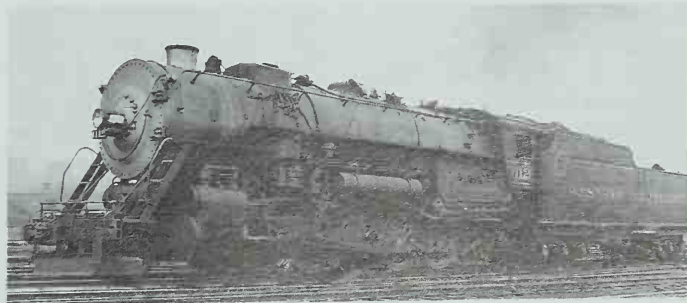
Western Maryland's 1-2 Decapods were enormous engines, outweighing the Pennsylvania Railroad's 2-10-0s by more than 16 tons. Collection of H. K. Vollrath.
