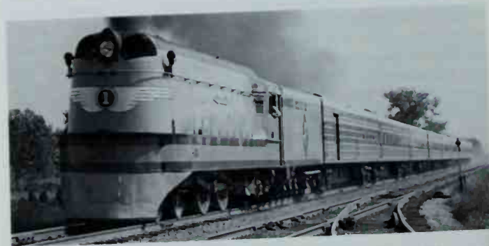
Milwaukee Road 1, shown at speed on a nine-car Hiawatha near West Lake Forest, Illinois, was the first steam locomotive built streamlined. Photo by Lucius Beebe.
