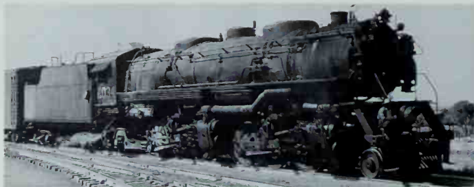
National Railways of Mexico was the only North American railroad to buy single-expansion 2-6 6-2s in quantity. Standard gauge 2034, built by Alco in 1937, is a thoroughly modern locomotive, and gives the impression of being a slightly under-scale Challenger. Photo by A. M. Payne.
