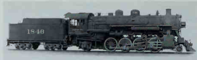
Mikado 1846 (later 646) was built by Lima in 1923. The Harriman influence is evident in the straight boiler and the deep-arched cab roof. Lima photo.
