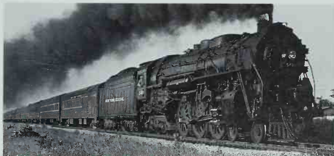
J-3a Hudson 5411 rolls through Trenton, Michigan, with the Cleveland Mercury in June 1953. A Worthington type SA feedwater heater has replaced the original Elesco unit. Photo by John Krave.
