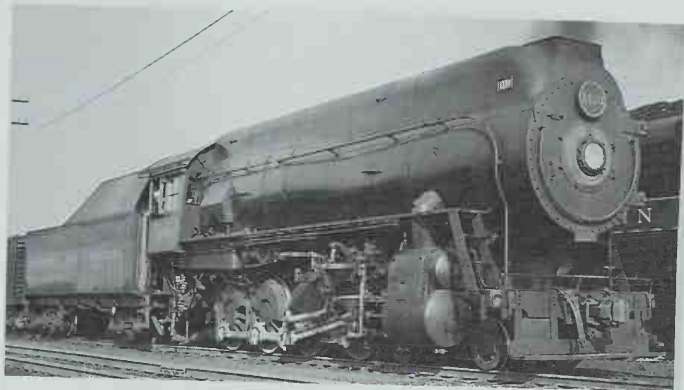
N&W experimented with a pair of 4-8-0s to create semistreamlined switchers with automatic stokers and injectors. Even with modern controls, they were old locomotives; the simplicity of modern 0-8-0s won out. Photo by H. Reid.
