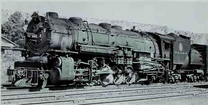
The Vanderbilt tender of Santa Fe type No. 1401 appears inadequate for what was once the largest two-cylinder locomotive in the world. Some of the 2-10-2s eventually acquired large rectangular tenders. Photo by R. H. Kindig.
