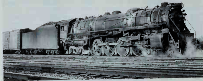
Visible in the photo of H-1 No. 3035 are Boxpok drivers and rollers bearings on the lead and trailing trucks. The unobstructed view of the trailing truck is evidence of the new frame. C&NW photo.
