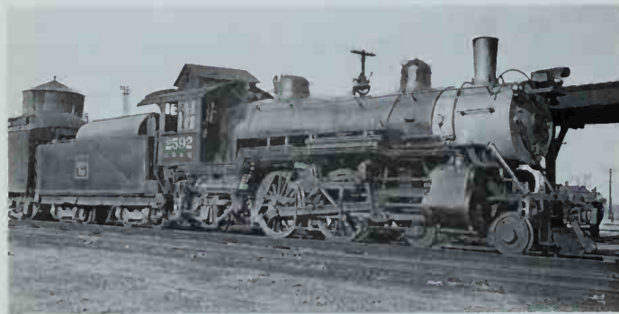
Number 2592, a P-6A, was rebuilt in 1927 from P-2 2544, a Rogers product of 1903. It lasted until 1951. The rebuilding included the replacement of the original 84 \frac{1}{4} " drivers with 69" wheels. Photo by Robert Graham.
