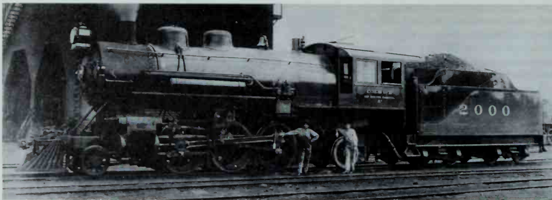
Milwaukee Road's 195 Prairies were more modern than most of their contemporaries, sporting piston valves and Walschaerts valve gear. The men posing with CM&StP 2000 are of average height (those are 63" drive wheels) and show how large even a small steam locomotive is. Milwaukee Road photo.
