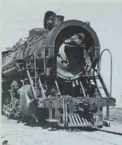
Locomotives built with Coffin feedwater heaters usually had the horse-shoe-shaped heater tank hidden in the smokebox. Coffin feedwater heaters added after the locomotive was built were usually hung in front of the smokebox, like that on Denver & Salt Lake Mikado 409. Photo by Ralph Hallock.
