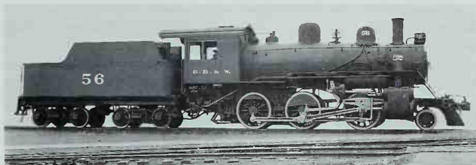
Green Bay & Western's Moguls were light engines, weighing about 140,000 pounds. Number 56 (later 256) was the last, built by Alco's Schenectady Works in 1924. Superheater, piston valves, and Walschaerts valve gear were state of the art, but the narrow firebox between the drivers and the wheel arrangement itself were long since passé. Alco photo.
