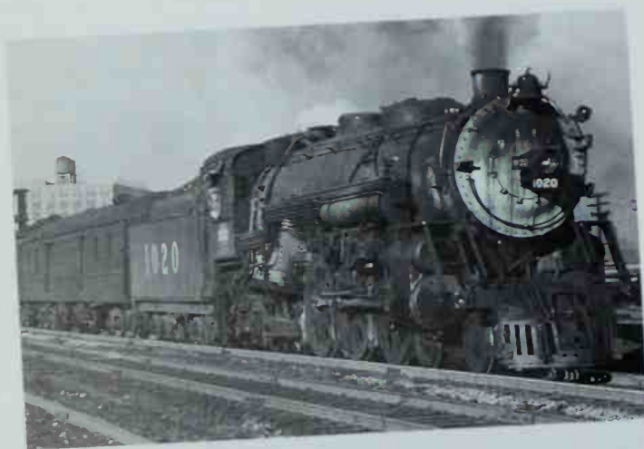
C&E's best-known engines were the six Lima heavy Pacifics of 1923. Number 1020 displays latter-day improvements — a cast, drop-coupler pilot and a full set of Boxpok drivers — as it accelerates the Dixie Limited out of Chicago on a winter day in 1947. Photo by Donald R. Deneen.
