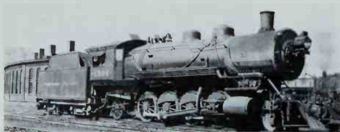
W-class Mikado 1504, shown out of service (the piston rod is missing), was part of the first large group of Mikados. Photo by Maurice L. Kunde.
