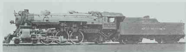
Many consider the Pacific reached its zenith, at least in terms of appearance, in Southern Railway's green-and-gold Ps-4 class, built by Schenectady, Richmond, and Baldwin between 1923 and 1929. It was a development of the USRA heavy Pacific. One example is on display in the Smithsonian Institution's National Museum of American History in Washington. BLW photo.
