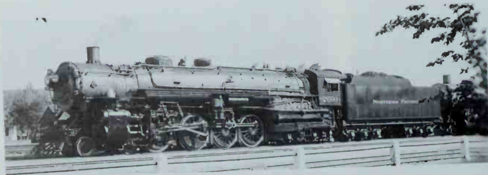
Northern Pacific 2600 was the first 4-8-4. The outside-cradle frame — the heavy frame members below the firebox and outboard of the trailing truck — was also used on Canadian National and Chicago & North Western 4-8-4s. Photo by R. V. Nixon.
