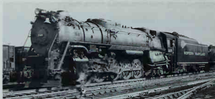
Vestibule cabs gave Western Maryland's Potomacs something of a Rio Grande look. The front end, though, was pure WM: high headlight, small rectangular number plate, and rock-pusher pilot. Photo by Russell L. Wilcox.
