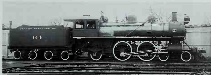
Atlantic 64 was built by Schenectady in 1905. It is typical of the time, with Stephenson gear and inside piston valves. Alco photo; collection of C. W. Witbeck.
