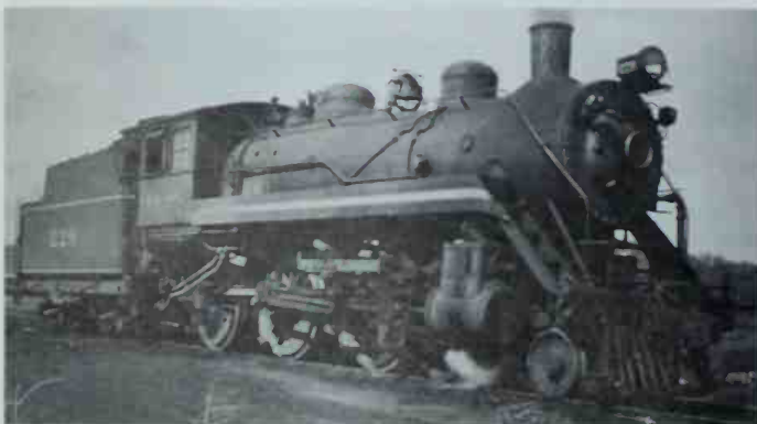
The G6-24 Ten-Wheelers were the last of their type on the roster, and at least one, No. 229, received running board skirts. Less obvious are piston valves retrofitted in the slide-valve steam chests. Photo by Robert Milner.
