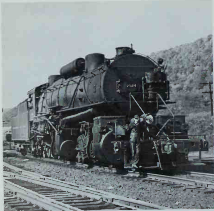
Baltimore & Ohio 7324, formerly Buffalo, Rochester & Pittsburgh 808, built by Brooks in 1923, drifts backward into the yard at Clarion Junction, Pennsylvania, after pushing a freight up Clarion Hill. The 2-8-8-2's low-pressure cylinders are 44" in diameter. It was common practice to use piston valves for high-pressure cylinders and slide valves for low-pressure cylinders on Mallets. Photo by W. G. Thornton.
