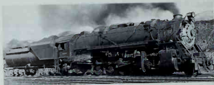
The 63" drivers of S-1 No. 6208 are larger than customary for 2-10-2s. They made B&O's "Big Sixes" fast freight power, not drag locomotives. Hundman Collection.
