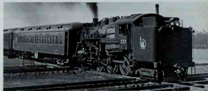
Central Railroad of New Jersey 227, a 4-6-4T, leaves Elizabethport, N. J., with the shuttle train for Newark, 7 miles away. The narrow coal bunker allows the crew to look out directly to the rear; the headlight and pilot duplicate equipment at the front of the locomotive. Photo by C. A. Brown.
