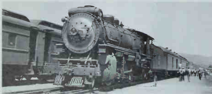
Western Pacific's Mikados occasionally pulled passenger trains. Number 326 is at the head of train 39, the westbound Exposition Flyer , at Portola, Calif., on July 4, 1940. WP's Mikes all had Elesco feedwater heaters. Later classes were built with them; earlier classes received them during visits to the shops. Photo by Guy L. Dunscomb.
