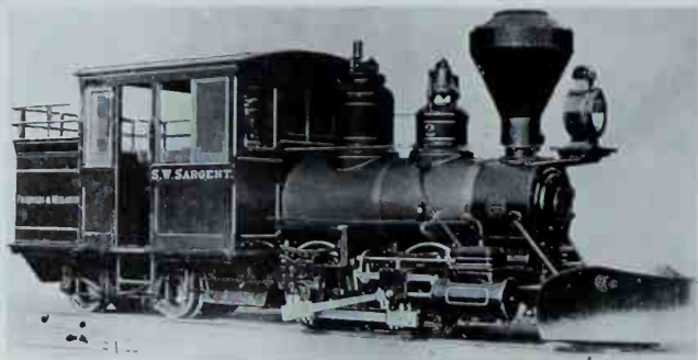
Franklin & Megantic 2 was photographed without its right running board to show details of its outside frame. Collection of Linwood Moody.
