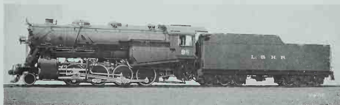
Consolidations 90-95 were large by anyone's standards. The 100 square feet of grate area was the same as Lima's Super-Power Berkshire, and more than Reading's 4-8-4s. Baldwin photo.
