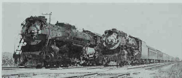
The Hudsons and the Baldwin 4-8-4s looked very much alike. A comparison is possible as Hudson 3005 leads the Exposition Flyer past a freight behind O-5 5601 at Somonauk, Illinois, in September 1944. Photo by L. E. Griffith.
