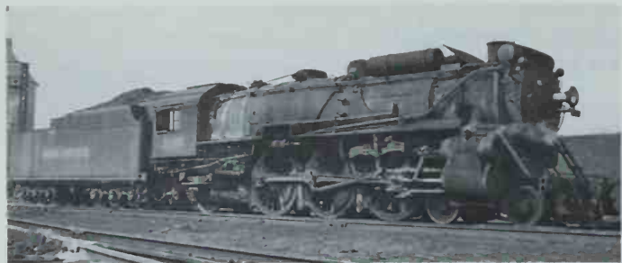
The Pacifics most characteristic of the New Haven were the I-4s. They were built in 1916 and were top passenger power for 20 years. Elesco feedwater heater, air reservoirs atop the boiler, and 12-wheel tenders were later modifications. Photo by E. R. Meakes.
