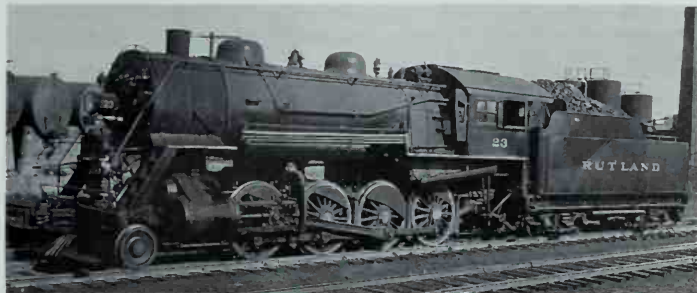
In the late 1940s Consolidation No. 23 (Schenectady, 1907) was equipped with a stoker and had its air pump moved to the pilot; Stephenson valve gear remained. Photo by H. N. Proctor.
