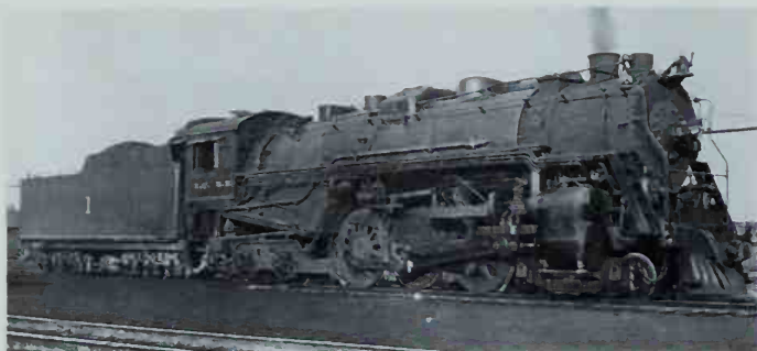
The first attempt at rebuilding the 2-8-4s resulted in the only Hudson designed for freight service in North America. It was too powerful for its weight. Photo by C. W. Witbeck.
