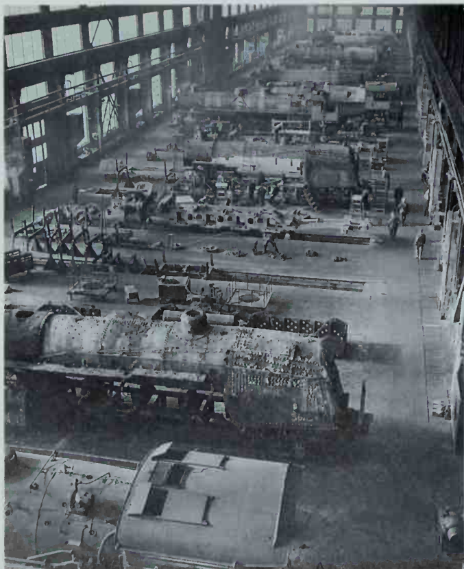
Paducah Shops was the road's principal rebuilding facility. Locomotives entered the erecting hall at one end and were carried sideways by a crane to the pit track where all the work was done. IC photos.
