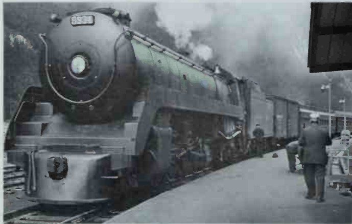
The Selkirks of 1938 were unique on two counts for ten-coupled steam locomotives: they were streamlined and they were built for passenger service. Rail Photo Service photo by G. C. Corey.
