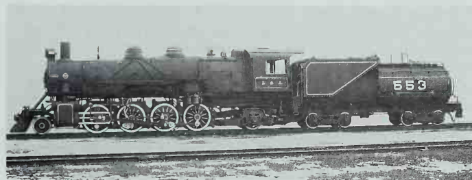
L&A's M-21 Mikados, built by Baldwin between 1923 and 1927, looked older than they were because of the striping on the drivers and the shape of the domes. Baldwin photo; collection of H. L. Broadbelt.
