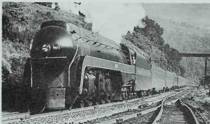
N&W's top passenger trains rated J-class 4-8-4s, though the seven cars of the Powhatan Arrow hardly tax No. 607 as it whistles into Glen Lyn, Virginia. The train's total weight is about the same as the weight of the engine and tender. Photo by Ben F. Cutler.
