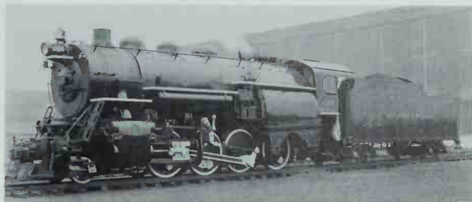
Class E-68 (formerly E-5a) 2-8-0 No. 1119 represents Delaware & Hudson's last series of nonexperimental Consolidations, built by Colonie Shops in 1929. The outboard lead truck journal and the outside ashpan hoppers are typical D&H details. D&H photo.
