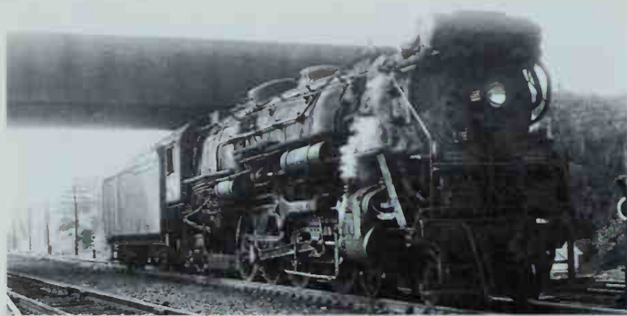
The last steam freight engines NH purchased were the R-3-a class, three-cylinder 4-8-2s. Number 3558, built by Alco in 1928, was still in service in 1950, awaiting helper duties at Hopewell Junction, New York. Photo by John V. Weber.
