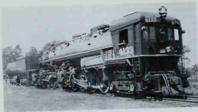
SP's cab-forwards gave the engineer a forward view unequaled by any other steam engine. Number 4133, built by Baldwin in 1930, was an AC-6, the last class with flat-front cabs. Baldwin photo; collection of H. L. Broadbelt.
