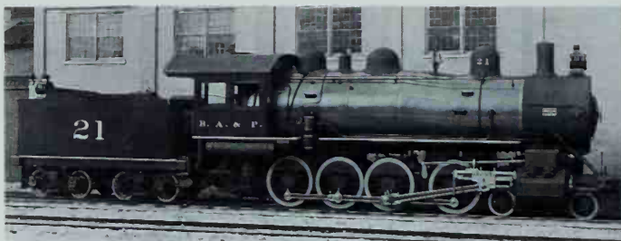
Butte, Anaconda & Pacific 21, photographed at Alco's Schenectady Works in 1903, is a cross-compound. The jacket and insulation of the large low-pressure cylinder on the right side have been trimmed for clearance. Notice that the right side of the locomotive has been specially painted for the photo with flat
