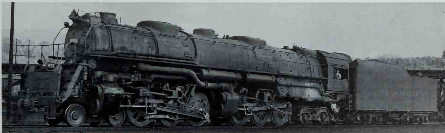
Clinchfield's first Challengers, 650-657, were based on Delaware & Hudson's class J 4-6-6-4. Photo by C. W. Witbeck.
