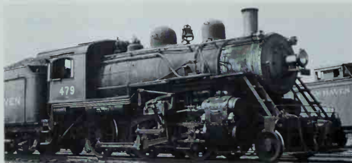
New Haven chose the Mogul as its standard freight locomotive at the turn of the century and had 226 of the type built after 1900. Number 479 was the highest-numbered but not the last built. Southern valve gear and piston valves were added after No. 479 had been in service several years. Photo by Kent W. Cochrane.
