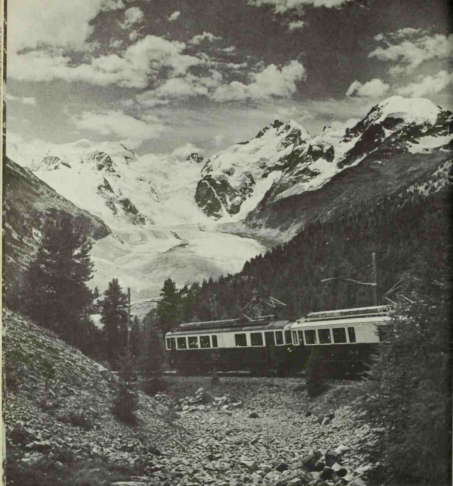
The Rhetian Railway near Monte Bello on the Bernina line with the Bernina group of mountains in the background, the highest and steepest adhesion railway in Europe. Its highest station is Bernina Hospiz, 7,405 feet, and its gradient is 7 per cent.
