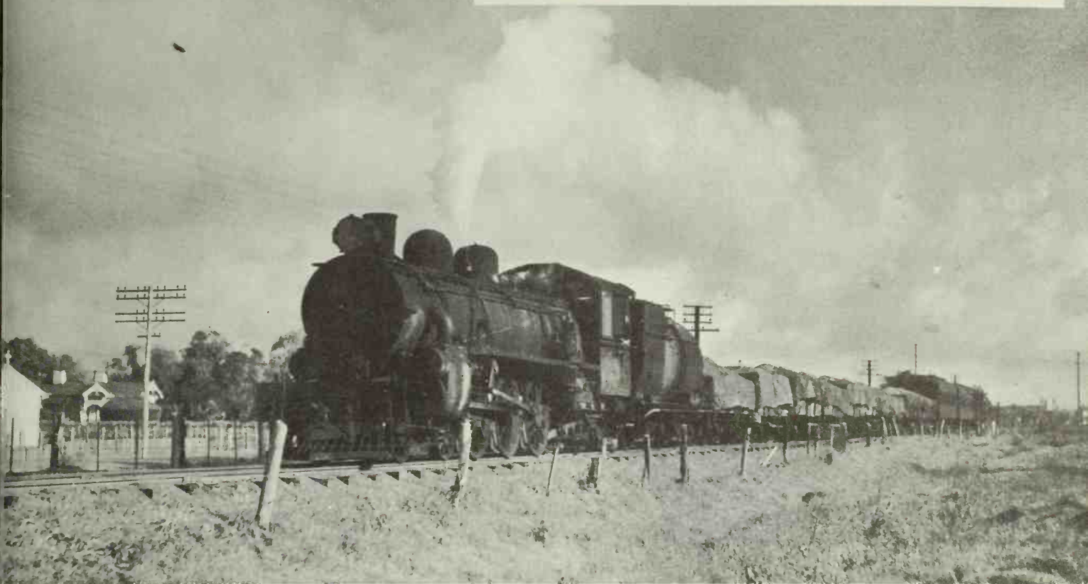
A typical New Zealand mixed train #107 with a Class AB locomotive 4-6-2 type passing Aorangi. (Photo by W. W. Stewart)
