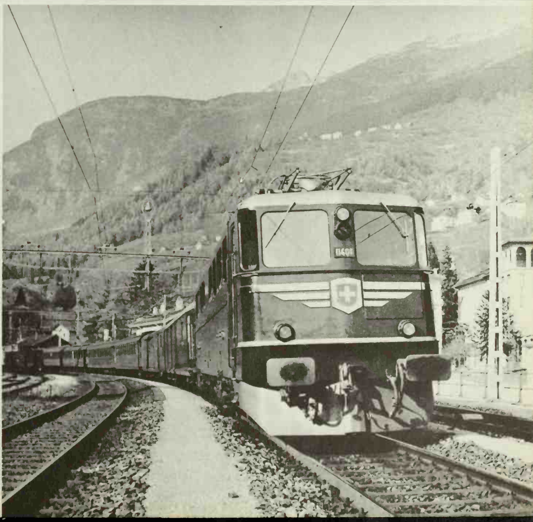
The AE 6-6 specially built for the Gotthard Line.
