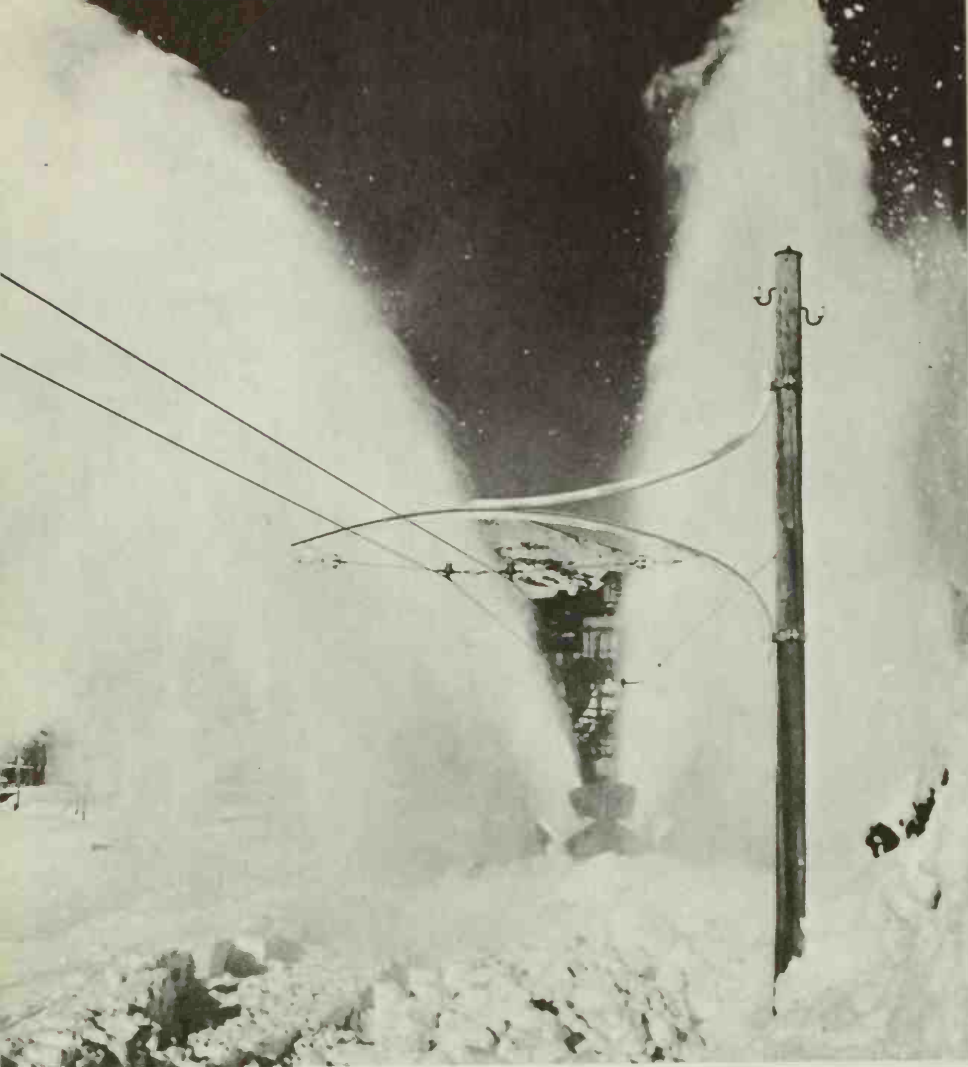
This rotary snowplow is really clearing the line to the Jungfrau at Eiger Glacier on the Jungfrau Railroad at an altitude of 6,720 feet.
