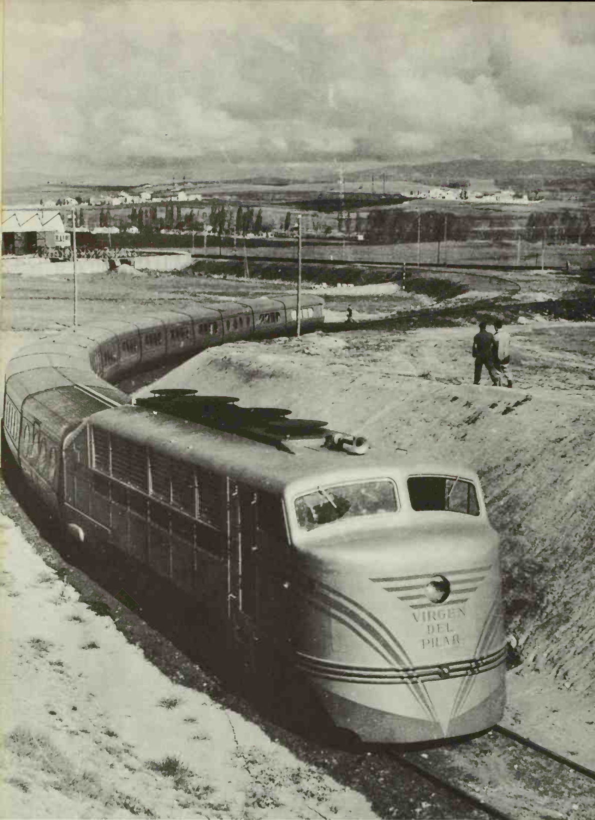
The Talgo train, built in the United States by the American Car and Foundry Co., started its regular passenger service on the Madrid-Hendaye line of the Spanish National Network in July of 1950, and has covered over a million kilometers with not too many serious mechanical difficulties.
