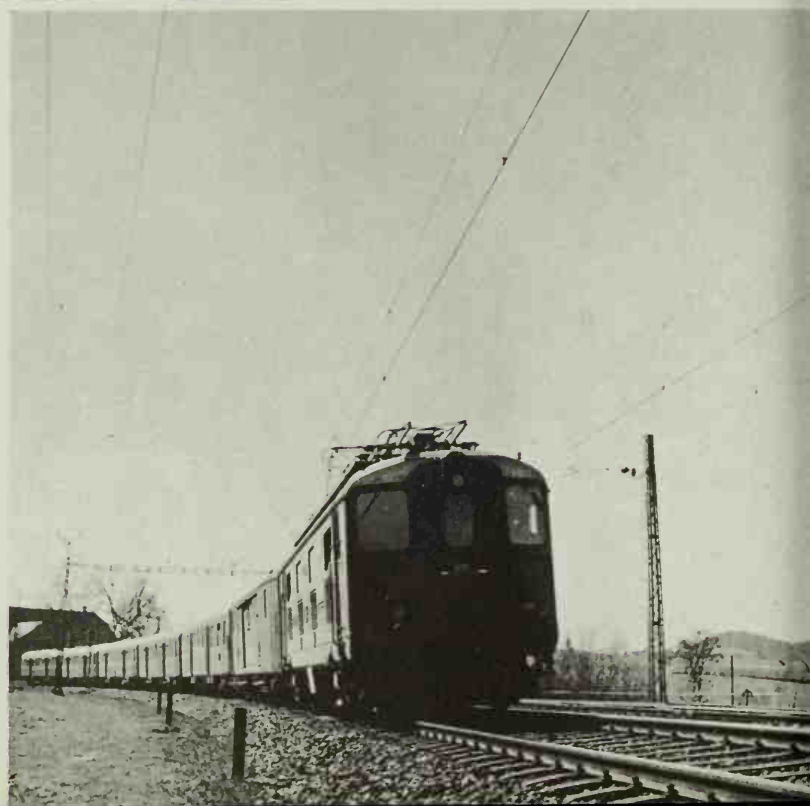
Type of lightweight fast train used between the big cities in the midlands of Switzerland. The locomotive is Class R 4-4.
