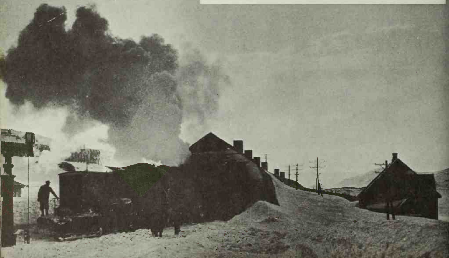
Another type of Norwegian plow and doser, working at Ustaoset on the Norwegian State Railway.
