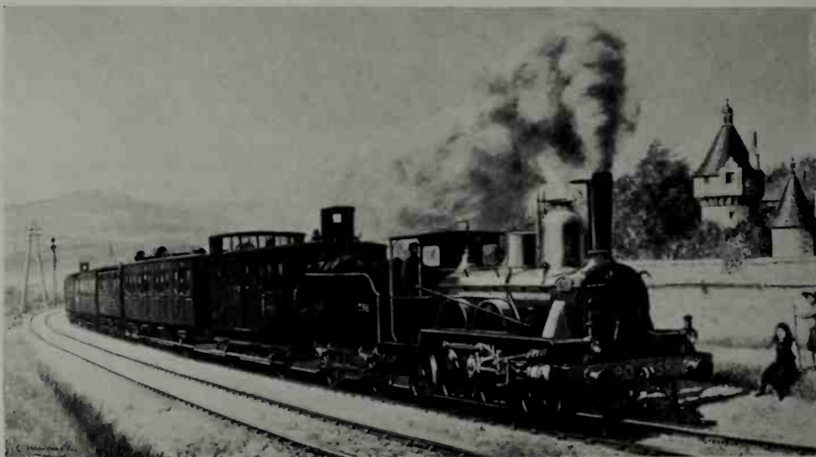
143-5. Nineteenth-century France: Above is a train on the Eastern Railway, headed by a Crampton engine ( Odessa ), piloting a post- Crampton 2-4-0. In the middle is an express of the Paris-Orleans Railway in the 'nineties. The engine, a particularly fine example of old French styling, was clothed in polished brass. Highfliers of the Northern Railway of France during the 'eighties were the imposing Oustrance-class bogie engines, one of which, in the lower view, is heading a train through the chalk downs of the Pas de Calais.
