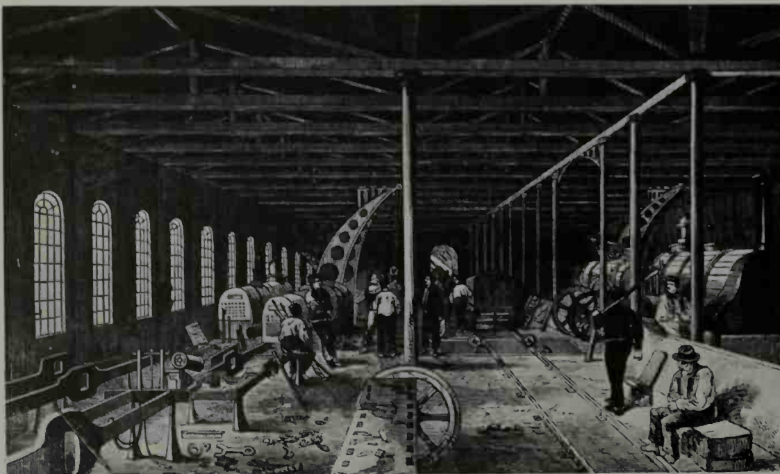
113. Erecting shop of the Grand Junction Railway at Crewe in 1849, with one of Alexander Allan's locomotives being assembled.
