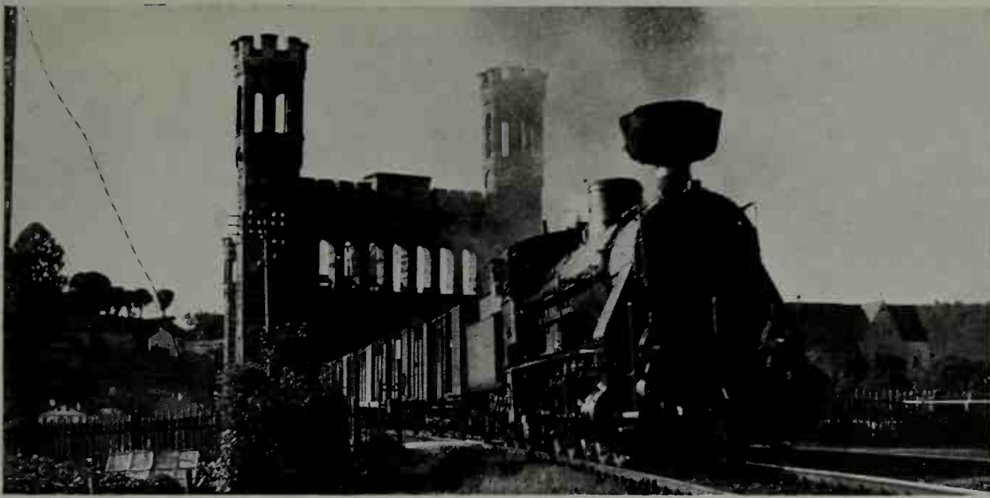
255-6. Austria: Left, a goods train comes off the international bridge at Passau, between Austria and Lower Bavaria. In the lower view, a train dives under Falkenstein on the Tauern line, Carinthia. Both the engines shown are lignite-burning 0-10-0 of Gölsdorf's design.
