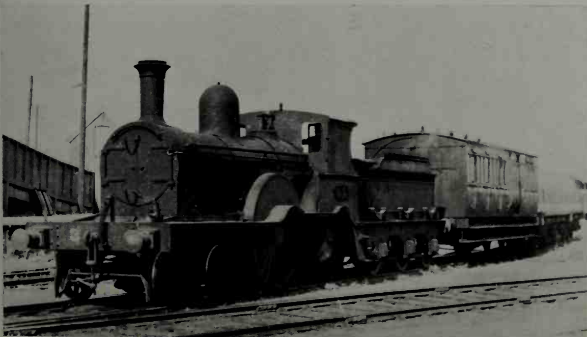
217. Typical of Irish broad-gauge practice in the 'nineties was this express engine of the Great Southern and Western, likewise the squat, six-wheeled brake-third.
