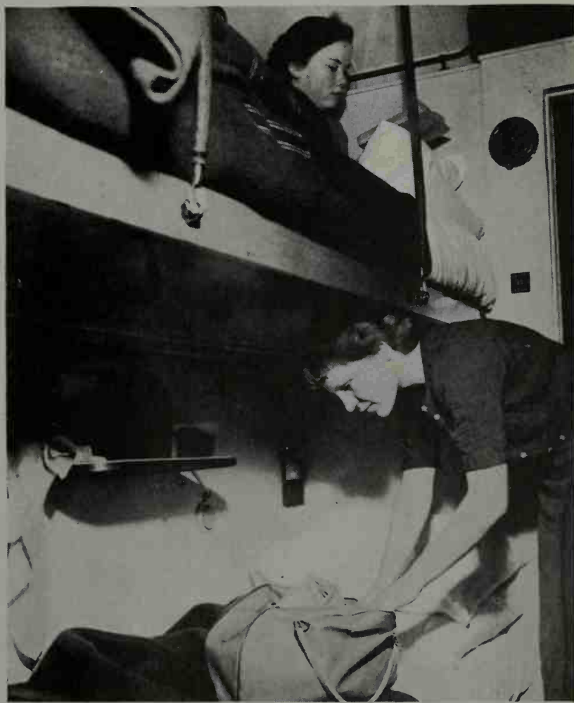
374-5. British first-class sleepers have changed in style rather than arrangement (see 191). Above the attendant's cap is the ball-and-socket joint of the forced ventilation system, arranged for warm or cool air. On the right is a superior category third-class sleeping compartment on a Scotch express in 1951. There are two berths with made-up beds, but the occupant of the lower one must still mind her head.
