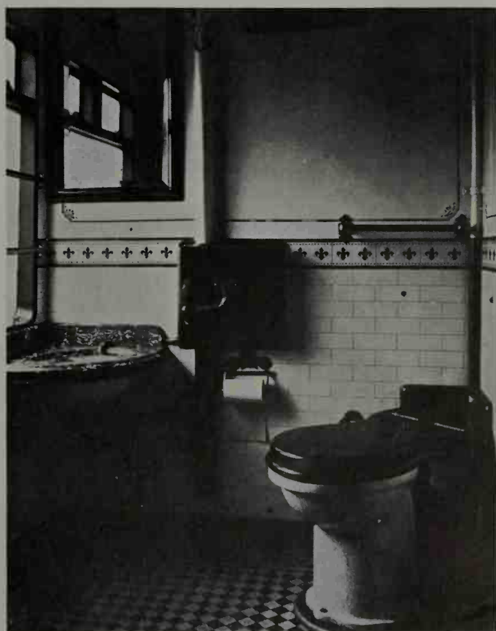
161. Train lavatories ranged from the dreadful to the creditable. This, on the North Eastern in 1911, was excellent of its period, with a pedestal valve closet, flushed by closing the lid.
