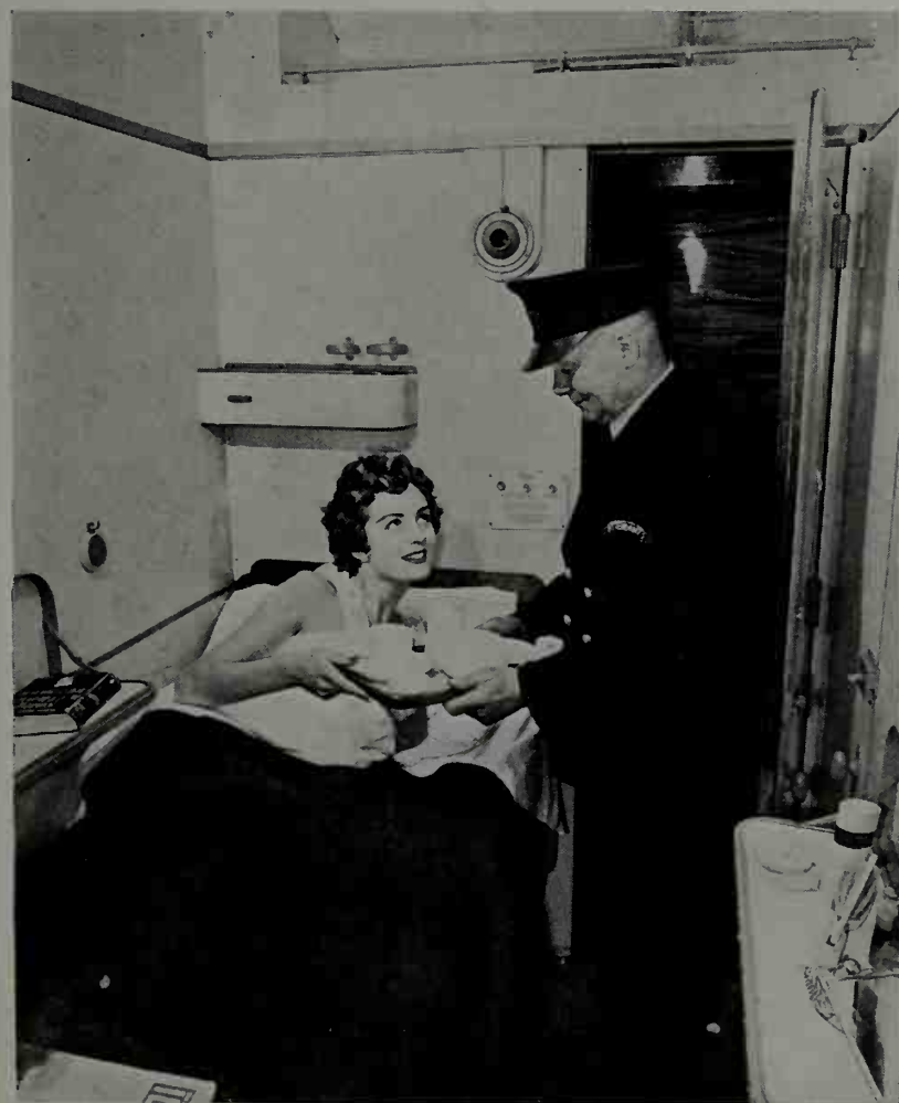
374-5. British first-class sleepers have changed in style rather than arrangement (see 191). Above the attendant's cap is the ball-and-socket joint of the forced ventilation system, arranged for warm or cool air. On the right is a superior category third-class sleeping compartment on a Scotch express in 1951. There are two berths with made-up beds, but the occupant of the lower one must still mind her head.
