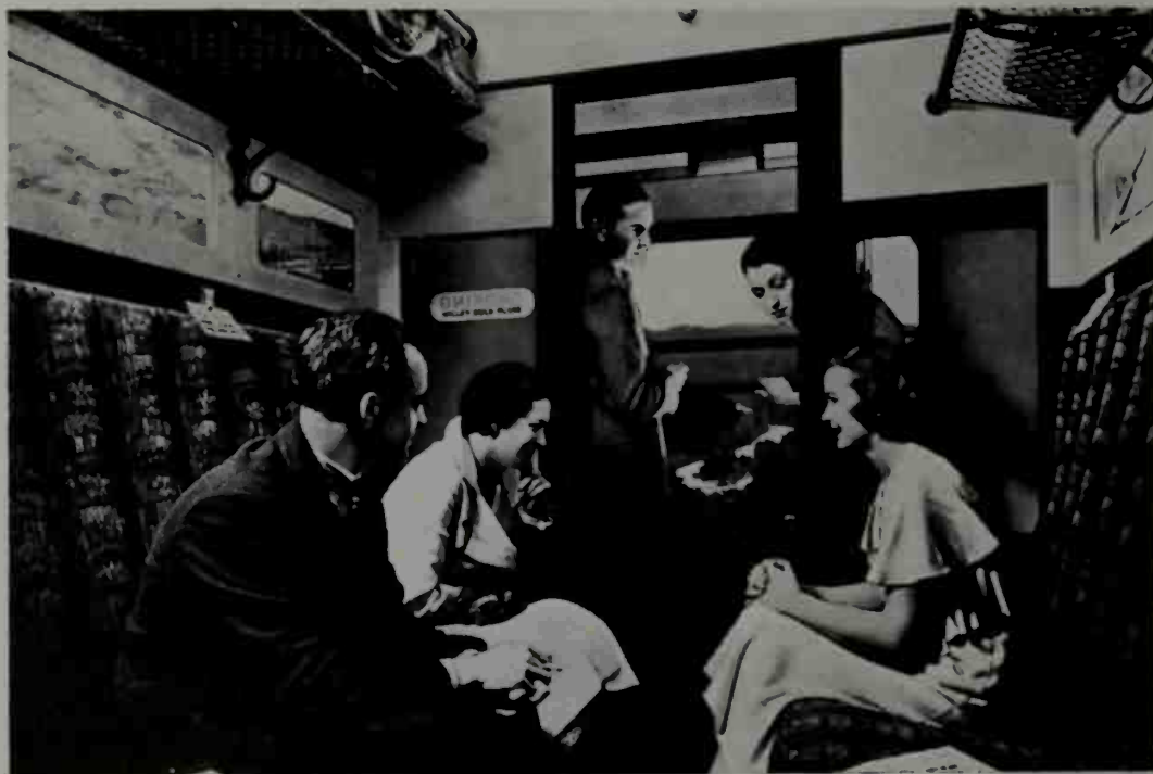
370. Third-class sleeping cars, long-established in Russia and Scandinavia, reached Great Britain in 1928. At first, except on the Great Western, they were made as convertible day coaches; this unconvertible L.M.S. example belongs to the middle nineteen-thirties. Bedding consists of a spring mattress, a rug and a pillow. (Russia provided these on hire, and Sweden furnished full bedding without charge.)
