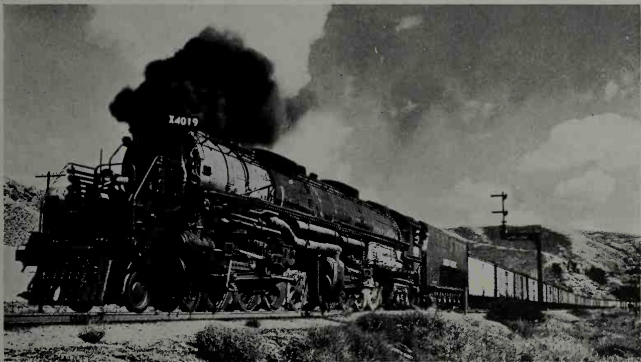
362-4. U.S.A., the passing of steam. Above is the City of Portland of the Union Pacific Railroad, headed by three General Motors oil-electric locomotives working in multiple-unit. The nineteen-fifties saw an extraordinary recession in steam traction; the latter days of steam, at the same time, produced some giants, such as this 4-8-8-4 Mallet of the Union Pacific, leading a freight train through the Black Hills of Wyoming in the late 'forties. Below, a later essay, is a gas-turbine locomotive, also on the Union Pacific.
