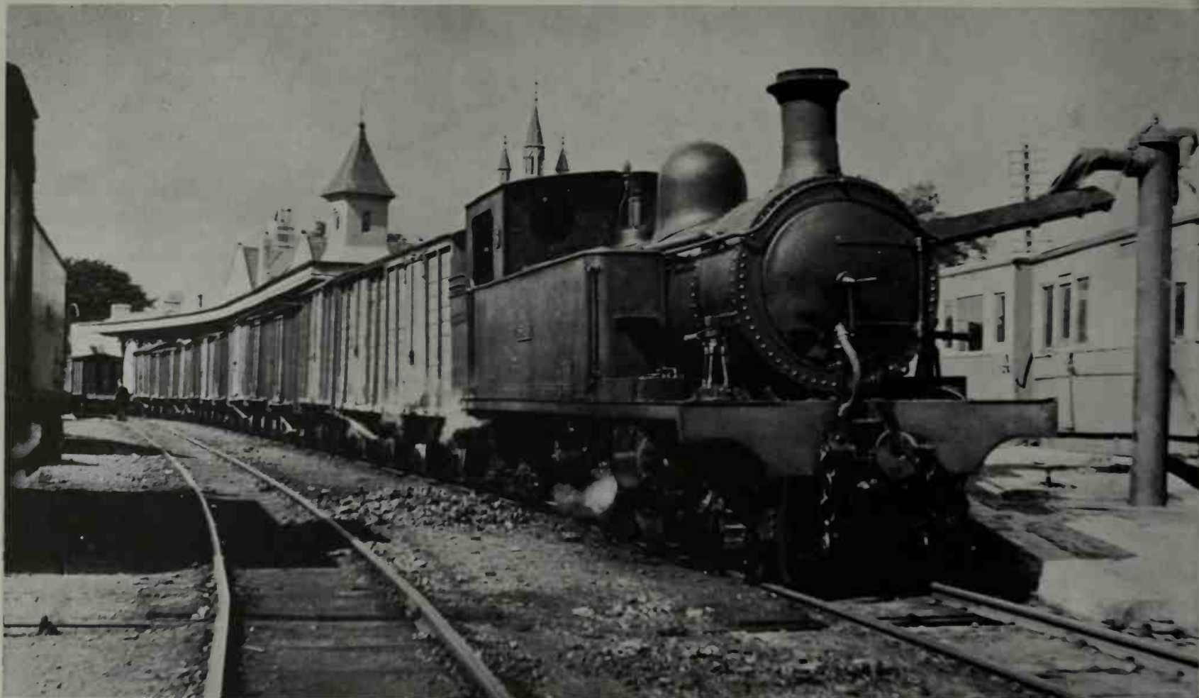
236-7. Narrow-gauge in Ireland could produce quite imposing effects. Above is an up Killybegs goods train at Stranorlar, County Donegal Railways, with 2-6-4 tank engine Columkille . The C.D.R., it should be remarked, was the pioneer in these islands of oil-engine traction. In the lower view, on the Tralee and Dingle line of Coras Iompair Eireann, a double-headed cattle train bellows on its way through the mountains of Kerry.
