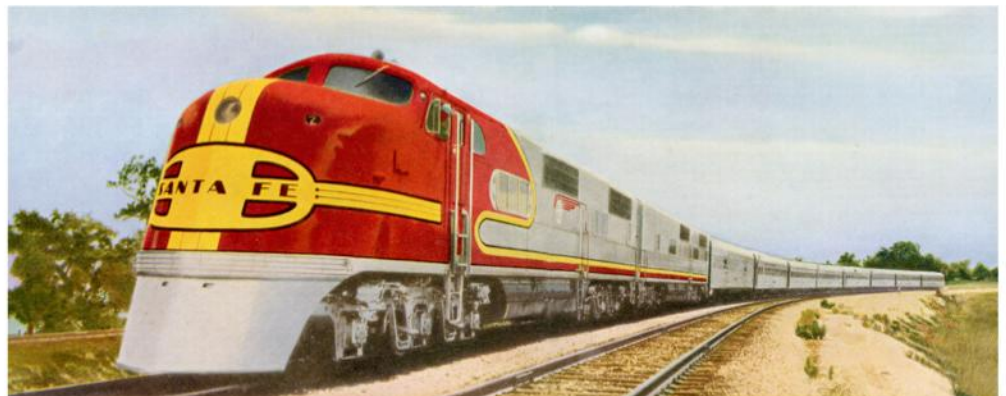
Diesel No. 2 missed the streamlined Super Chief's debut, taking the reins a month later. Underneath their streamlined styling and Warbonnet livery, and above their A1A trucks, the E1A-E1B duo was internally similar to the original Super's box-cabs.
