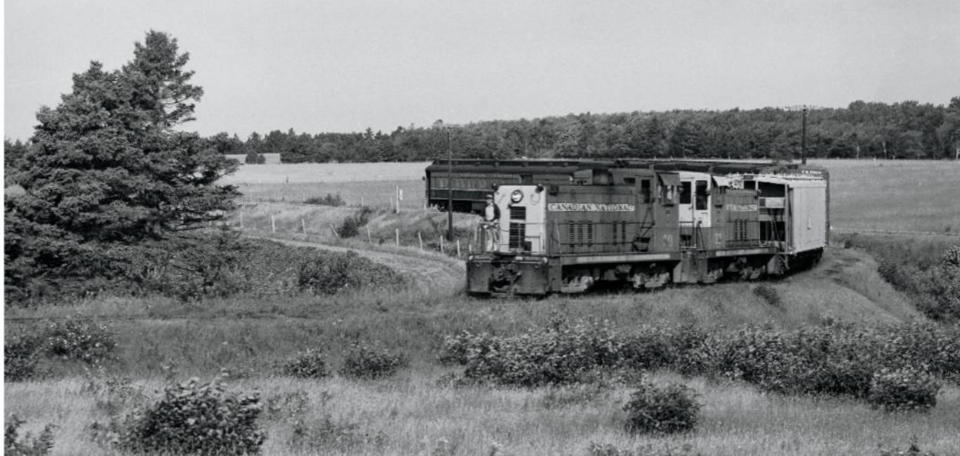
Mixed train M217 from Summerside rounds the west leg of the wye at Emerald Junction before backing up to the station to await train 39's arrival. This is an example of the sharp curves on P.E.I. that, in a test, would help deem a Budd RDC not usable on the island's railway.
