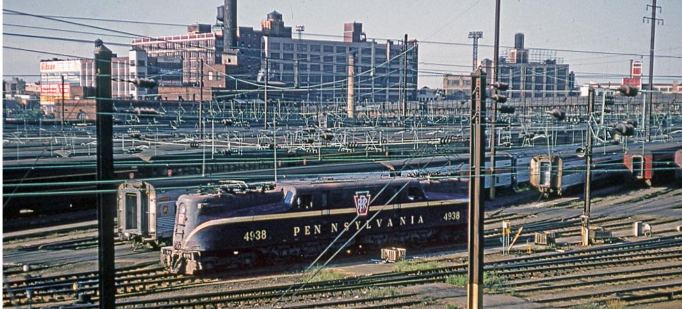
GG1 4938 (above) moves around the catenary-crowned trackage at Sunnyside Yard, the sprawling passenger facility east of Penn Station. A train of MP54 "red cars" (left) passes the Long Island's Hunterspoint station as it moves from Sunnyside to Penn Station.
