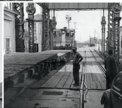
The author saw 70-tonners 39 (left) and 42 working the Borden slip. In a view from an idler flat-car (bottom left), brakemen signal engineers working the Abegweit as train 40's baggage car is pulled onto land. As seen from the ferry's rail deck (below), 39 pushes a cut of freight cars on board. When space allows, motor vehicles are carried here — note the Volkswagen at right.
