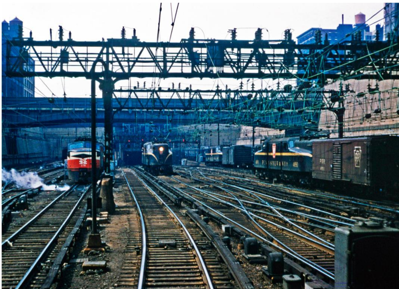
A view west from Penn Station toward the Hudson River tunnels reveals a New Haven EP-5, a GG1 running light, Long Island Rail Road M.U. cars laying over, and two more GG1s, each with a PRR express boxcar. This open area has recently been covered over by a new building.
