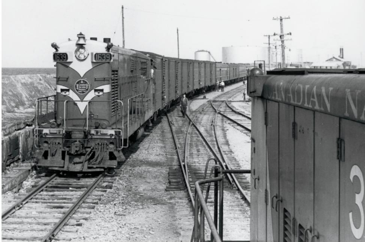
As seen from 70-tonner 39, the Borden ferry-slip switcher, train 39, the daily-except-Sunday "Boat Train" to Moncton, N.B., has arrived from Charlottetown behind H12-44 1639. Carmen appear ready to separate the front-end express boxcars from the RPO, baggage car, and coaches at the rear. The H12s on P.E.I. wore CN's road-unit livery of green and yellow.
