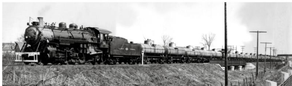
Having gone under the NYC, IT 30, one of three 1929 Baldwin 2-8-2s, is on the original (1895) Illinois Terminal linking Alton and Edwardsville with empties for Roxana refineries in the late '40s.
