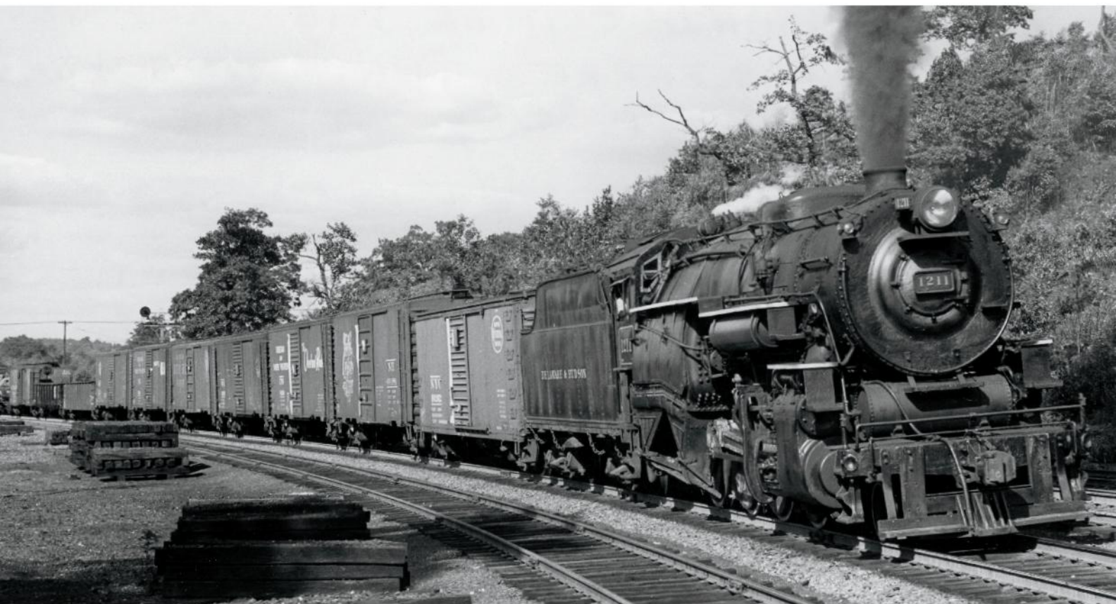
Bound for Buttonwood Yard and interchange to the Pennsylvania Railroad, a D&H freight with E-6a 2-8-0 No. 1211 up front climbs the last grade into Wilkes-Barre on September 20, 1950. Already Alco road-switcher diesels are on the Delaware & Hudson scene. The varied boxcar consist suggests overhead traffic, which, after shipments of anthracite coal began to wane, D&H parlayed into its slogan "The Bridge Line."
