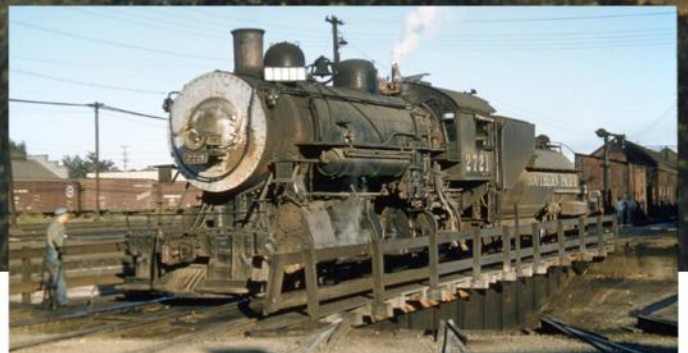
San Jose, Sept. 10: Consolidation 2721, a 1904 Baldwin, rides the turntable in preparation for a day's work in local freight service.
