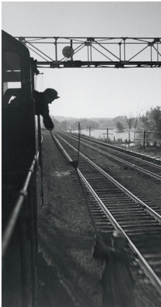
The operator at Portage, Ill., hoops up orders to the engineer of an Illinois Central GP9 in 1957. A few years later at Champaign, the same procedure didn't go so smoothly.
