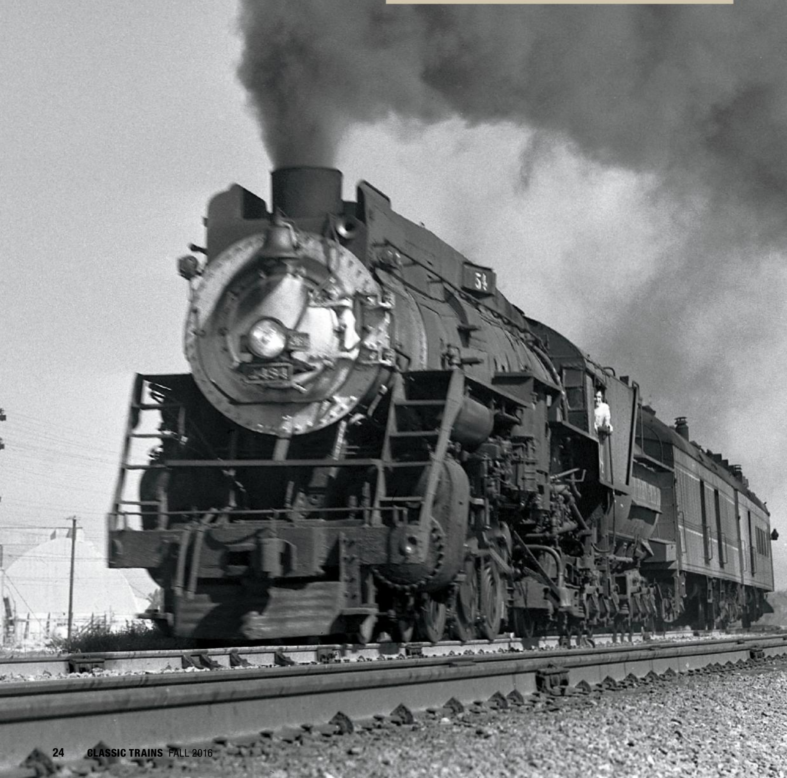
Tracy, Sept. 8: Class SE-4 0-8-0 No. 4507 switches the yard. SP's Sacramento Shops built 16 engines of this class during the 1930s.
