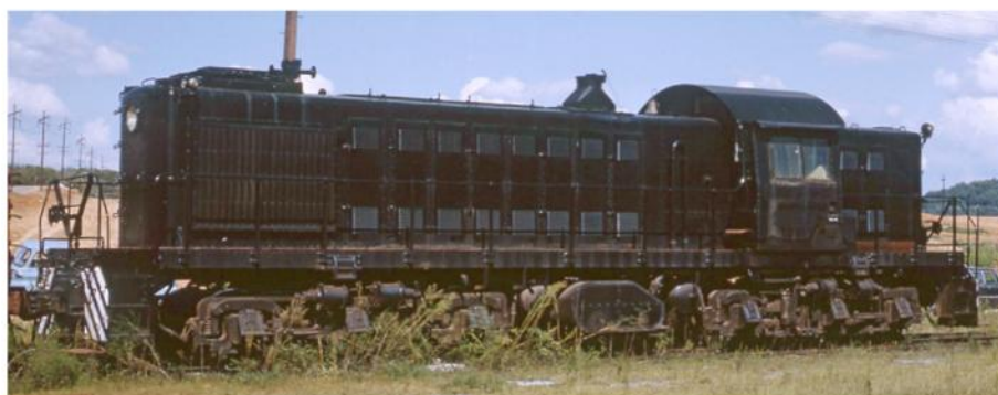
Also on September 20, I found at L&N's yard this Alco "RSD1," the six-motor version of the RS1, of which 87 were built for the U.S. Army. Neatly painted out on the long hood were "SOUTHERN" and the road's round emblem, and "USAEC 8659" on the cab. Disguised for security purposes as a civilian unit, it had served at Oak Ridge, the nuclear-weapons-development "secret city," and was being sent to scrap. According to an April 1980 TRAINS roster, it was assigned to the Atomic Energy Commission there about 1946.
