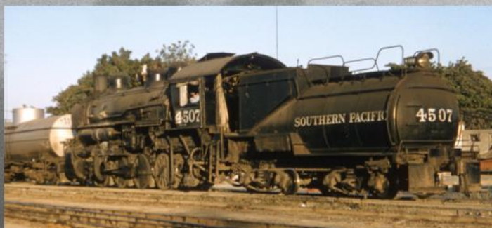
Tracy, Sept. 8: Class SE-4 0-8-0 No. 4507 switches the yard. SP's Sacramento Shops built 16 engines of this class during the 1930s.
