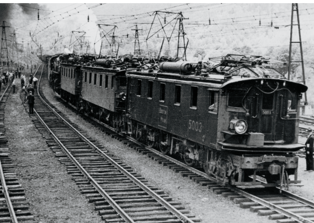
B&M's short electrified section, based on New Haven designs, operated 1911-46 to get trains through Hoosac Tunnel. Here, three motors haul a westbound freight at East Portal in May '38.
