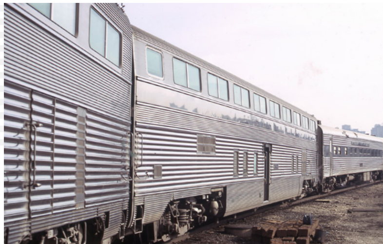
The angled top window panel identifies the middle car as one of the two Hi-Level prototypes in this 1972 photo of Amtrak's Super-El Cap .
