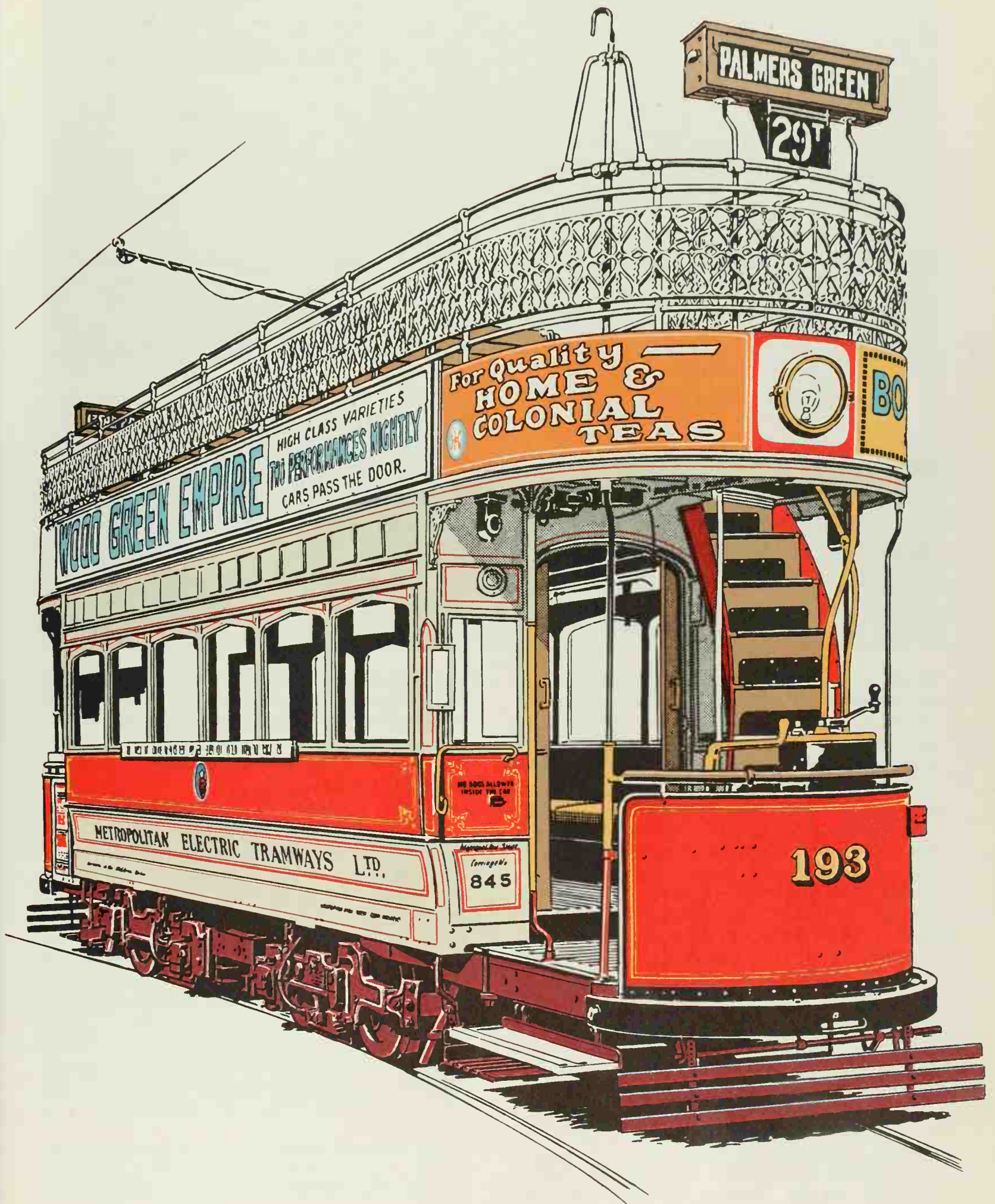
Class C1 M.E.T. car built in 1908, pictured after its adaptation for through running with L.C.C. but before the top cover was fitted
