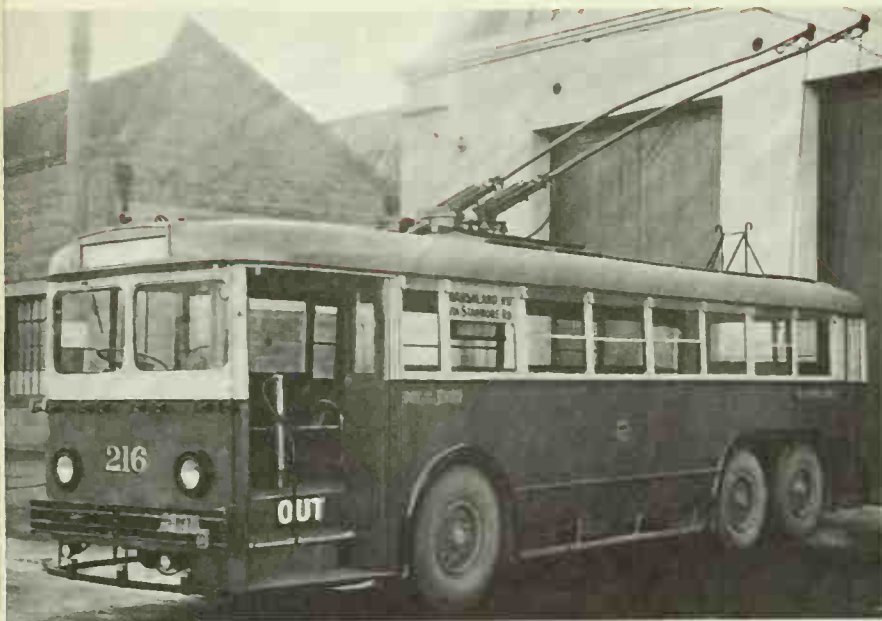
Left: A trolleybus which ran in Christchurch, New Zealand from 1952 to 1956; note the front hooks for transporting baby carriages
