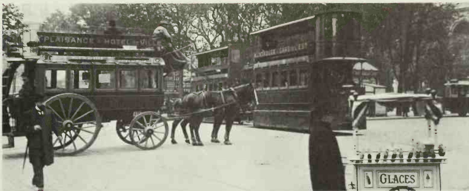
Top: Behind the ice-cream man at the Place du Châtelet, Paris—a Mekarski compressed-air tram and a horse bus with 'knifeboard' seating on the top deck
