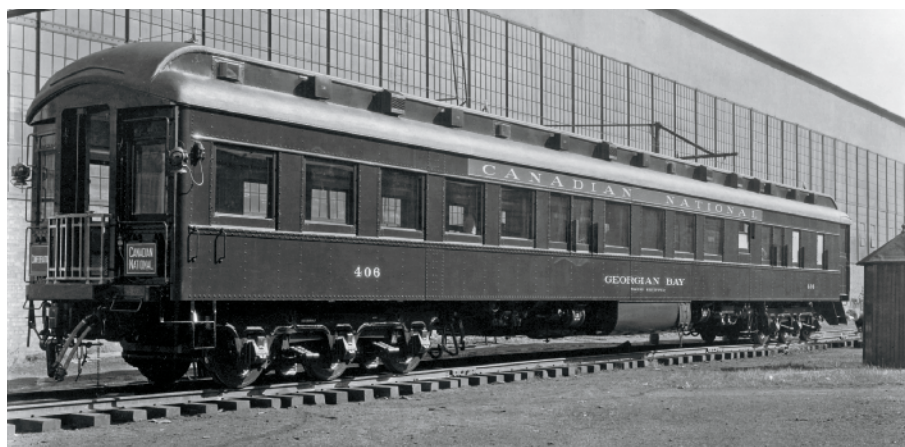
Georgian Bay , a 1930 solarium-lounge, featured radio gear, per the RADIO EQUIPPED lettering below the car name. Air-conditioning is yet to come — note the cinder shields on some windows.
