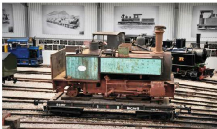
↑ Another new acquisition at the Statfold Barn Railway is Cameroon Development Corporation Hunslet 0-4-2T No. 3756. The locomotive has a 'colonial' cab, which will be re-attached.
