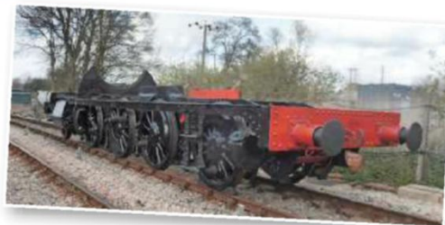
↑ The newly wheeled frames of '42XX' No. 4253 at Rolvenden on March 31. CHARLIE MASTERSON
