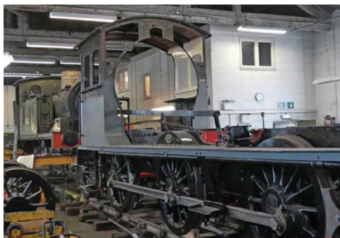
Evoking memories of nearby North Road Works, 'J27' No. 65894 awaits the return of its boiler at NELPG's Darlington Hopetown Works, while 'J72' No. 69023 is lifted for attention to its axleboxes. MICHAEL DENHOLM
