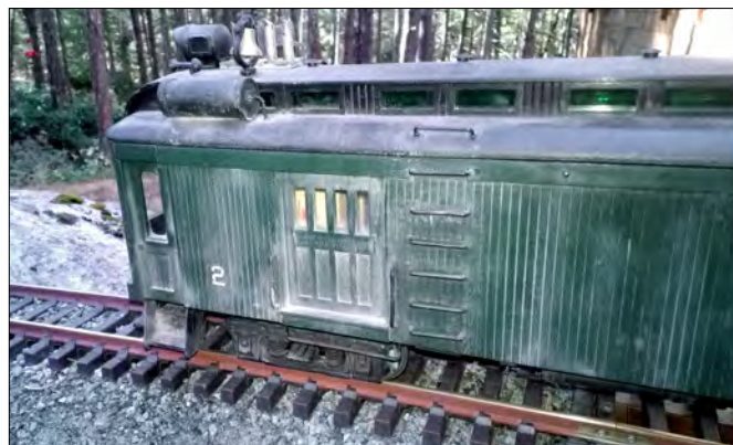
Roof access is provided by new grabirons aft of the baggage door. A new step below the baggage door has also been added.
