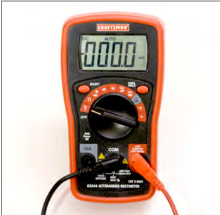
1. A multimeter has three basic parts: the display (digital shown), the dial (to select what you want to measure), and the probes (to connect to the component being measured.)
