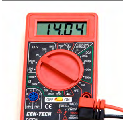
2. With a traditional meter, you must select from a range of values within which you believe your voltage, current, etc. might read. Here, the meter is set to 20V and displays the measured voltage (of a throttle) at 14.04V DC.
