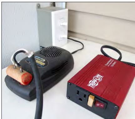
3. On the left is the fan-cooled 110V AC-to-12V DC converter/power supply; on the right is the 12V DC-to-110V AC inverter to provide correct current for the battery charger.
