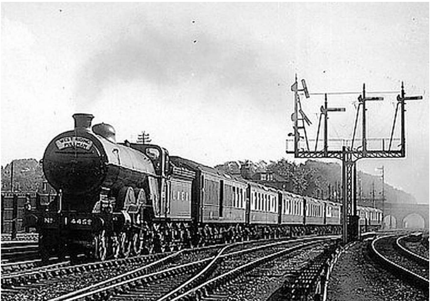
When originally built in August 1908, large boiler Atlantic N° 1451 was built without a superheater, receiving one in March 1922. It was then renumbered by the LNER, first becoming 4451 and later 2881. The image shows it working the 'West Riding Pullman'. (Author's Collection)
