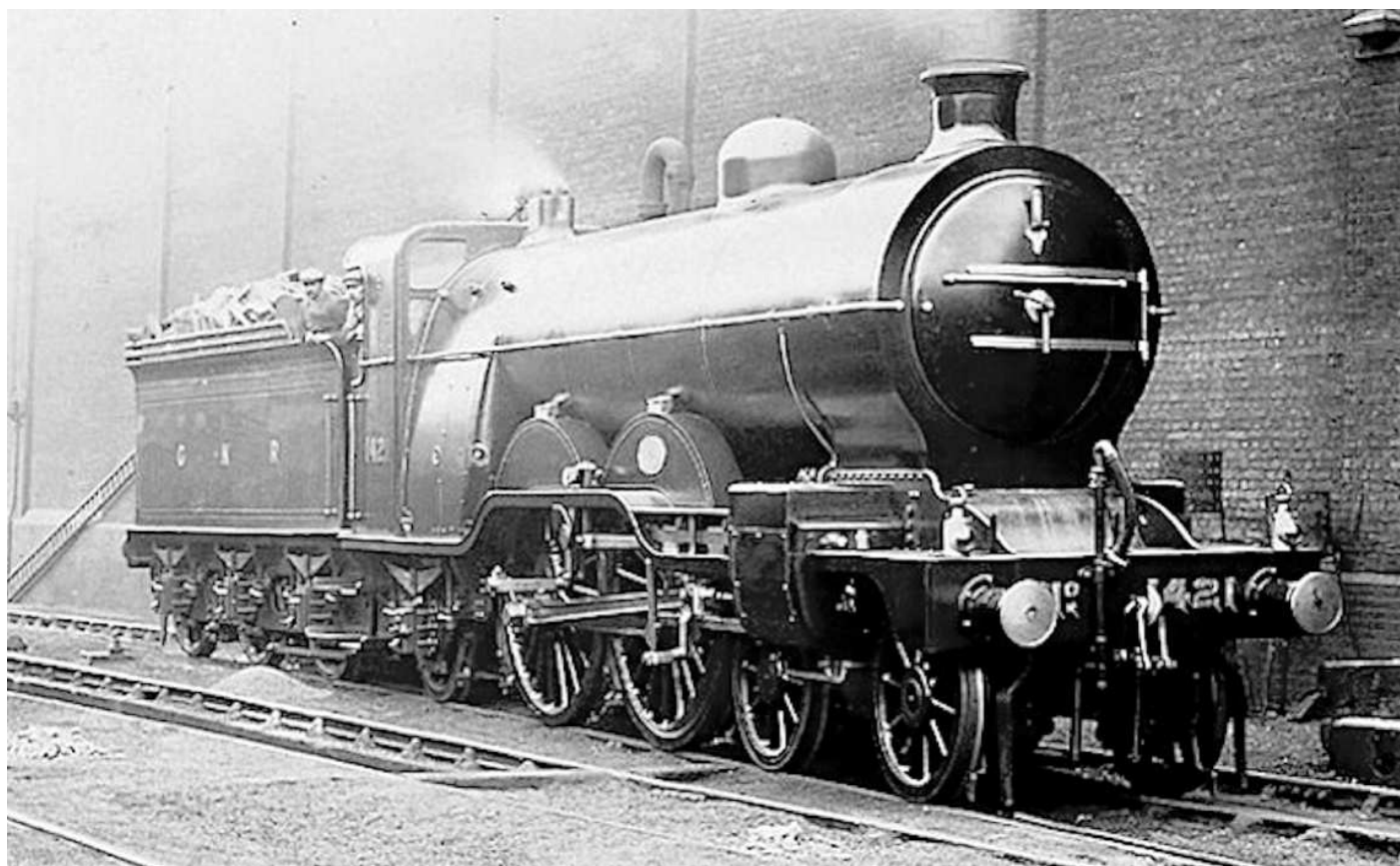
This GNR engine 1421 , works number 1166, was built in August 1907 at Doncaster Work. It was withdrawn from service forty years later in August 1947. 1421 was the last of Ivatt's C1 class compound engines and used Walschaerts valve gear. (Author's Collection)
