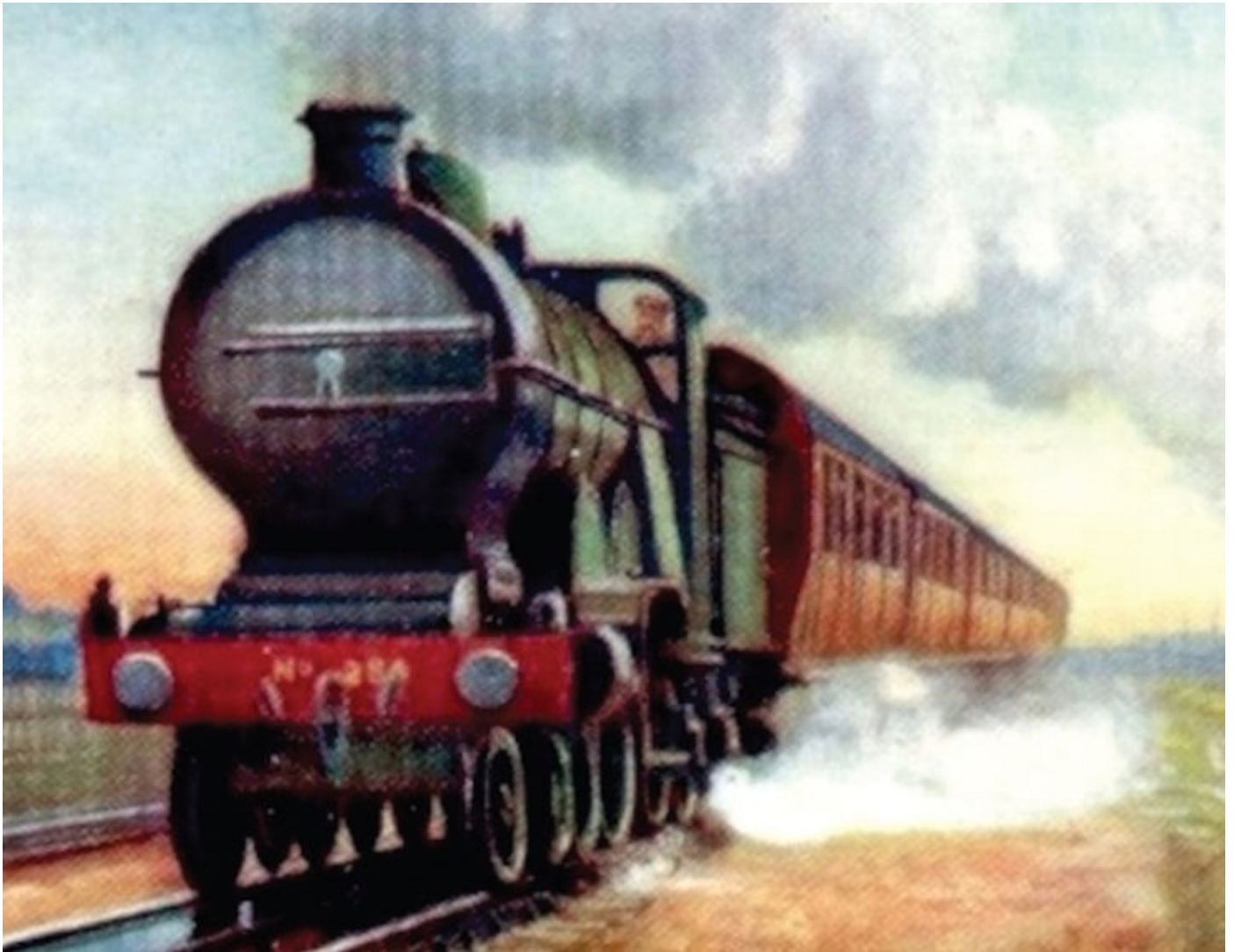
Large boiler Atlantic 284 had a tender, which had three coal rails instead of the usual two. It was common practice to interchange tenders and other engines acquired such tenders after the Grouping. This contemporary image of 284 does however show the tender as having two coal rails. (Author's Collection)
