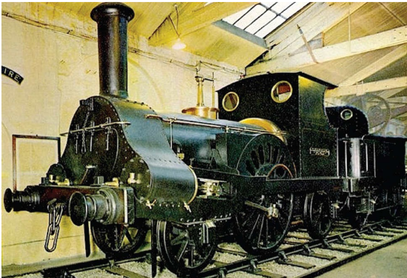
The Grand Junction Railway's 2-2-2 N° 49 Columbine was designed by Alexander Allen and was built at Crewe Works in 1845. It was withdrawn from service in 1902 and was set aside for preservation. In 1868, Ivatt, at the age of seventeen, was apprenticed at Crewe Works under John Ramsbottom. He would have learned his skills and trade working on engines such as this. (Author's Collection)
