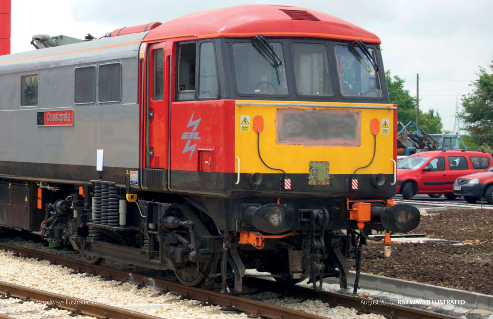
LEFT: The hole cut in the side of 86702 is clearly shown in this image; an access panel was attached later.
