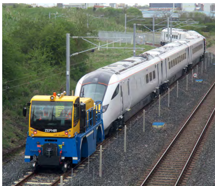
Type 20.300 road/rail loco Zephir 2631 moving unit 800004 on the Hitachi test track at Newton Aycliffe on May 13. (Alex Betteney)
