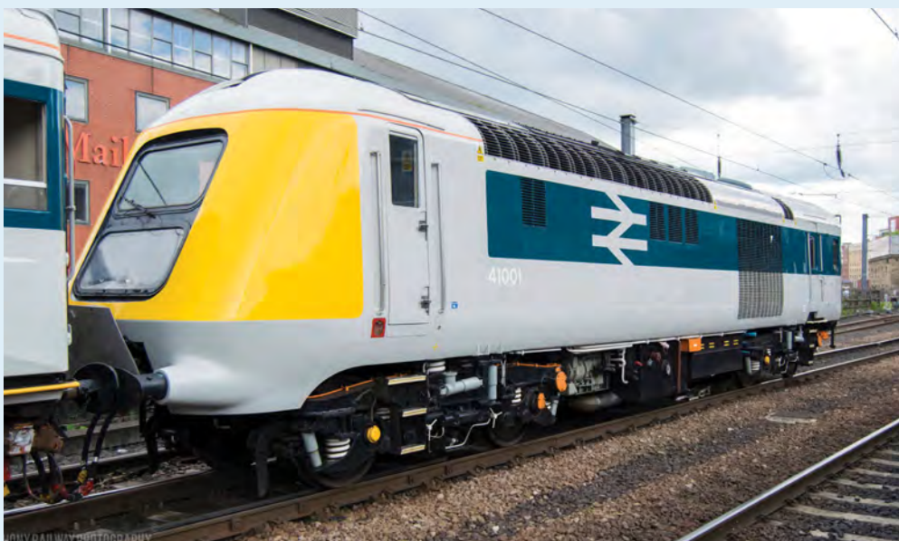
ABOVE: The flexibility that the nose-end buffers and coupling equipment offers is well illustrated in this view, as 41001 passes Newcastle on July 21 while en route to the Bo'ness & Kinneil Railway. (Anthony Whiteford)
