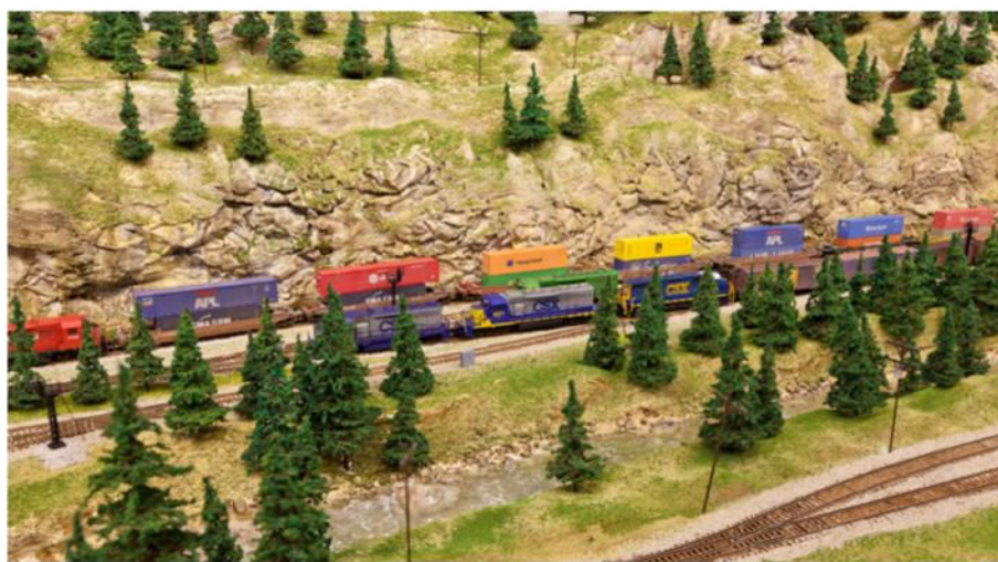
③ CSX SD40-2 no. 8071, in the center of the photo, is sound-equipped. Jean-Baptiste removed the motor and modified the chassis. The decoder is in the powered CSX Geep in front of 8071, and wires run to the speaker in the SD40-2.
