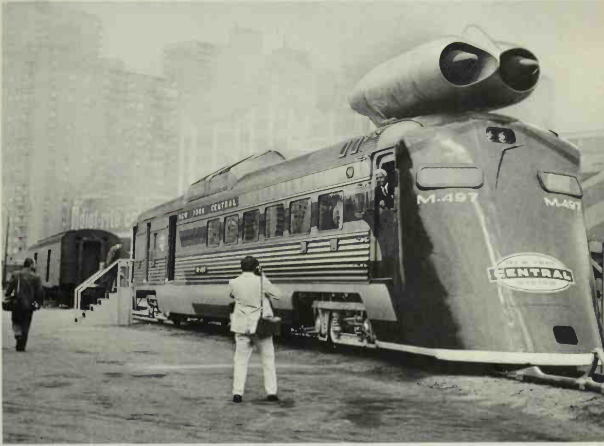
An American jet-powered train. During test runs, it set a record of 183.85 miles per hour. U.P.I.
