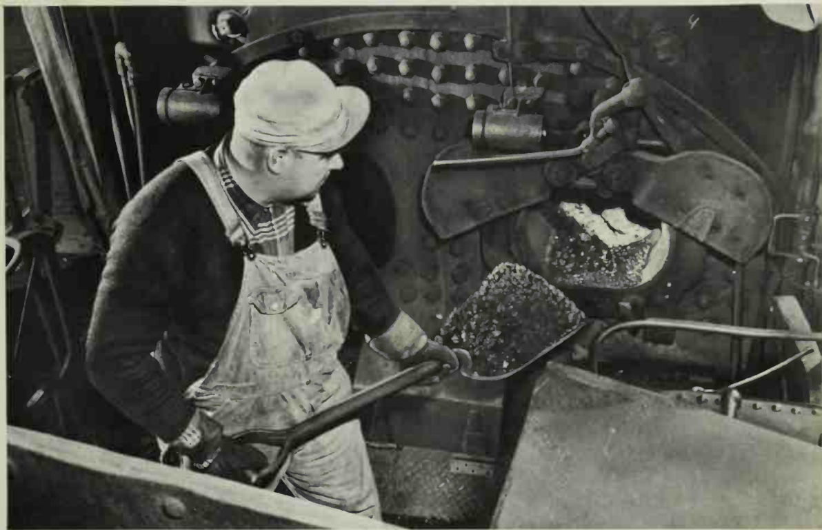
A fireman shoveling coal into the firebox. This firebox had butterfly doors that opened to either side.
