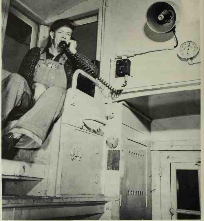
Inside the modern caboose, a conductor can talk by radiotelephone to the engineer at the head of the train. SANTA FE RAILWAY
