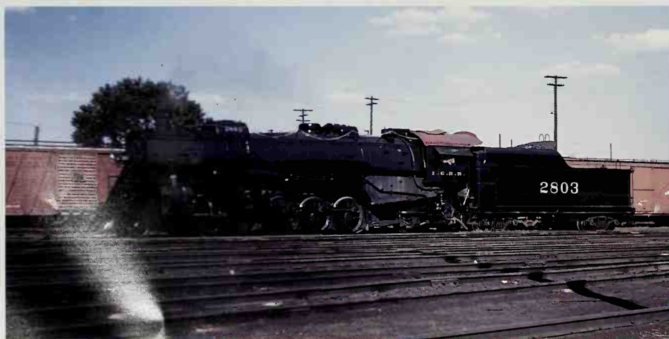
Recently outshopped, #2803 at Freeport, Illinois was built by Lima in 1921 and rebuilt with a new boiler by IC's Paducah Shops. She was used with other locomotives of her class on the Iowa Division's Dubuque District in meat train service. Owen Leander
