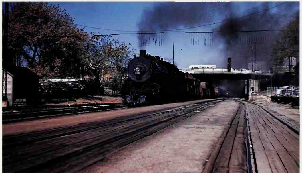
With a Kankakee city bus on the overpass, IC Mikado #2134, one of 28 similar 2-8-2s built by Lima with 64½" drivers, passes through Kankakee on Oct. 10, 1954. Note caboose directly behind locomotive. Jerry Carson
