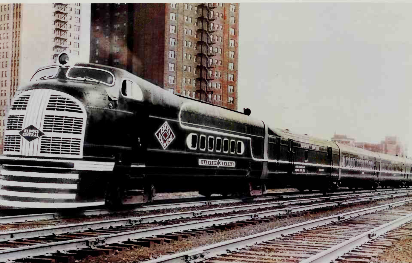
The streamlined Green Diamond was a sensation when it began service between Chicago and St. Louis in May of 1936; the green five-car train consisted of lightweight cars which were integral to one another. Glass plate courtesy Rich Gajnak
