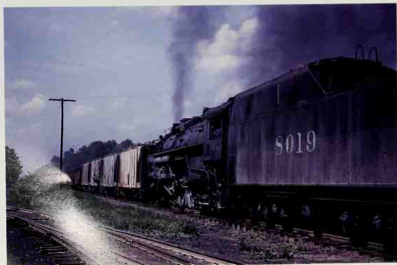
ABOVE. This Chicago exposition featured classic railroad equipment, including this IC 2-8-4 Mountain built by Lima in November of 1926. Large offset brass bell and old red and white IC logo on the overhead feedwater heater makes the locomotive distinctive. Rich Gajnak collection
