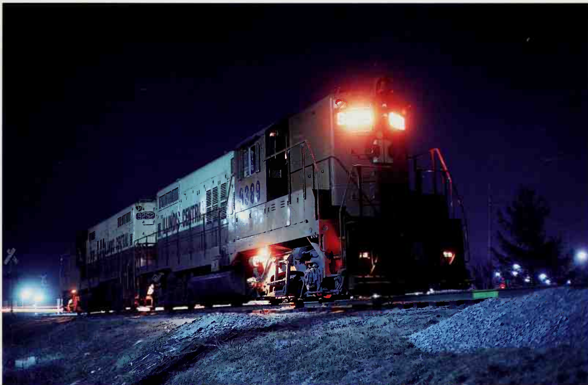
A pair of split-rail Geeps whine into the night as they perform switching duties for the Main Line of Mid-America. Unit #9389 is an EMD GP-9 with 1,750 hp and tractive effort of 44,600 lbs. Jerry Carson
