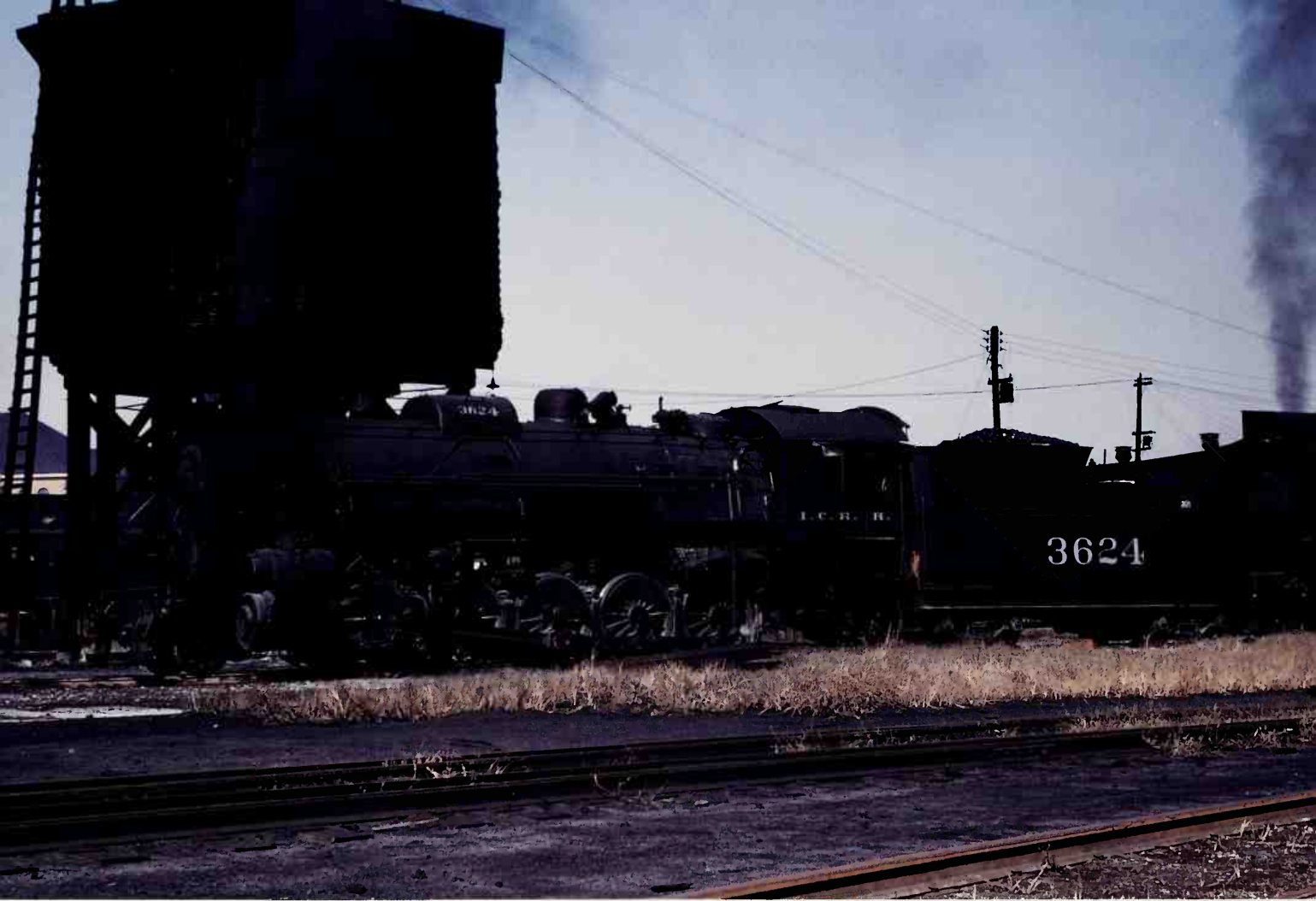
ABOVE. #3624 was built from a chassis and boiler from other locomotives; the clean locomotive sits next to one of IC's many black water tanks. Owen Leander
