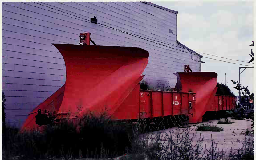
The IC favored gondolas converted to snowplows; here #X8034 and sister hides next to the roundhouse in 1981. Twenty years earlier the IC operated 26 of these. Jerry Carson
