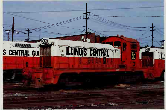
Illinois Central switcher #13 was a 600 hp SW-1 built in 1946. Jerry Carson
