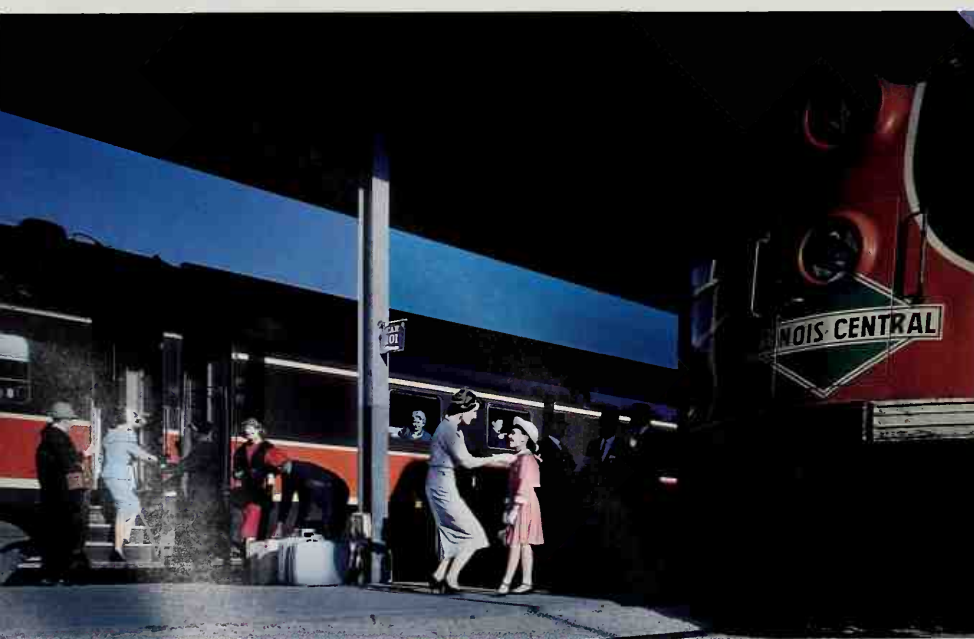
The streamlined Green Diamond was a sensation when it began service between Chicago and St. Louis in May of 1936; the green five-car train consisted of lightweight cars which were integral to one another. Glass plate courtesy Rich Gajnak
