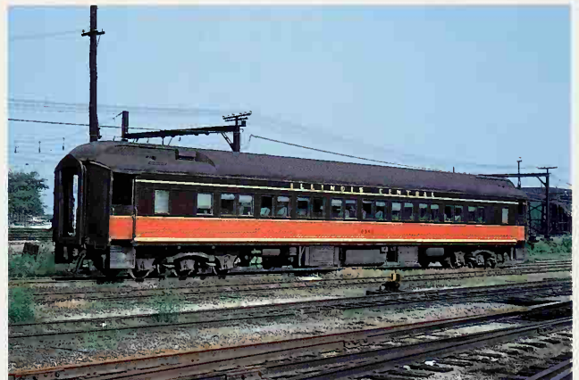
Long, sleek coach #2804 was 81 feet long; car had electro-mechanical air conditioning. Owen Leander
