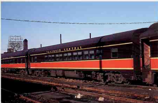
Coach #2685 sat 48 with its 79 foot length on six-wheel trucks. Owen Leander
