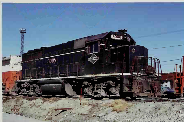
A 3,000-hp GP-40 #3008 built in 1966 offered lots of horsepower for IC freights. Jerry Carson
