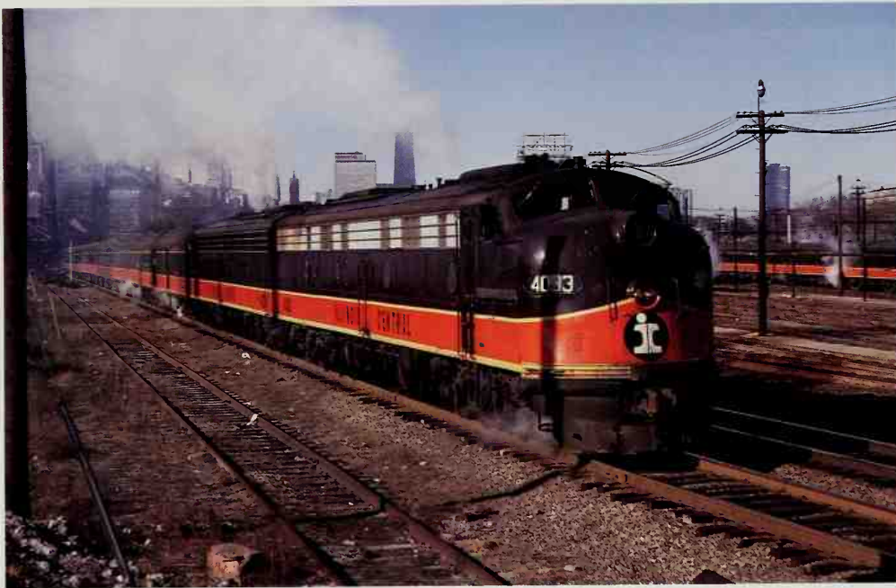
In March of 1969, IC #4033, an E-8 with 2,250 hp powered by four EMD D27 traction motors, leads a passenger run out of the yards south of Chicago's Central Station. Owen Leander
