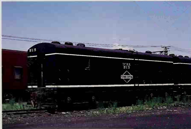
HU-5 heater car contained two Clarkson steam generators. Owen Leander
