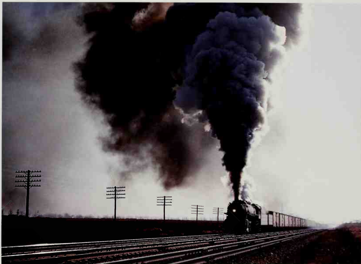
The IC was capable of putting on a spectacular smoke and steam show at any time on its lengthy route between the Great Lakes and the Gulf of Mexico. In November of 1955 near Bradley, Illinois, #2527, a former Central-type 2-10-2 converted to a 4-8-2, alternately darkens and whitens the prairie air. Jerry Carson
