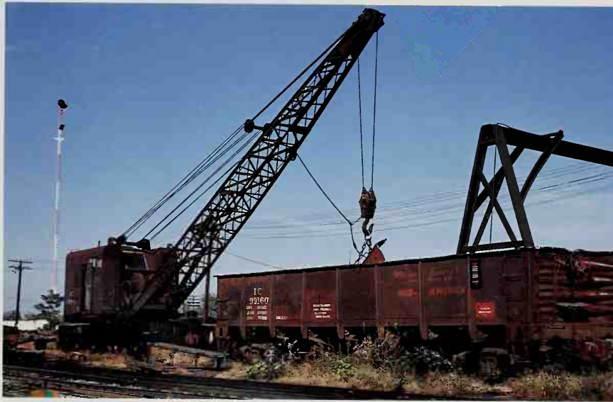
In 1963, the IC operated 41 different wrecking and locomotive cranes to service the property, from manufacturers such as Bucyrus, Orton, Shaw, Browning, Brownhoist and others. Jerry Carson
