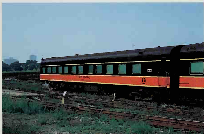
Split-rail design #3513 sleeper is the Centralia with 10 roomettes and six double bedrooms. Owen Leander
