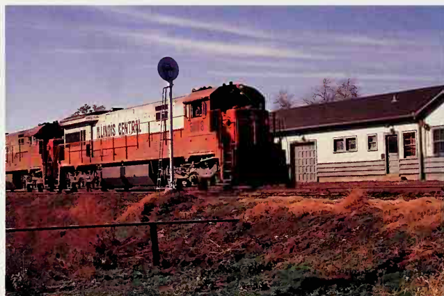
GE-built U33C, a 3,300 hp growler was one of 10 such IC diesels. Jerry Carson
