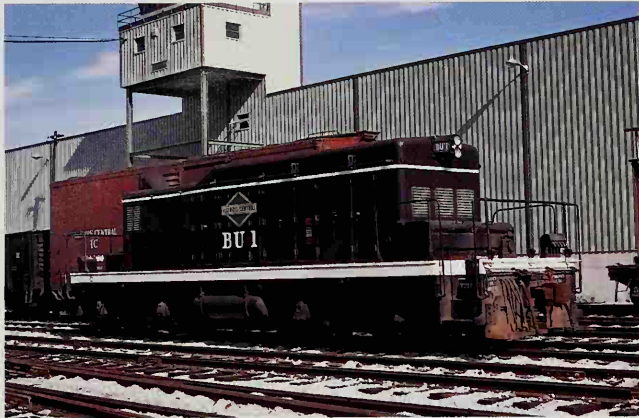
BU-1 was IC's slug converted in October of 1952 from SW1 #9017 at IC's own Paducah Shops. Owen Leander
