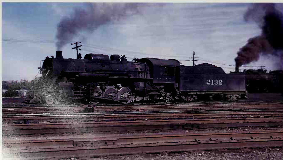
Of the same class as above, 2-8-2 #2132 had 30 x 32" cylinders and lasted until 1955. This old machine could tell a number of interesting stories if it could talk. Owen Leander
