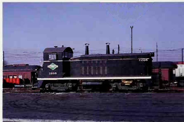
IC #1208 1,200 hp SW-7 built in 1950 shown at Cicero, Ill. Owen Leander
