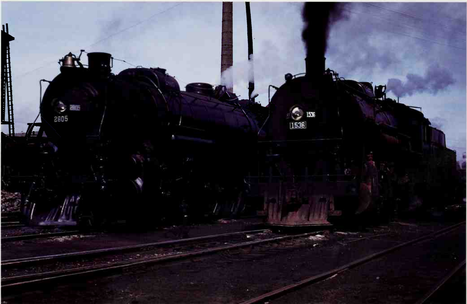
IC #1536, a 1914 Baldwin 2-8-2 with 63 \frac{1}{2} " drivers, and #2805, a bigger brother 2-10-2 from Lima in 1921 (renumbered in August, 1944 from #2942), wait on parallel ready tracks to lead their next trains. Owen Leander
