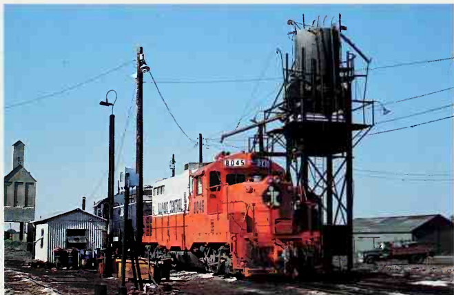
Originally built in 1954 as a GP-9, this unit was rebuilt to a GP-10. Jerry Carson
