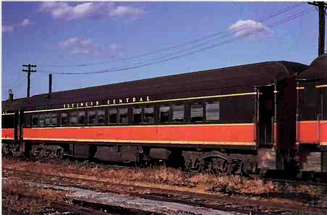
Heavyweight coach #2716 sat 64 passengers over its long six-axle trucks. Owen Leander
