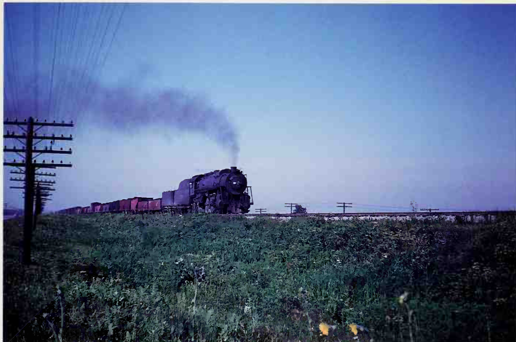
IC was known for its hotshot freight trains. Here #2611, a Paducah-built 4-8-2 with large 70" drivers, pulls a merchandise and coal train through Illinois prairie sometime in the 1950s; the engine was retired in 1960. Jerry Carson
