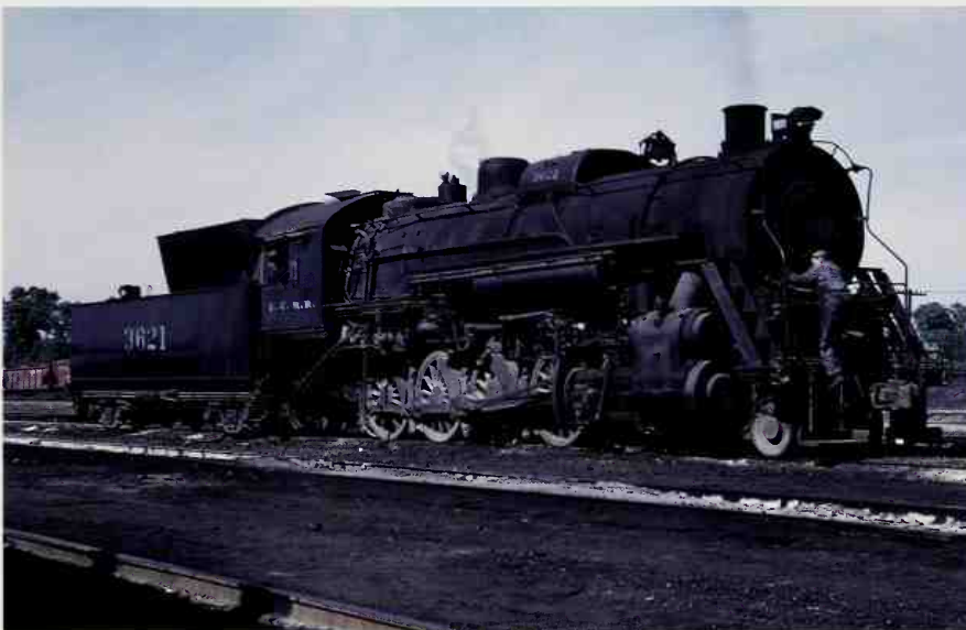
ABOVE. #3624 was built from a chassis and boiler from other locomotives; the clean locomotive sits next to one of IC's many black water tanks. Owen Leander
