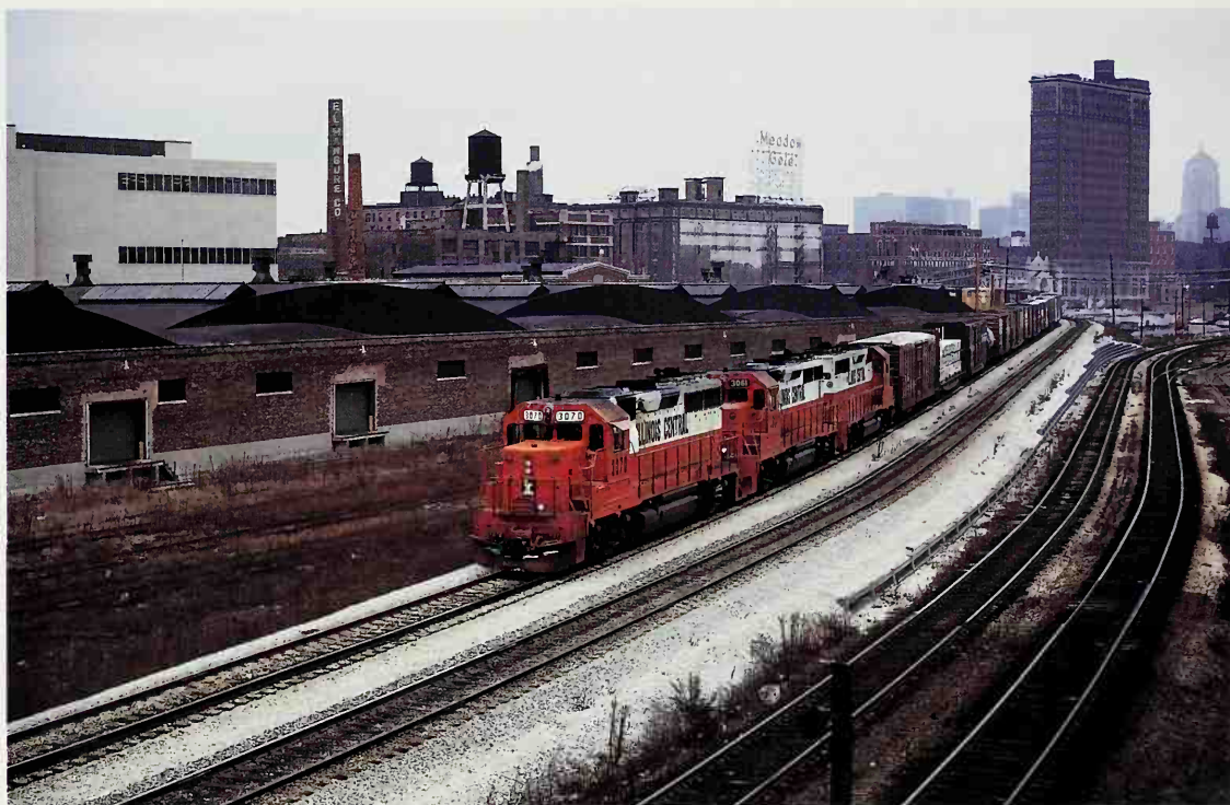
A pair of split-rail Geeps whine into the night as they perform switching duties for the Main Line of Mid-America. Unit #9389 is an EMD GP-9 with 1,750 hp and tractive effort of 44,600 lbs. Jerry Carson
