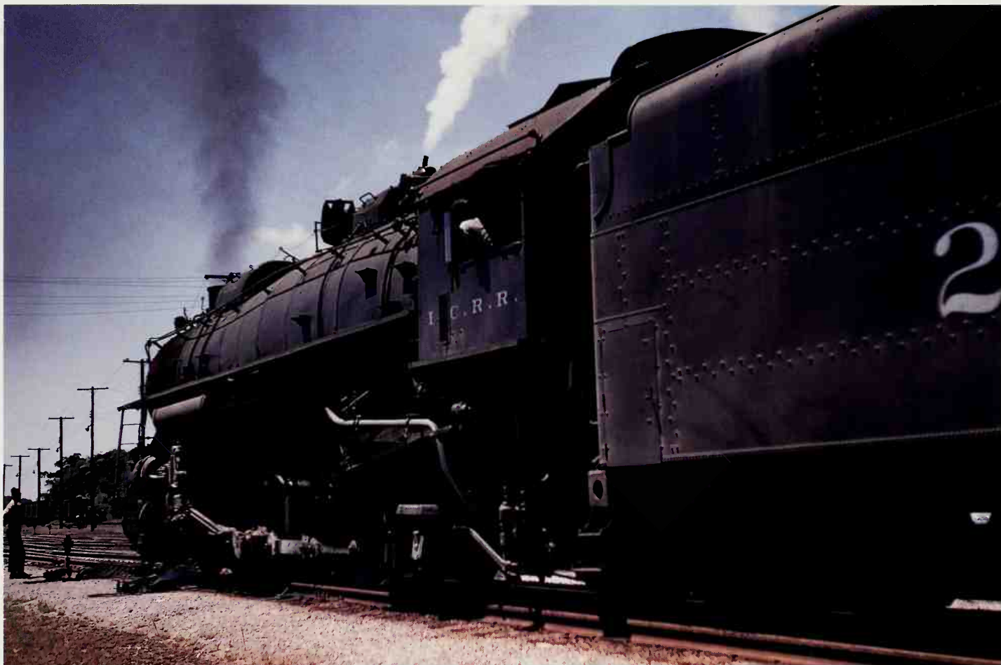
TOP. #2742 was one of a number of modernized 2-10-2s; it was built in 1923 and retired in December of 1959. The locomotive is shown at Paducah, Kentucky, to which track was laid around 1852 and at which a giant locomotive shop was constructed. Jerry Carson
