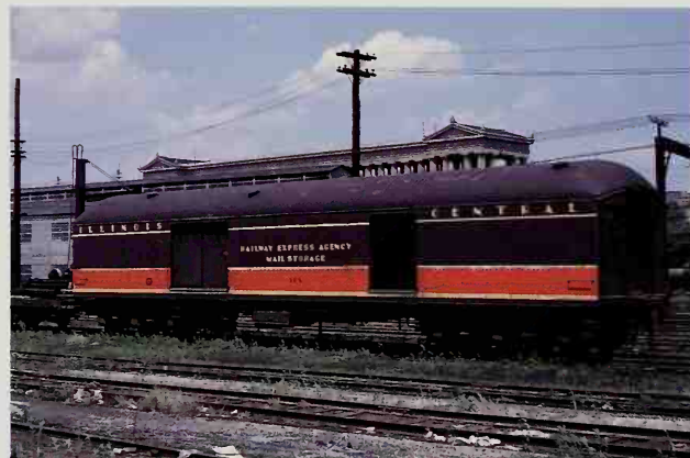
This is #568, a 64-foot-long storage and express car with an arched roof. Owen Leander
