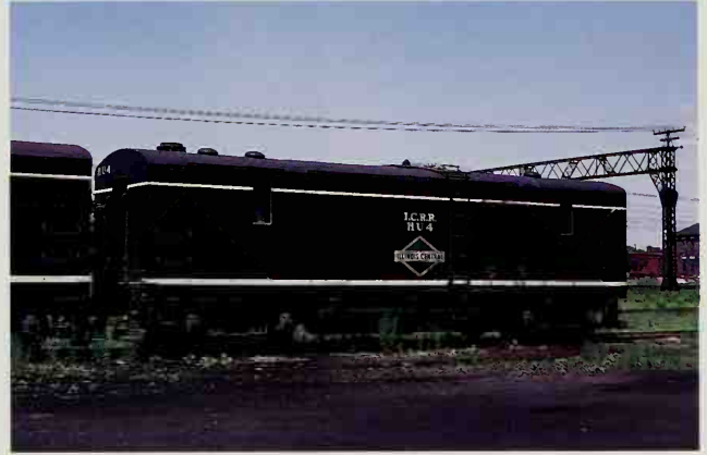
HU-4 was one of six heater cars built at Chicago's Burnside Shop on refrigerator car frames. Owen Leander
