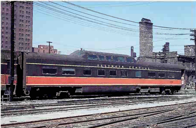
Pullman-Standard-built 1952 dome-coach #2211 seats 52 on lower level, 24 in dome. Owen Leander
