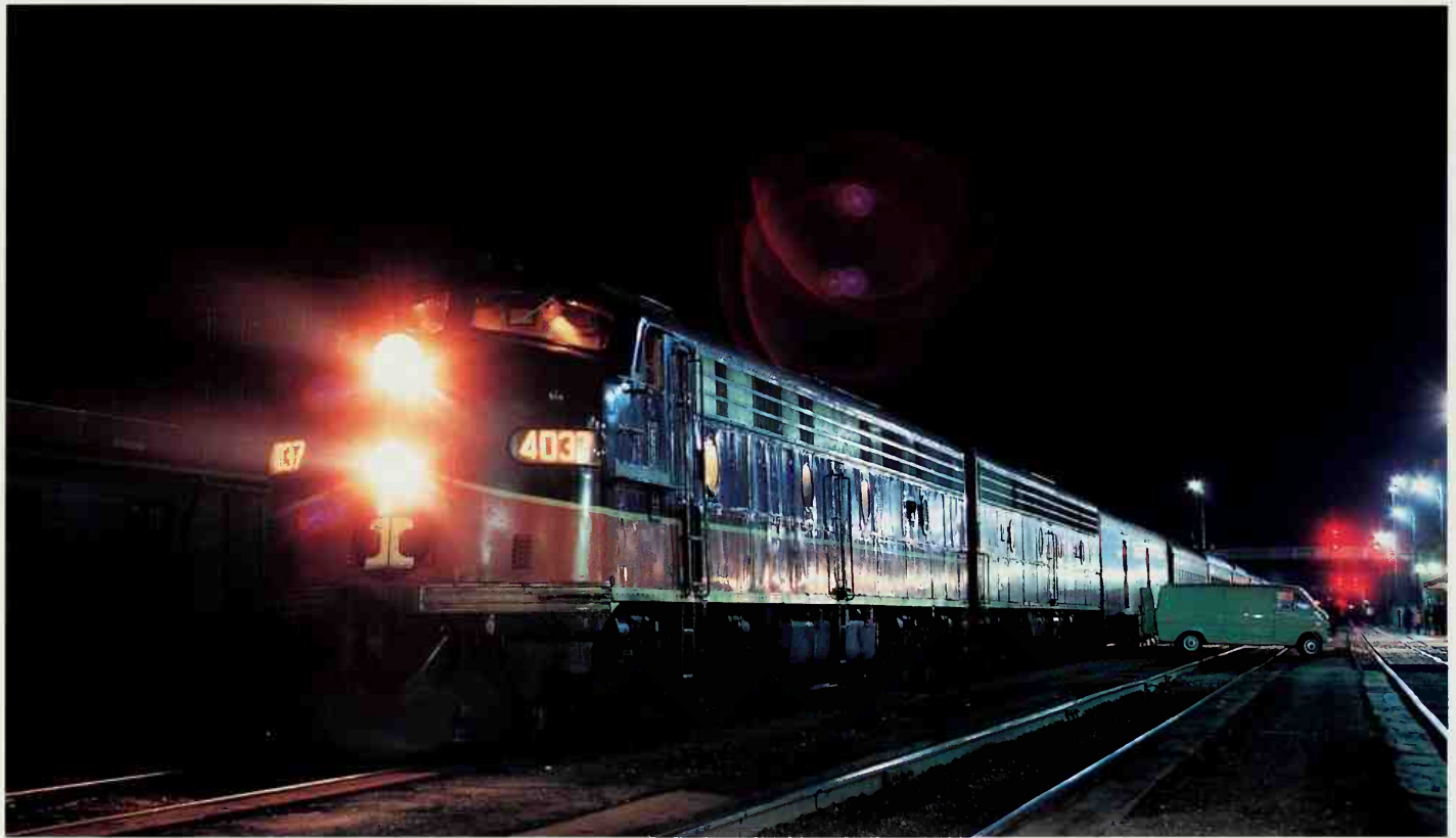
A 2,400-hp E-9 with four EMD type D37 traction motors with an IC split-rail on the nose gets ready to depart at Kankakee in spring of 1971. Kankakee, milepost 55.9 from Chicago, was a major station stop for passenger trains. A four-track, six-arch concrete bridge spanned the Kankakee River south of the IC station. Russ Porter
