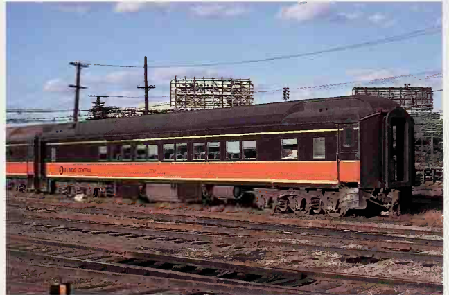
Coach-dormitory car #2732 had a dormitory capacity of 6, and 46 seat passenger capacity. Owen Leander
