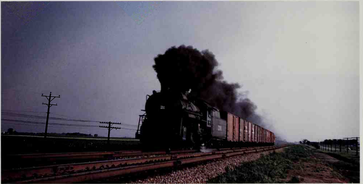
The IC reduced grades beginning in 1897 between Gilman and Springfield, Illinois from 58 feet to 26.4 feet per mile, thus increasing the tonnage ratings of locomotives by 88 percent. The #1391 is north of Gilman in the 1950s. Jerry Carson
