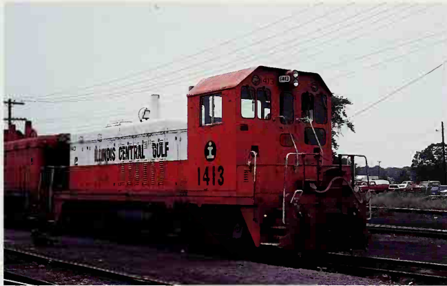
At Centralia, #1413 with squared off roof is a 1,300 hp EMD switcher; note lights over windows. Jerry Carson
