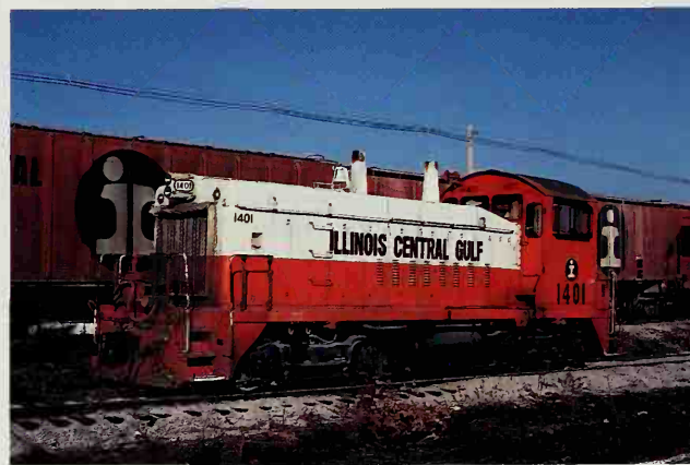
In Chicago, sharp looking #1401 was rebuilt in 1978 at Paducah to an SW-14. Jerry Carson
