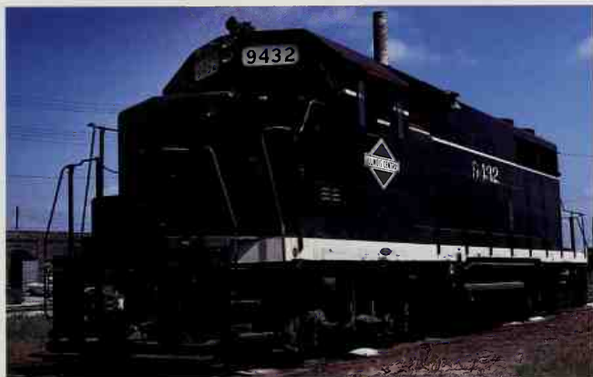
A GP-28 low-nose with 1,800 hp that was built in 1964. Jerry Carson
