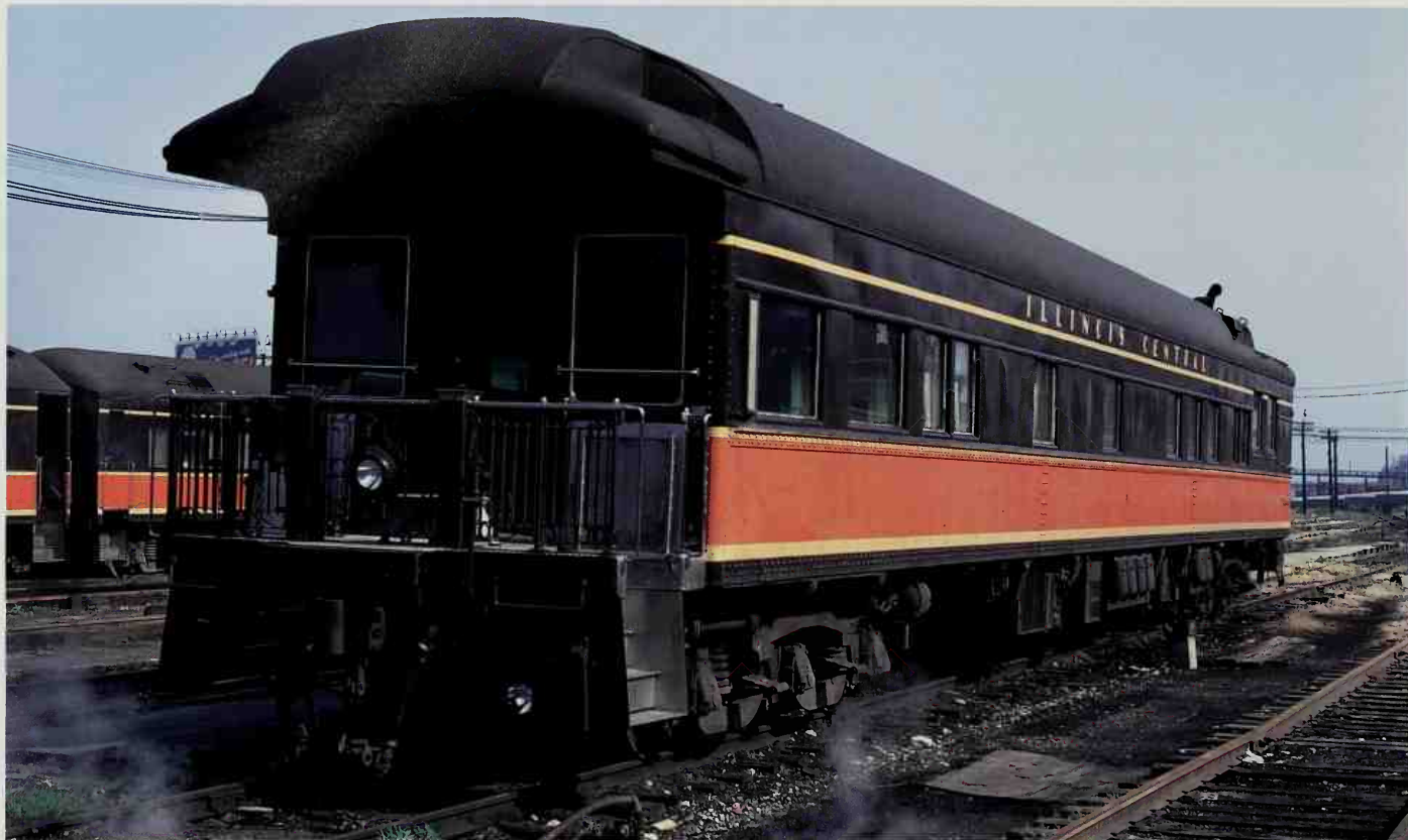
Office car #6 rests between trips in Chicago's passenger coach yard. The 83' 3" heavyweight observation was the heaviest office car on the IC in June of 1970 when this photo was taken. It contained a vapor hot water heater and Waukesha air conditioning. Owen Leander
