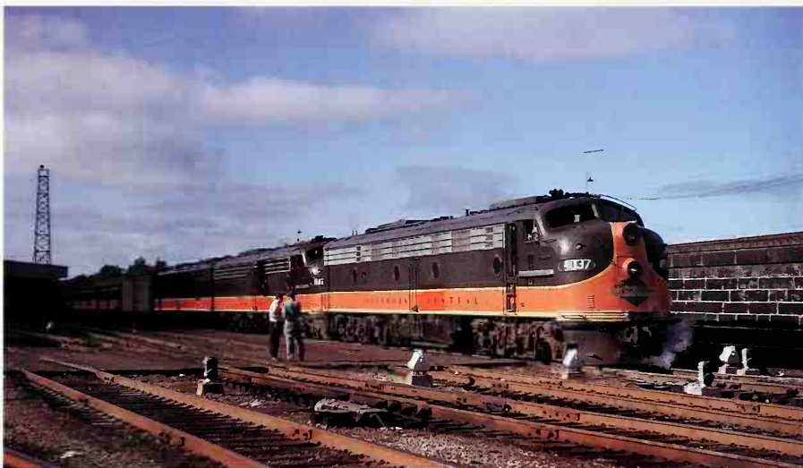
IC #4037, a 2,400 hp E-9A diesel leads off a three-unit set of power for an IC train awaiting departure time at Chicago Central Station in 1963. Owen Leander
