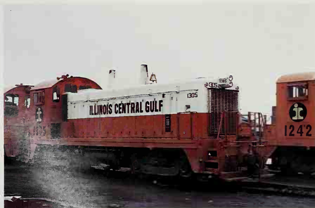
EMD SW-13 began as a 1,200 hp unit but was rebuilt to a 1,300 hp diesel. Jerry Carson
