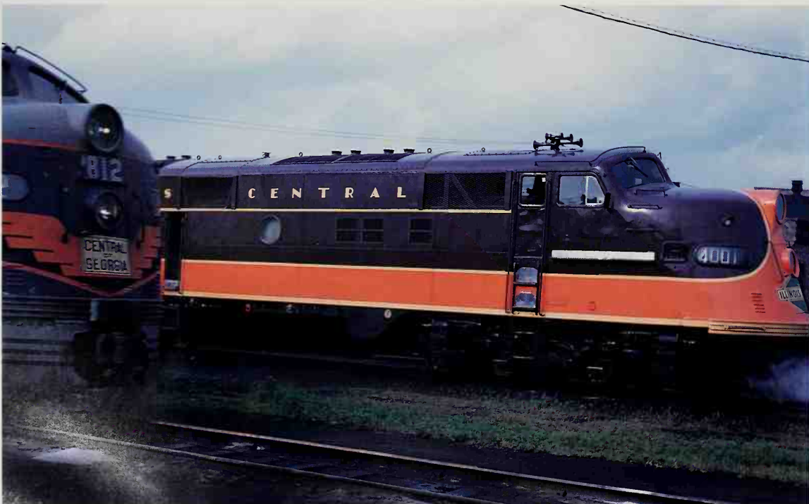
Diesel locomotive #4001, an E-6A built in 1941, and a Central of Georgia 2,250-hp EMD E-8A built in 1950, sit in Chicago in the fall of 1958. The IC and CofG pooled equipment for Florida-bound travelers. Jack Bailey, Don Heimburger collection
