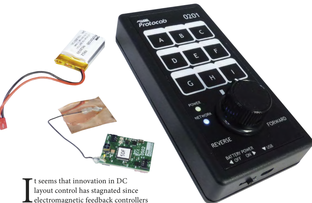
Protocab's Direct Controller (ref.0201) fits nicely in the hand with its throttle wheel positioned well for thumb use. Seen adjacent is its Locomotive Control Unit (ref.0502) with pressure sensitive copper switch and compact Lithium Ion Polymer Battery (ref.1902-902030).
