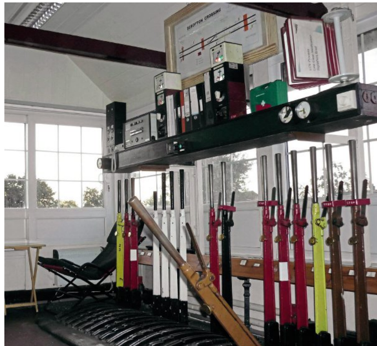
The lever frame and equipment inside the 'box'. Tim Helme
