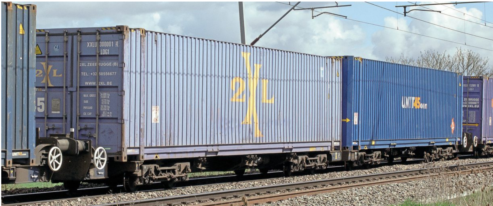
Carrying the 45ft high-cube containers for which it was built, No. 39 70 4901 036-6 passes Wilson's Crossing, Kingsthorpe, near Northampton, on April 16, 2016, bound for Purfleet. The immense 9ft 6in boxes are finished in 2XL and Unit45.com colours. Dan Adkins
