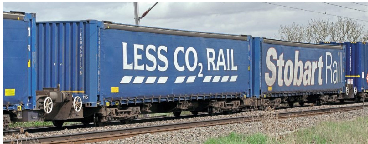
The IDAs are best known for carrying the distinctive Stobart Rail and Tesco 'Less CO2 Rail' 45ft swap body containers, these making use of the 'Super Lows' deck length rather than its low height. The more recent 9ft 6in 'Less CO2 Rail' high-cube container just visible on the wagon to the right, needs both features though. No. 39 70 4901 038-2 is seen at Kingsthorpe on May 3, 2016. Dan Adkins
