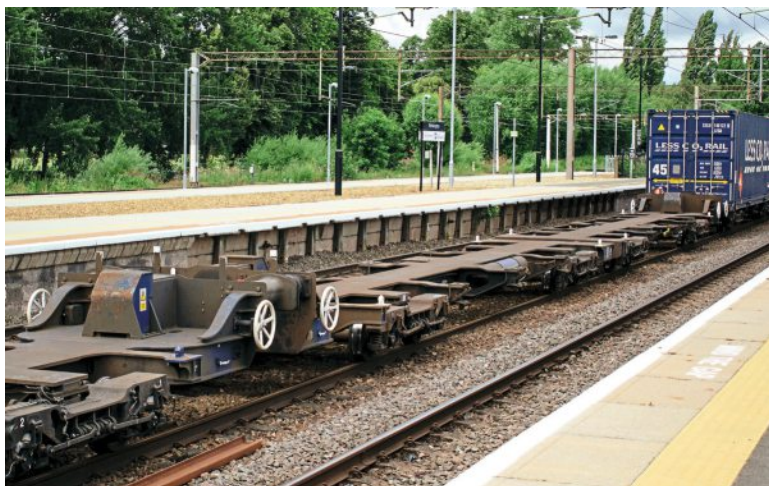
An empty production IDA, No. 39 70 4901 055-6, rumbles through Northampton on its way from Daventry to Purfleet on August 4, 2016. As is often the case for intermodal wagons, the 'Super Low' is filthy with cleaning limited to the handbrake areas and lettering. Of note is that it has white container spigots while those on its adjacent sister are blue. Dan Adkins
