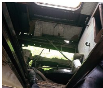
Above: The view through the toilet floor to the coach underframe and tracks. SDR
