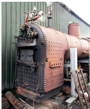
Isabel's valves lifting at 160psi during the boiler's steam test on July 11. EOR
