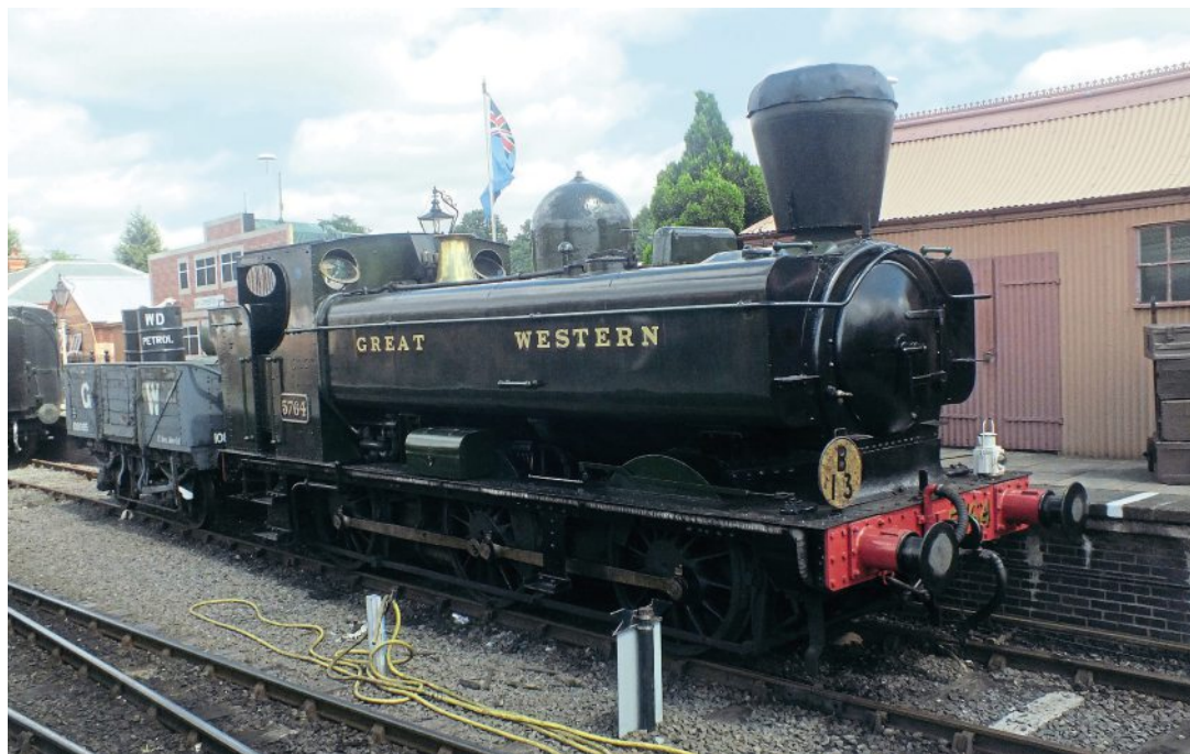
Out of ticket GWR Collett 0-6-0PT No. 5764, fitted with GWR-style spark arrestor for display in a mock military setting during the Step Back to the 40s weekend on July 1. Such spark arrestors were fitted to pannier tanks running on the nearby Cleobury Mortimer & Ditton Priors Light Railway, which served a military depot at Ditton Priors. PAUL APPLETON.
