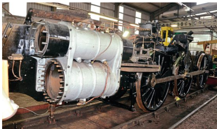
The rewheeled chassis of BR Standard 4MT 4-6-0 No. 75069 inside Bridgnorth Works in early July. It is hoped to have the locomotive complete this autumn so it can take some part in the SVR's busy pre-Christmas schedule. TONY BENDING
