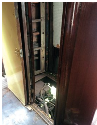
Above: The view through the toilet floor to the coach underframe and tracks. SDR
