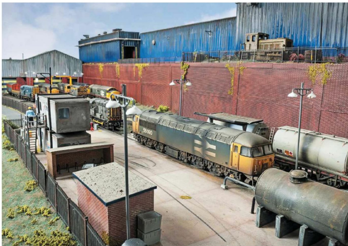
Above: Streaks of dirt on buildings are created by airbrushing a mix of black and RailMatch Roof Dirt (2403).
