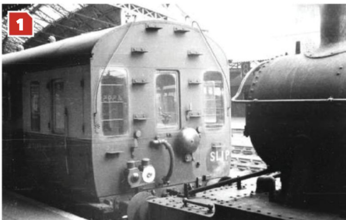
1: The rear of a slip coach for Reading being attached to a Paddington-bound train at Bristol Temple Meads in 1955. The centre window is a droplight, below which is the pedal-operated gong. The slip tail lamps, red beside white, indicate that this is the first (and in this case, only) slip. NEIL SPRINKS/CJL COLLECTION
