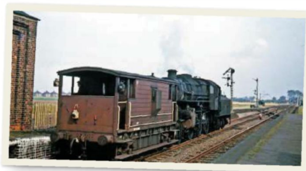
Ivatt 4MT No. 43068 arrives at Gedney with a brake van on September 3 1963. The signal behind has a tall, concrete post, with a somersault arm and a miniature wooden post, also with a somersault arm. The one behind that has a concrete post but has an LNER upper quadrant arm. ROB TIBBITS/COLOUR RAIL
